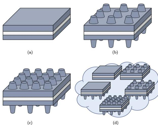
Fig. 1 Schematics of nanophotonic structures studied. Each structure is composed of silver (Ag, represented by white) and titanium dioxide (TiO<sub>2</sub>, shown in dark blue). (a) Three-layer structure. (b) Matched-period double-sided nanocone structure. (c) Unmatched-period double-sided nanocone structure. (d) Meta-structure.
