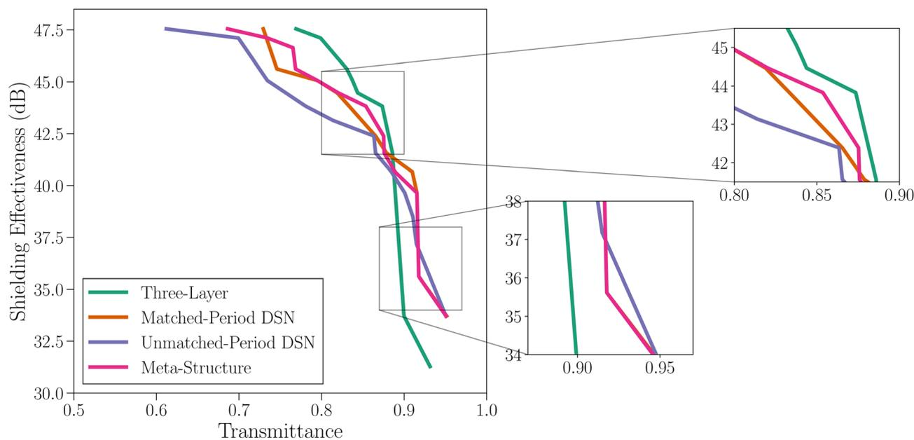
Fig. 5 Plot of the aggregated Pareto frontiers for the structures we study using Multi-BOWS, based on 10 repeated experiments. To alleviate the effects of the number of evaluations, we sample the first 100 evaluations from each simulation, except in the case of the unmatched-period double-sided nanocone structure. Those sampled evaluations of 10 repeated experiments are aggregated in order to show the best structures found. Note that DSN stands for double-sided nanocone.
