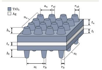
Fig. 2 Schematic of nanophotonic structures. The parameters used in this diagram apply across all structures studied. As an example, for a three-layer structure, the parameters for upper and lower cones are not used, while the other parameters remain applicable.
