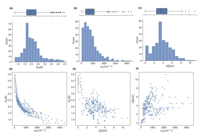
Fig. 1 The dataset of diatomic molecules' ground state spectroscopic constants. Panels (a–c) display the distribution of the main spectroscopic constants in the dataset- $R_{\rm e}$ ,  $\omega_{\rm e}$  and  $D_0^0$  – via a histogram representation and a box plot (at the top) for each. Panels (d–f) show the relationship between different spectroscopic constants of the molecules in the database.
