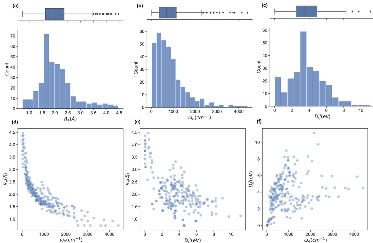
**Fig. 1** The dataset of diatomic molecules' ground state spectroscopic constants. Panels (a–c) display the distribution of the main spectroscopic constants in the dataset— $R_e$ ,  $\omega_e$  and  $D_0^0$ —via a histogram representation and a box plot (at the top) for each. Panels (d–f) show the relationship between different spectroscopic constants of the molecules in the database.
