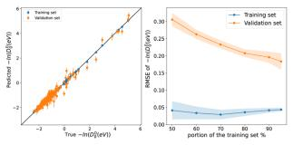
Fig. 5 Left panel, scatter plot of experimental values of  $-\ln(D_0^0)$  on the x-axis and predicted  $-\ln(D_0^0)$  on the y-axis via models d1, points, and error bars represent the predictive distribution means and standard deviations respectively after averaging over 1000 MC-CV steps. Right panel shows the learning curves of model d1. Points and shade around represent the  $\overline{RMSE}$  and  $\pm 0.5STD(\overline{RMSE})$  over 500 MC-CV splits.
