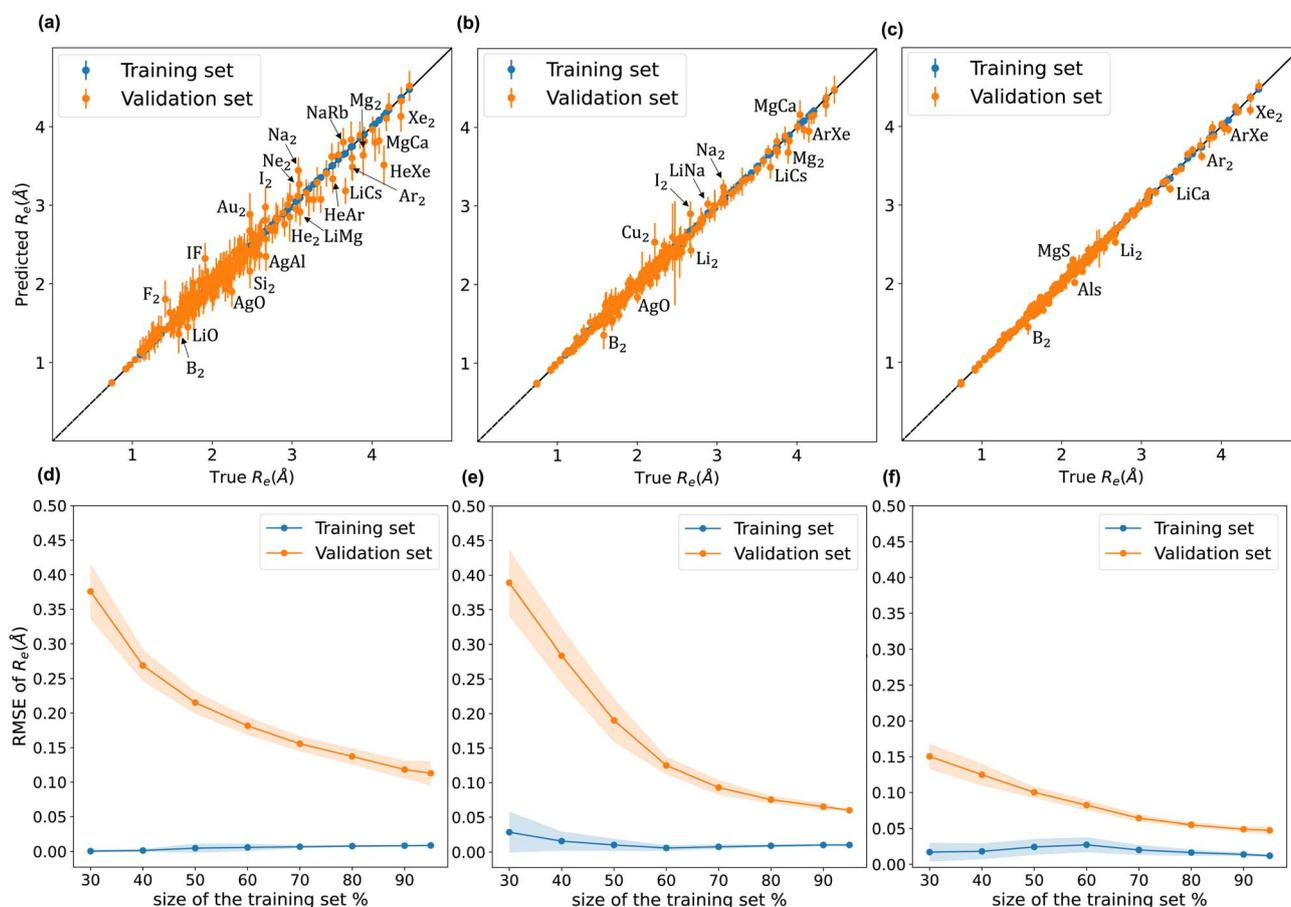
Fig. 3 Upper row shows scatter plots of experimental values of  $R_e$  on the x-axis and predicted  $R_e$  on the y-axis *via* models (a) r1 (b) r2 (c) r3, points, and error bars represent the predictive distribution means and standard deviations respectively after averaging over 1000 MC-CV steps. The lower row shows three learning curves of models (d) r1, (e) r2, and (f) r3. Points and shade around represent the RMSE and  $\pm 0.5\text{STD}(\text{RMSE})$  over 500 MC-CV splits.
