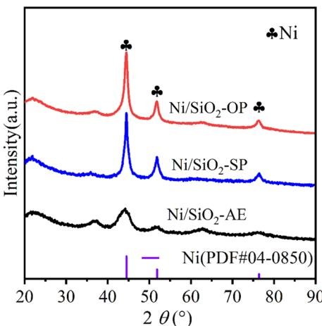
Fig. 3 XRD patterns of  $\text{Ni}/\text{SiO}_2$  catalysts.
