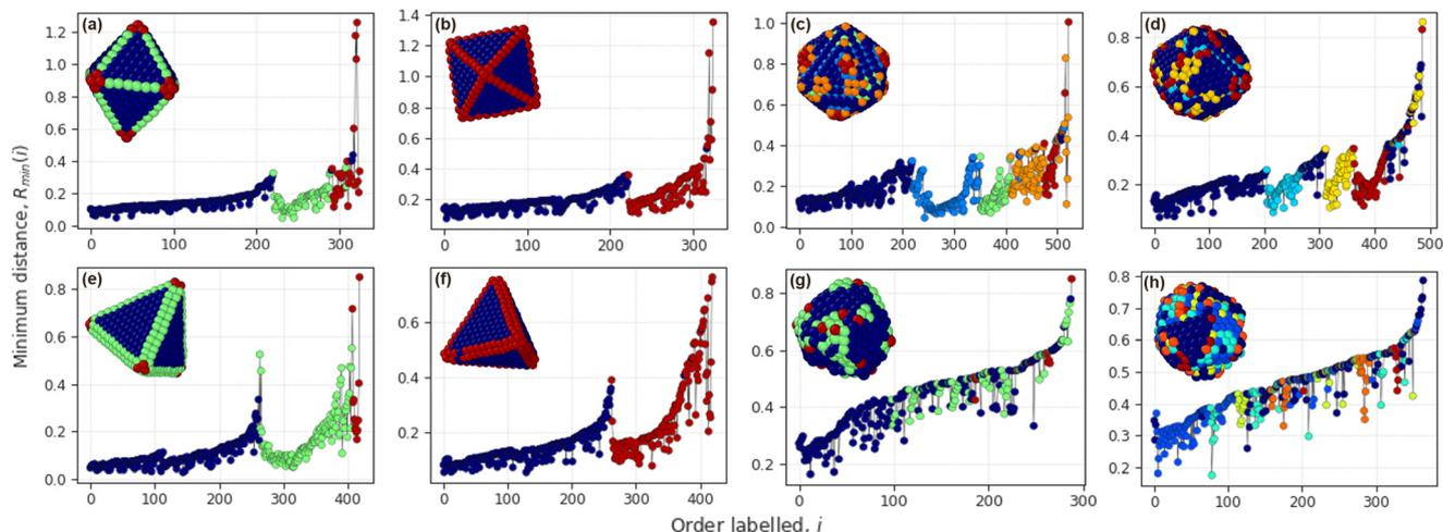
**Fig. 7** Iterative label spreading minimum distance plots for octahedron nanoparticles simulated at (a) 323 K and (b) 523 K, rhombic dodecahedron nanoparticles simulated at (c) 323 K and (d) 523 K, tetrahedron nanoparticles simulated at (e) 323 K and (f) 523 K, and (g) small- and (h) medium-sized disordered nanoparticles simulated at 723 K, coloured by clusters identified.
