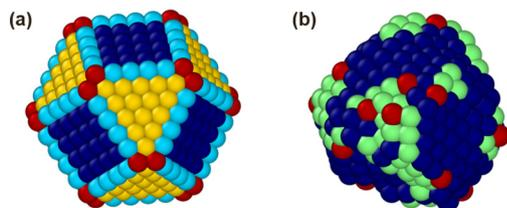
**Fig. 9** Identified surface clusters for the (a) ordered cuboctahedron nanoparticle simulated at 0 K and (b) smallest disordered nanoparticle simulated at 723 K. The cluster identifier number ascends from blue (smallest number) to red (biggest number). Clusters 1, 2, 3, and 4 of (a) thus correspond to the {100} facets, edges, {111} facets, and corners, respectively.
