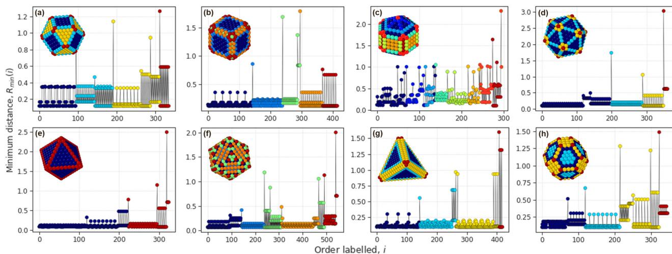
**Fig. 6** Iterative label spreading minimum distance plots for the (a) cuboctahedron, (b) cube, (c) decahedron, (d) icosahedron, (e) octahedron, (f) rhombic dodecahedron, (g) tetrahedron, and (h) truncated octahedron nanoparticles simulated at 0 K, coloured by clusters identified.
