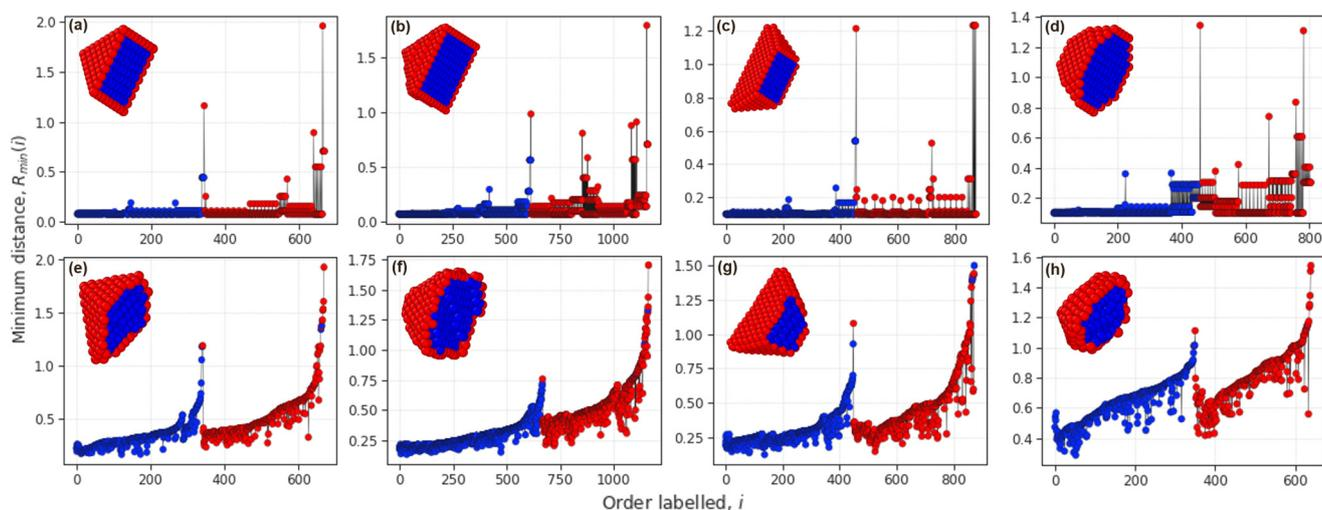
**Fig. 4** Minimum distance plots for the (a) octahedron, (b) rhombic dodecahedron, (c) tetrahedron, and (d) truncated octahedron nanoparticles simulated at 0 K, the (e) octahedron, (f) rhombic dodecahedron, and (g) tetrahedron nanoparticles simulated at 523 K, and (h) the smallest disordered nanoparticles simulated at 723 K. The nanoparticles are sliced across the *x*-axis or (100) plane. The points are coloured by whether they are surface (red) or bulk (blue) atoms.
