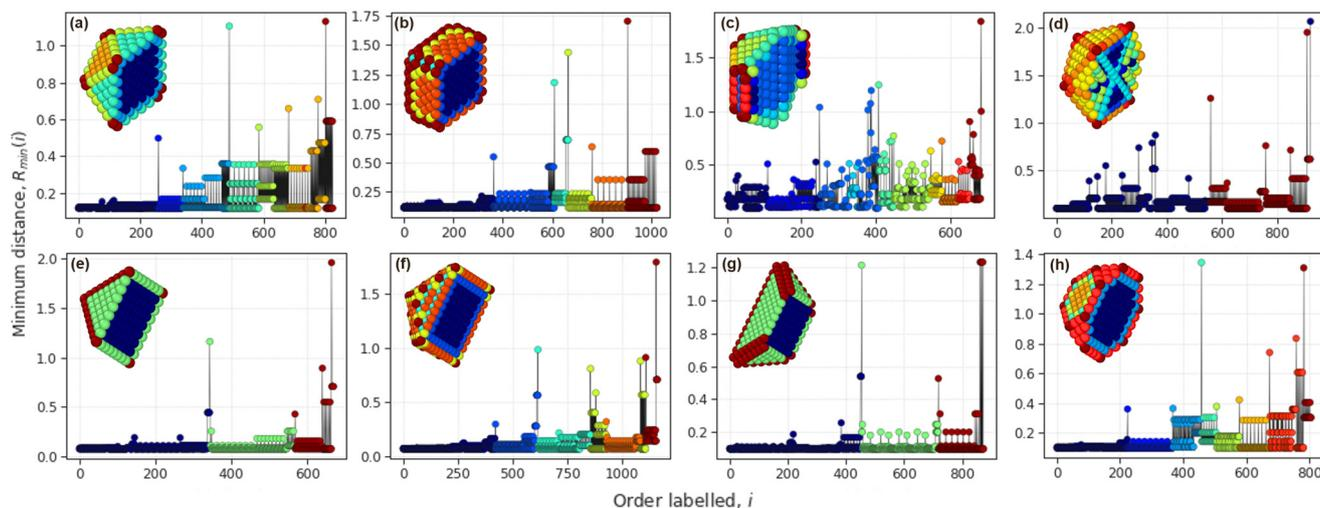
**Fig. 5** Minimum distance plots for the (a) cuboctahedron, (b) cube, (c) decahedron, (d) icosahedron, (e) octahedron, (f) rhombic dodecahedron, (g) tetrahedron, and (h) truncated octahedron nanoparticles simulated at 0 K, coloured by clusters identified. The nanoparticles are sliced across the  $x$ -axis or (100) plane.
