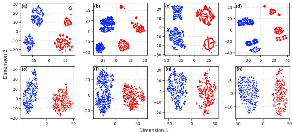
**Fig. 3** Mapping of the high dimensional data sets for the (a) octahedron, (b) rhombic dodecahedron, (c) tetrahedron, and (d) truncated octahedron nanoparticles simulated at 0 K, the (e) octahedron, (f) rhombic dodecahedron, and (g) tetrahedron nanoparticles simulated at 523 K, and (h) the smallest disordered nanoparticle simulated at 723 K, onto 2D manifold learnt *via* *t*-distributed stochastic neighbour embedding. The red and blue points correspond to surface and bulk atoms, respectively.
