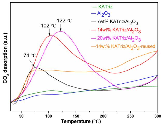
Fig. 6 CO<sub>2</sub>-TPD profiles of KATriz, Al<sub>2</sub>O<sub>3</sub>, and KATriz/Al<sub>2</sub>O<sub>3</sub> catalysts.
