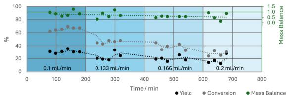
Fig. 9 Time profile of the effect of flow rate on yield, conversion and mass balance (mass entering the reactor/mass leaving the reactor) for Hf(OTf)<sub>4</sub>. Two-points moving average trendlines used for yield (black) and conversion (grey) to highlight the trends. Linear trend line used for mass balance (green).
