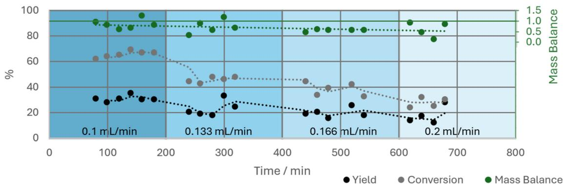
Fig. 9 Time profile of the effect of flow rate on yield, conversion and mass balance (mass entering the reactor/mass leaving the reactor) for Hf(OTf)<sub>4</sub>. Two-points moving average trendlines used for yield (black) and conversion (grey) to highlight the trends. Linear trend line used for mass balance (green).
