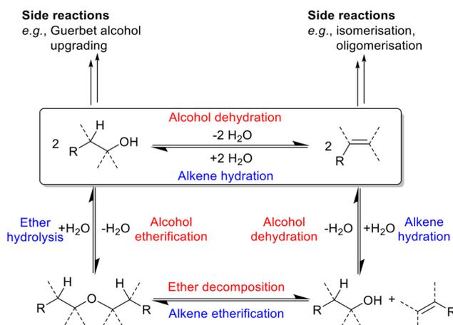
Scheme 1 Alcohol dehydration and competing side reactions.<sup>8</sup>
