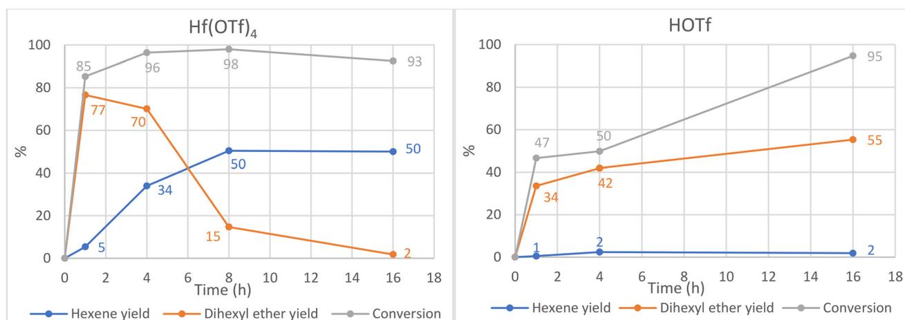
**Fig. 2** Dehydration of 1-hexanol to dihexyl ether and subsequent conversion to hexenes over time in a batch reactor using Hf(OTf)<sub>4</sub> (left) and HOTf (right). Reaction conditions (left): Hf(OTf)<sub>4</sub> (0.5 mol%), 500 r min<sup>-1</sup>, 180 °C, 1-hexanol (5 mL). Reaction conditions (right): HOTf (0.5 mol%), 500 r min<sup>-1</sup>, 180 °C, 1-hexanol (5 mL).
