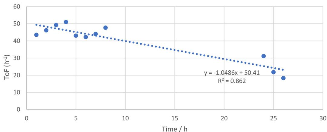
Fig. 8 Catalyst lifetime tests: Hf(OTf)<sub>4</sub> (0.7 mmol), 180 °C reaction temperature, 5 mL paraffin oil, 0.1 mL min<sup>-1</sup> 2-Me-butan-1-ol, 100 min<sup>-1</sup> N<sub>2</sub>, outlet temperature 160 °C.
