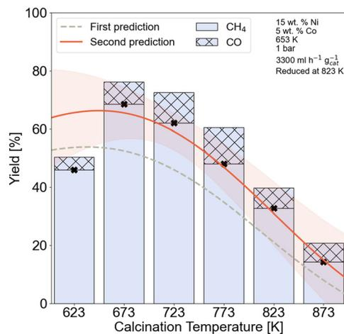
**Fig. 7** Effect of calcination temperature on the CH<sub>4</sub> yield. Experimental conditions are given in the right inset. Dashed lines represent the first prediction of yield by the model, and red lines represent the second prediction. The orange band indicates the model uncertainty.
