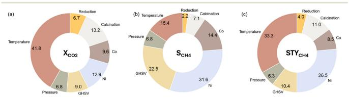
Fig. 6 Relative importance based on Shapley Additive Explanations (SHAP) values of the considered experimental variables for (a)  $X_{CO_2}$ , (b)  $S_{CH_4}$ and (c) STY<sub>CH<sub>4</sub></sub>
