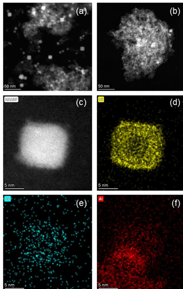
Fig. 9 HAADF-STEM images of (a) reduced 15Ni-5Co/Al<sub>2</sub>O<sub>3</sub>-673 and (b) reduced 15Ni-5Co/Al<sub>2</sub>O<sub>3</sub>-823. (c) Magnified HAADF-STEM image of reduced 15Ni-5Co/Al<sub>2</sub>O<sub>3</sub>-673. Elemental mapping of reduced 15Ni-5Co/Al<sub>2</sub>O<sub>3</sub>-673 for (d) Ni, (e) Co, (f) Al.
