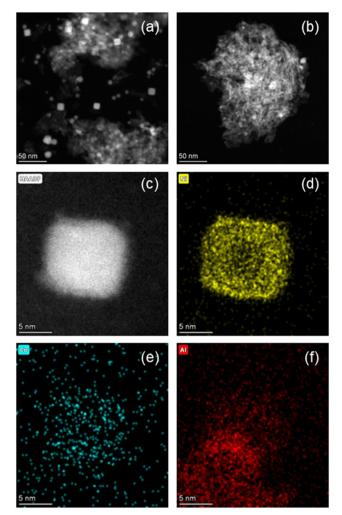
Fig. 9 HAADF-STEM images of (a) reduced 15Ni-5Co/Al<sub>2</sub>O<sub>3</sub>-673 and (b) reduced  $15Ni-5Co/Al_2O_3-823$ . (c) Magnified HAADF-STEM image of reduced 15Ni-5Co/Al<sub>2</sub>O<sub>3</sub>-673. Elemental mapping of reduced 15Ni-5Co/Al<sub>2</sub>O<sub>3</sub>-673 for (d) Ni, (e) Co, (f) Al.
