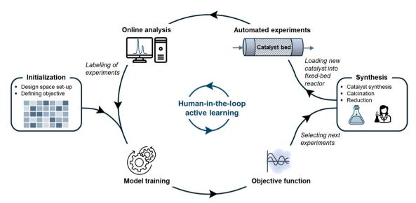
Fig. 1 General workflow for human-in-the-loop active learning of a catalytic reaction.
