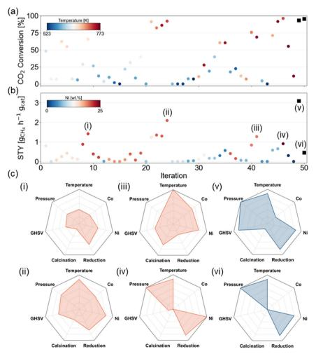
Fig. 5 Overview of the (a)  $X_{CO_2}$  and (b)  $STY_{CH_4}$  for all experiments in the training set and the two selected optimal points (black squares). (c) Radar plots show the experimental details for 4 selected training samples (red, i-iv) and the two optimized experiments (blue, v-vi).
