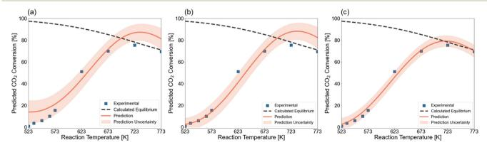
Fig. 10 Light-off curve prediction for a  $19Ni-4Co/Al_2O_3$  catalyst, calcinated at 723 K, reduced at 873 K. The test is performed at 1 bar and 3300 ml  $h^{-1}$   $g_{cat}^{-1}$  GHSV. (a) Prior prediction without knowledge about the catalytic system. (b) Predicted curve after performing one experiment with the  $19Ni-4Co/Al_2O_3$  catalyst at the zone of highest uncertainty. (c) Posterior prediction in which the Gaussian processes model the performed activity
