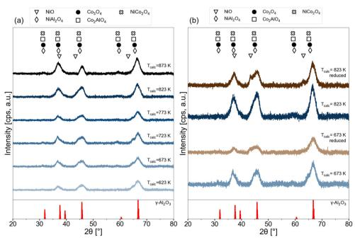
Fig. 8 XRD patterns of 15Ni-5Co/Al<sub>2</sub>O<sub>3</sub> samples (a) at various calcination temperatures (b) freshly calcined at 673 K and 823 K and reduced versions of these freshly calcined catalysts at 823 K.
