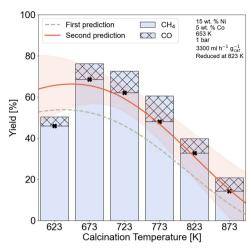
Fig. 7 Effect of calcination temperature on the CH<sub>4</sub> yield. Experimental conditions are given in the right inset. Dashed lines represent the first prediction of yield by the model, and red lines represent the second prediction. The orange band indicates the model uncertainty
