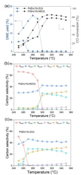
Fig. 7 Catalytic performance of the mpHZSM-5(25) and HZSM-5(25)based catalysts PdZn(15)-MZ(3) and PdZn(15)-Z(3): (a) DME yields and (b and c) carbon selectivities.
