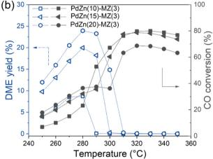
Fig. 8 Influence of (a) the Zn/Pd molar ratio and (b) the Pd loading for mpHZSM-5(25)-based catalysts.
