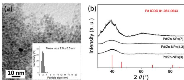
Fig. 1 (a) TEM image with size histogram of Pd/Zn-NPs(3). (b) XRD patterns of Pd/Zn-NPs with a Zn/Pd molar ratio of 3, 4.3 and 7.
