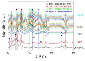
Fig. 5 Evolution of the XRD patterns of PdZn(15)–MZ(3) during activation of the calcined catalyst in H $_2$  atmosphere (2 vol% in N $_2$ ) in the temperature range of 40 °C to 350 °C.
