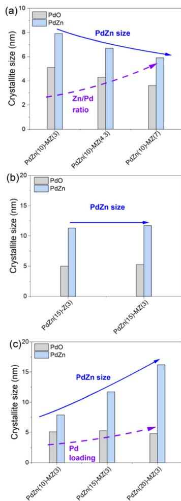
**Fig. 4** Crystallite sizes of PdO and intermetallic PdZn particles in the calcined and spent bifunctional PdZn/ZnO/zeolite catalysts: Influence of the (a) Zn/Pd molar ratio, (b) structure of zeolite dehydration catalyst and (c) Pd loading (crystallite sizes were calculated using the Scherrer equation of the (110) and (111) reflection at  $41.9^\circ$  ( $2\theta$ ) and  $41.2^\circ$  ( $2\theta$ ), respectively).
