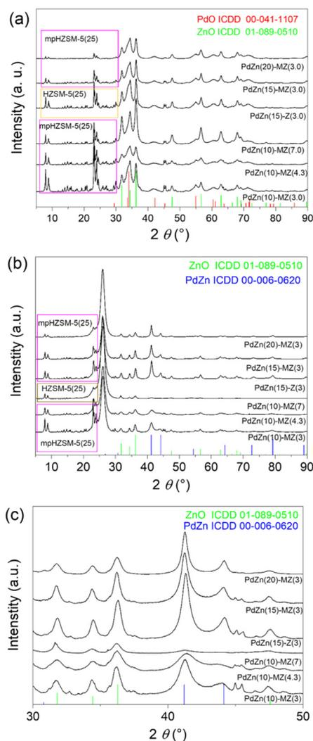
**Fig. 3** The XRD patterns of the (a) calcined and (b) spent Pd/Zn-based catalysts after catalytic tests with (c) enlarged area of characteristic PdZn reflections of the intermetallic PdZn particles (the reflection at about 26° (2 $\theta$ ) for the spent catalysts is due to the foil (Mylar foil) used to cover the sample for XRD measurements under Ar, see Fig. S4(b)†).
