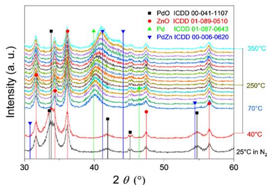
**Fig. 5** Evolution of the XRD patterns of PdZn(15)-MZ(3) during activation of the calcined catalyst in  $H_2$  atmosphere (2 vol% in  $N_2$ ) in the temperature range of  $40^\circ\text{C}$  to  $350^\circ\text{C}$ .
