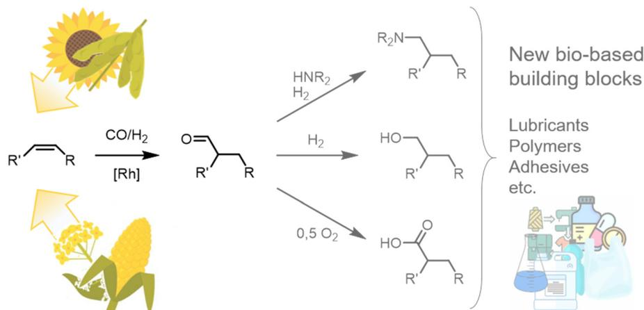
**Fig. 1** Hydroformylation on the internal alkene of a plant oil-derived oleochemical yielding an aldehyde as a bio-based platform chemical with a wide range of possible applications.
