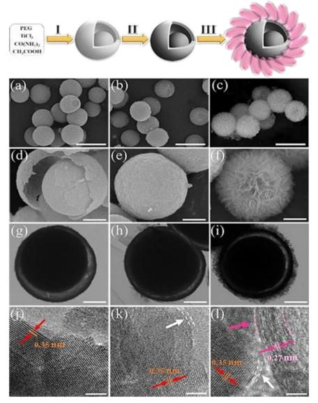
Fig. 3 Overall flowchart for the fabrication of the 3D Y@S TiO2-x/LDH architecture (steps I-III); corresponding (a-f) FESEM, (g-i) TEM, and (j-l) HRTEM images of the 3D Y@S TiO<sub>2-x</sub>/LDH sites. 13
