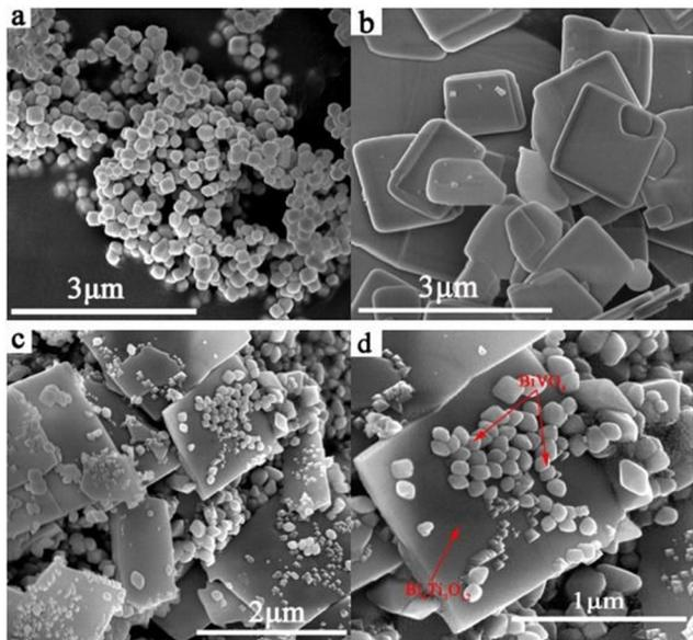
Fig. 8 SEM images of (a)  $\text{BiVO}_4$ , (b)  $\text{Bi}_4\text{Ti}_3\text{O}_{12}$ , and (c and d)  $\text{BiVO}_4/10\% \text{Bi}_4\text{Ti}_3\text{O}_{12}$ .<sup>52</sup>
