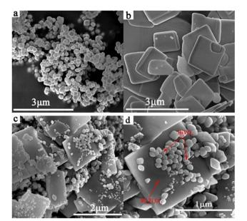
Fig. 8 SEM images of (a)  $BiVO_4$ , (b)  $Bi_4Ti_3O_{12}$ , and (c and d)  $BiVO_4/10\%$ Bi<sub>4</sub>Ti<sub>3</sub>O<sub>12</sub>.<sup>52</sup>
