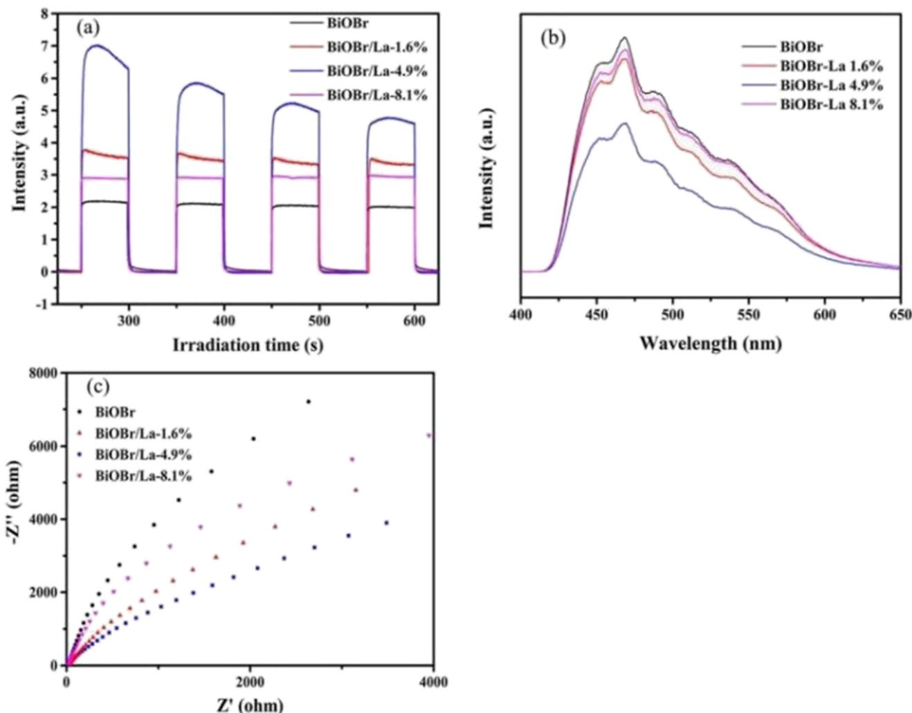
Fig. 18 Transient photocurrent curves (a), PL spectra (b), and EIS curves (c) for BiOBr and BiOBr/La catalysts.<sup>78</sup>
