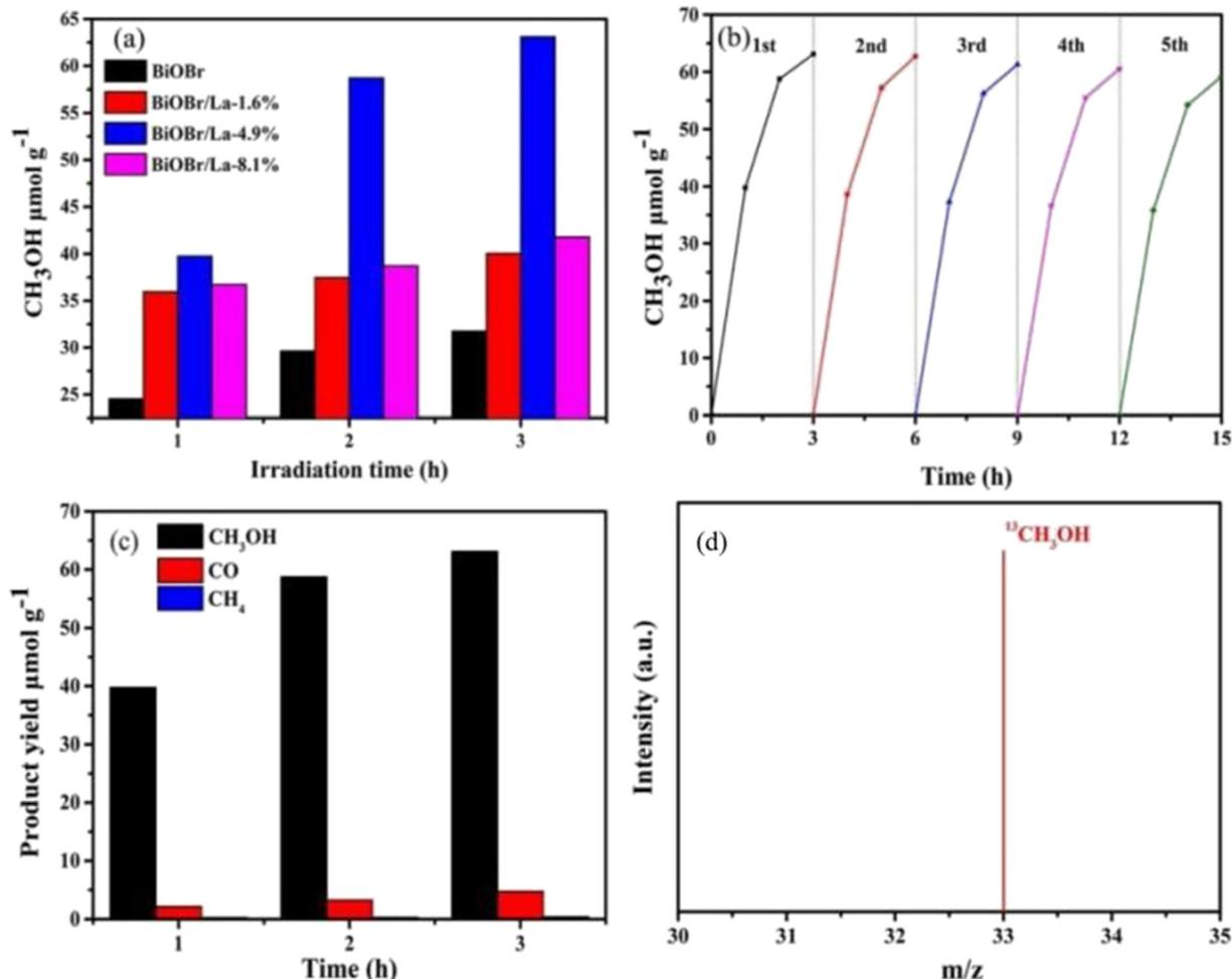
Fig. 19 (a) The yields of CH<sub>3</sub>OH for BiOBr and BiOBr/La catalysts, (b) cycling performance for BiOBr/La-4.9%, (c) products from CO<sub>2</sub> reduction on BiOBr/La-4.9% and (d) MS spectrum of CH<sub>3</sub>OH produced by <sup>13</sup>CO<sub>2</sub> reduction.<sup>78</sup>
