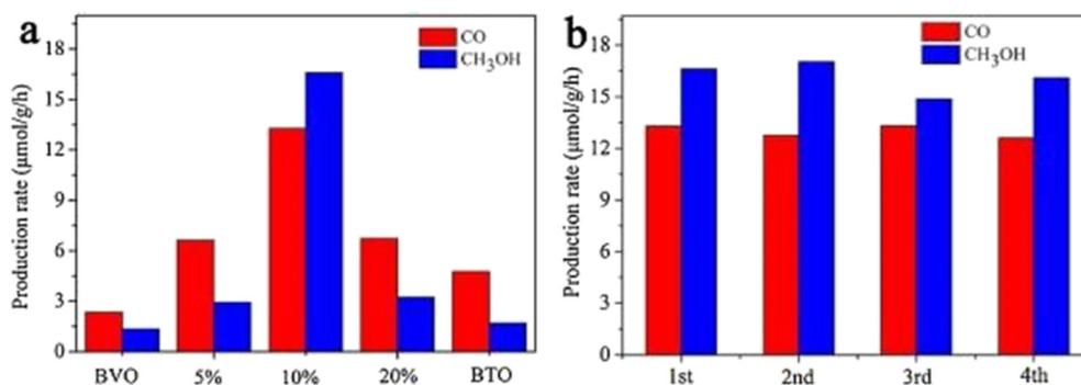
**Fig. 7** (a) CH<sub>3</sub>OH and CO evolutions on BiVO<sub>4</sub>/Bi<sub>4</sub>Ti<sub>3</sub>O<sub>12</sub> with different Bi<sub>4</sub>Ti<sub>3</sub>O<sub>12</sub> contents under a 300 W Xe lamp and (b) photocatalytic activity stability of the BiVO<sub>4</sub>/10% Bi<sub>4</sub>Ti<sub>3</sub>O<sub>12</sub> sample within 12 h with 3 h per circulation.<sup>52</sup>
