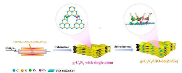
Fig. 4 Synthesis process of the q-C<sub>3</sub>N<sub>4</sub>/UiO-66 (Zr/Ce) photocatalyst.<sup>28</sup>
