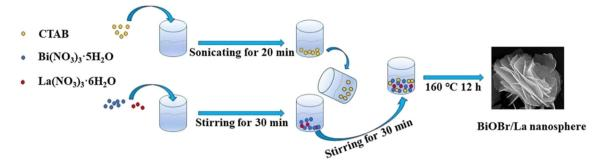
Fig. 16 Process diagram of BiOBr/La synthesis.<sup>78</sup>
