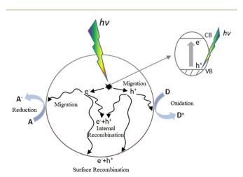
Fig. 1 Photocatalytic process of a semiconductor.
