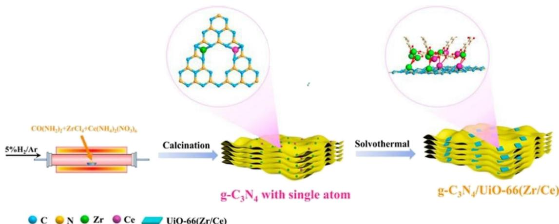
Fig. 4 Synthesis process of the  $g\text{-C}_3\text{N}_4/\text{UiO-66 (Zr/Ce)}$  photocatalyst.<sup>28</sup>
