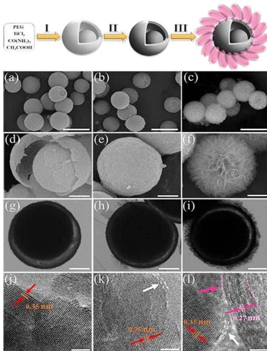
Fig. 3 Overall flowchart for the fabrication of the 3D Y@S TiO<sub>2-x</sub>/LDH architecture (steps I-III); corresponding (a-f) FESEM, (g-i) TEM, and (j-l) HRTEM images of the 3D Y@S TiO<sub>2-x</sub>/LDH sites.<sup>13</sup>
