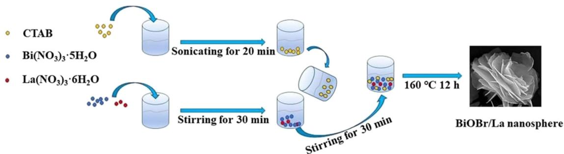
Fig. 16 Process diagram of BiOBr/La synthesis.<sup>78</sup>
