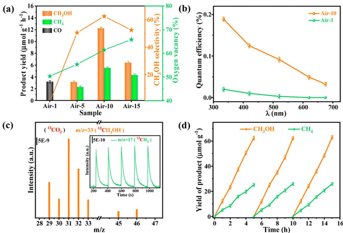
Fig. 11 (a) Product yields, CH<sub>3</sub>OH selectivity and oxygen vacancy content of different photocatalysts. (b) QE values of air-1 and air-10, respectively. (c) GC-MS spectra of <sup>13</sup>CH<sub>3</sub>OH and <sup>13</sup>CH<sub>4</sub> generated from <sup>13</sup>CO<sub>2</sub> photoreduction of air-10. (d) Photocatalytic stability of air-10.<sup>53</sup>
