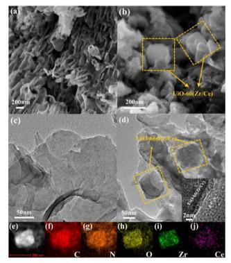
Fig. 5 SEM images of (a) g-C<sub>3</sub>N<sub>4</sub> and (b) g-C<sub>3</sub>N<sub>4</sub>/UiO-66 (Zr/Ce); TEM images of (c)  $g-C_3N_4$  and (d)  $g-C_3N_4/UiO-66$  (Zr/Ce); (e-j) EDS mapping of g-C<sub>3</sub>N<sub>4</sub>/UiO-66 (Zr/Ce).<sup>28</sup>
