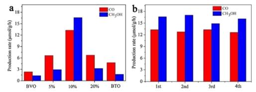
Fig. 7 (a) CH<sub>3</sub>OH and CO evolutions on  $BiVO_4/Bi_4Ti_3O_{12}$  with different  $Bi_4Ti_3O_{12}$  contents under a 300 W Xe lamp and (b) photocatalytic activity stability of the  $BiVO_4/10\%$   $Bi_4Ti_3O_{12}$  sample within 12 h with 3 h per circulation.<sup>52</sup>
