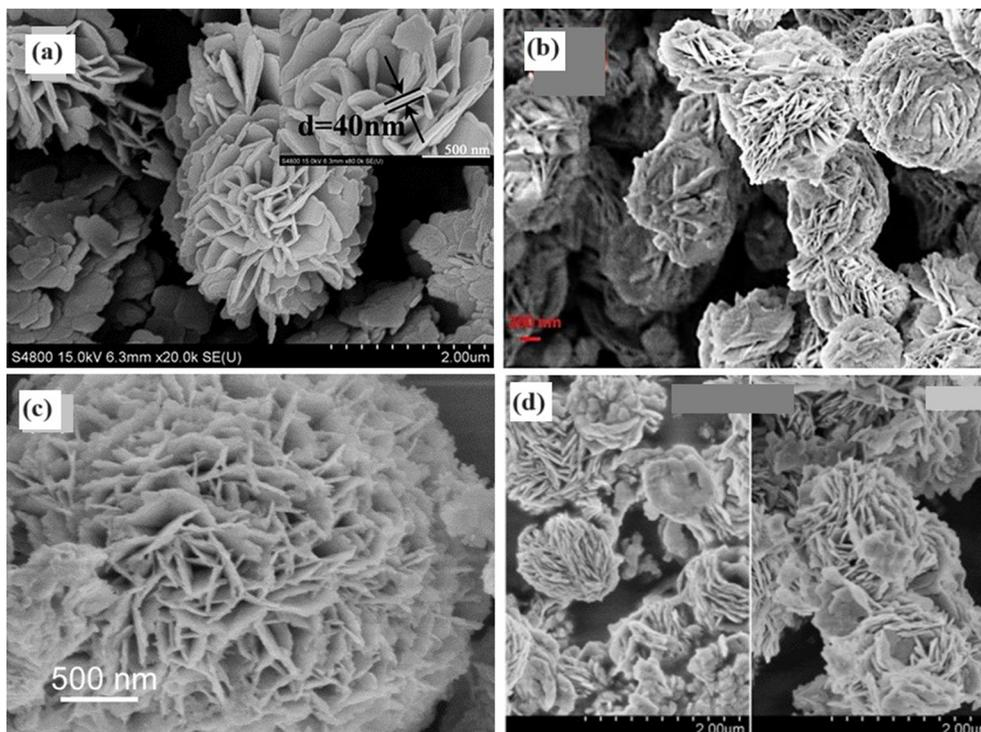
**Fig. 12** The morphologies of the 3D structures of a)  $\text{BiOCl}_{1-x}\text{Br}_x$ . Reprinted with permission from ref. 115. Copyright (2016) Elsevier; b)  $\text{G-BiOBr}_x\text{I}_{1-x}$  composites. Reprinted with permission from ref. 116. Copyright (2019) Elsevier; c)  $\text{BiOCl}_2\text{I}$ . Reprinted with permission from ref. 120. Copyright (2016) Elsevier; and d)  $\text{BiOCl}_x\text{Br}_y\text{I}_z$ . Reprinted with permission from ref. 117. Copyright (2015) Elsevier.
