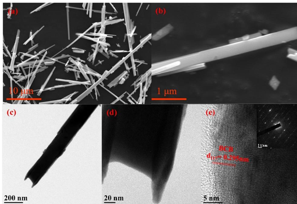
Fig. 10 a and b) SEM, c and d) TEM, and e) high-resolution TEM images of 1D  $\text{Bi}_{12}\text{O}_{17}\text{ClBr}$  nanotubes. Reprinted with permission from ref. 100. Copyright (2020) Elsevier.
