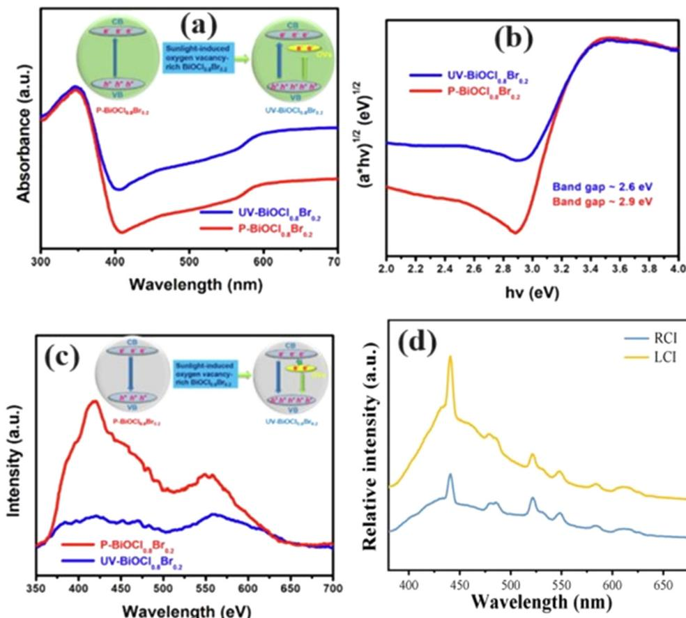
Fig. 13 a) UV-vis diffuse reflectance spectra, b) band gap energies from Tauc plots, c) photoluminescence emission spectra of the P-BiOCl<sub>0.8</sub>Br<sub>0.2</sub> and UV-BiOCl<sub>0.8</sub>Br<sub>0.2</sub>. Reprinted with permission from ref. 122. Copyright (2022) Elsevier; d) PL spectra of BiOCl<sub>0.5</sub>I<sub>0.5</sub> rich in OV (RCI) and BiOCl<sub>0.5</sub>I<sub>0.5</sub> less rich in OV (LCI). Reprinted with permission from ref. 125. Copyright (2022) Elsevier.
