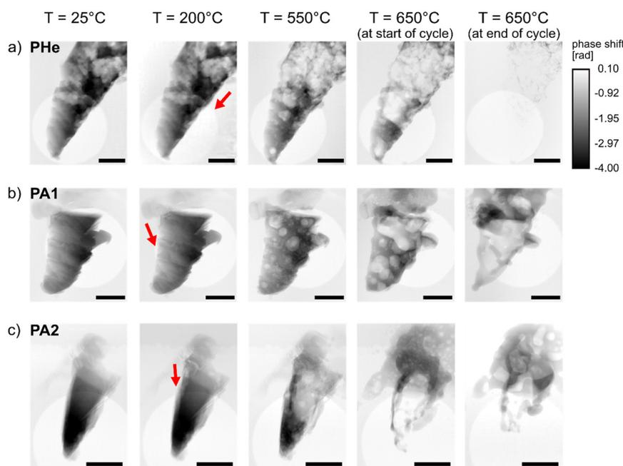
**Fig. 2** *In situ* X-ray ptychography projections of a) PHe, b) PA1, and c) PA2 as a function of applied temperature for  $T = 25, 200, 550,$  and  $650$  °C (showing start and end of the constant temperature cycle) under their respective gas environment. The red arrows indicate both bubble formation and the direction of bubble propagation. All scale bars =  $2.4$   $\mu\text{m}$ .
