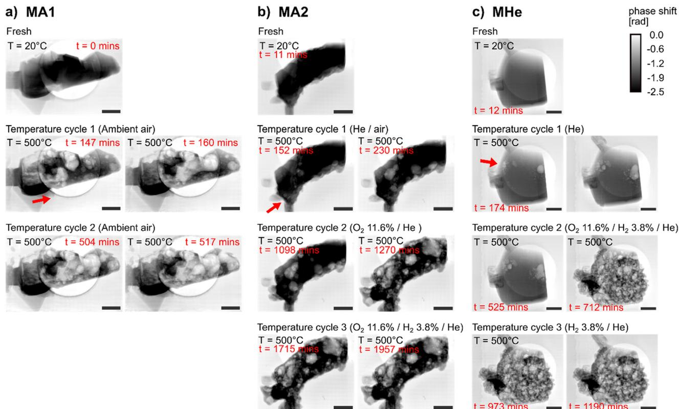
**Fig. 4** *In situ* X-ray ptychography projections of samples a) MA1, b) MA2, and c) MHe. The top row for each sample shows the fresh sample. The subsequent rows for each sample exhibit morphological changes at the start and end of each constant temperature condition of 500 °C, under their respective environments. The red arrows indicate bubble formation and the direction of bubble propagation. All scale bars = 2  $\mu\text{m}$ .
