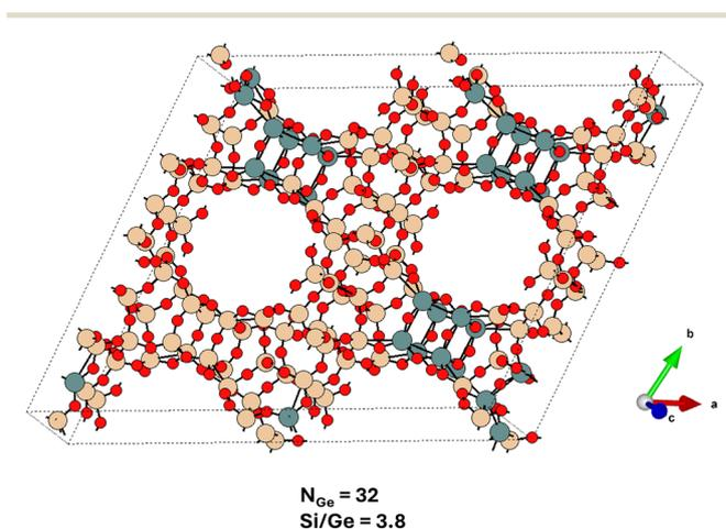
**Fig. 6** The global structure optimum for the UTL system with  $\text{Si}/\text{Ge} = 3.8$  adopting a large simulation cell (Table S4<sup>†</sup>) – compare with Fig. 4. The Ge content at this  $\text{Si}/\text{Ge}$  ratio allows for a complete filling of D4R units with germanium atoms, however, a partial spillover of Ge atoms towards the non-D4R T sites is observed. The structure is viewed approximately along the c-axis.
