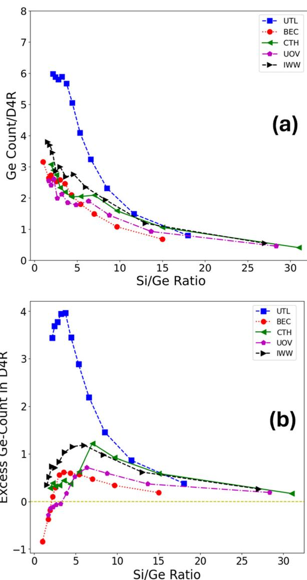
**Fig. 2** Quantification of the D4R occupation by germanium across a range of Si/Ge ratios and all zeolite topologies considered, using the metrics defined in section 2.3, namely: (a) Ge count/D4R, and (b) excess Ge-count in D4R, measuring the excess occupation of D4R units by germanium compared to the case of uniform germanium distribution (yellow dashed line) across all the T sites.
