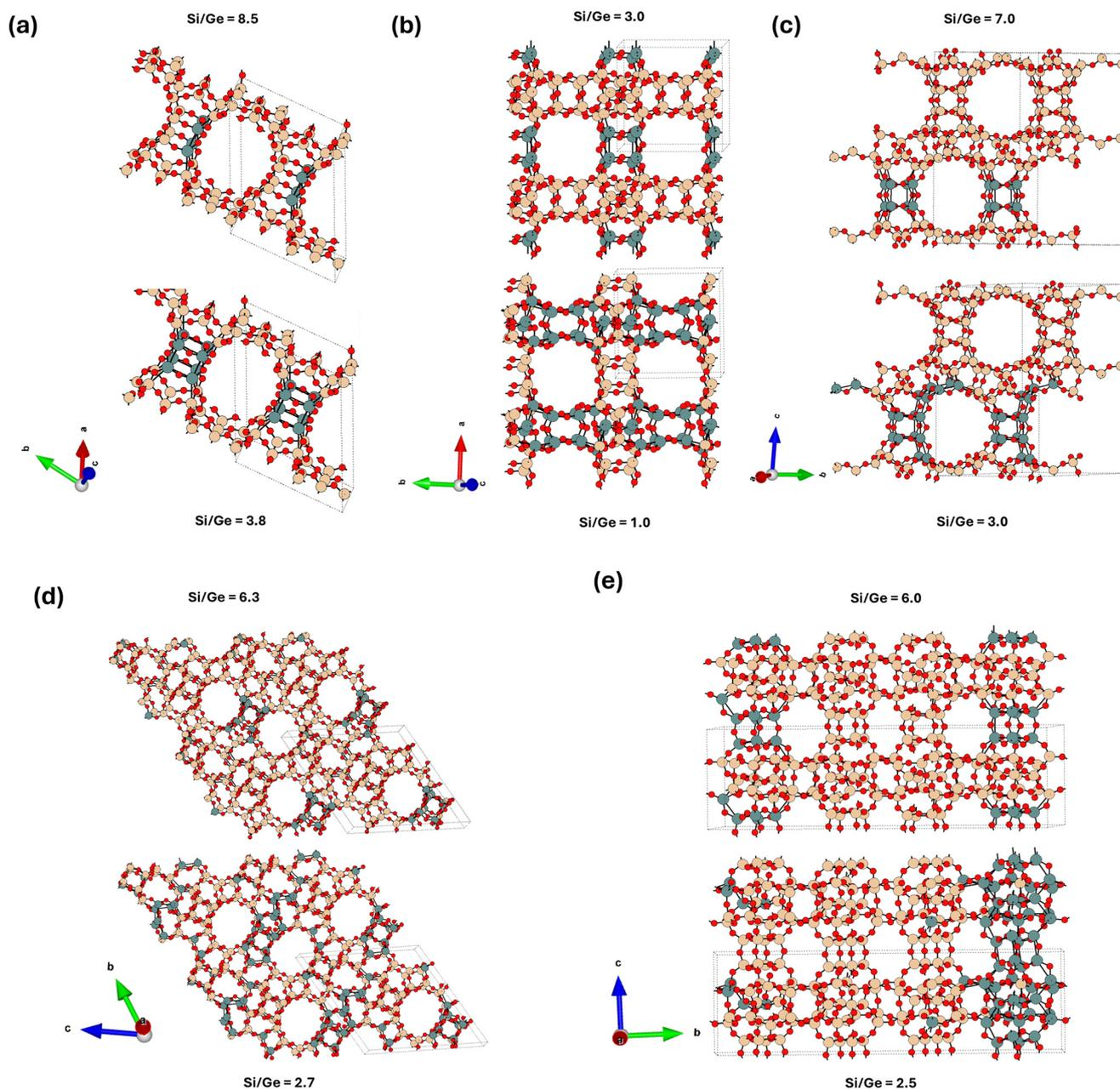
Fig. 4 The structures of the lowest-energy germanium distributions for the (a) UTL, (b) BEC, (c) CTH, (d) UOV, and (e) IWW topologies. For each topology, the global structure optima for two specific Si/Ge ratios are depicted, corresponding to the Ge loading sufficient to fill half (above) and all (below) of the D4R T sites.
