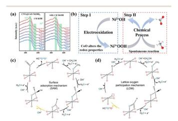
Fig. 2 (a) In situ Raman spectra of the OER and MOR for CNTs@CoO-Ni(OH)<sub>2</sub>. (b) Dynamic reconstruction of the active Ni<sup>3+</sup>OOH layer.<sup>56</sup> Reproduced from ref. 56 with permission from the Royal Society of Chemistry, Copyright 2023. Possible reaction mechanisms for (c) SAM and (d) LOM.63 Reproduced from ref. 63 with permission from American Association for the Advancement of Science, Copyright 2023.
