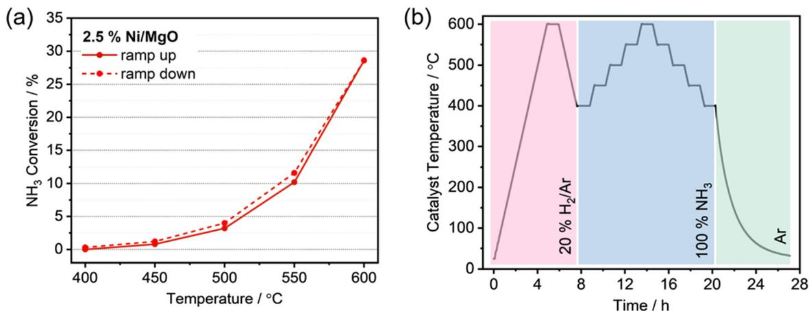
Fig. 1 (a) Ammonia decomposition over a 2.5% Ni/MgO catalyst (ID S82 of the catalyst precursor in the example database created for this publication, which can be accessed via the link <https://haber.archive.fhi.mpg.de>); (b) workflow for rapid testing of ammonia decomposition catalysts; further parameters are: feed composition 100% NH<sub>3</sub>, volume flow (W/F) 36 000 NmL h<sup>-1</sup> g<sup>-1</sup>, *p* = 1 bar.
