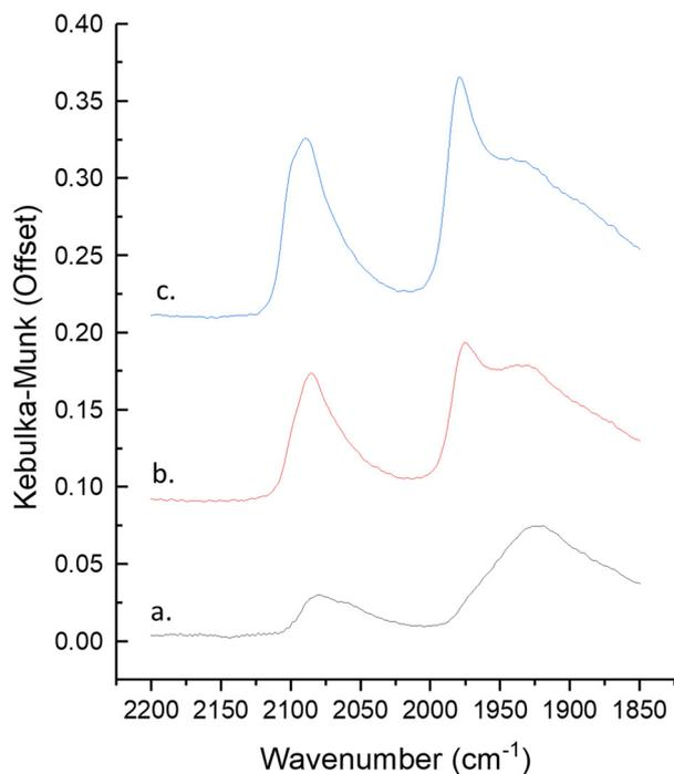
Fig. 5 DRIFT spectra of CO adsorbed at room temperature for (a.) 1.0 wt% Pd/Al<sub>2</sub>O<sub>3</sub>, (b.) 2.5 wt% Pd/Al<sub>2</sub>O<sub>3</sub> and (c.) 5.0 wt% Pd/Al<sub>2</sub>O<sub>3</sub> catalysts.
