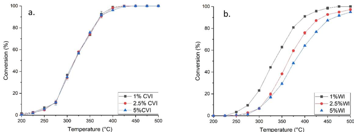
**Fig. 6** Propane conversion as a function of temperature for Pd/Al<sub>2</sub>O<sub>3</sub> catalysts synthesised by a. CVI and b. WI when the volume of sample was varied to normalise activity to Pd sites. (Black square) 1.0 wt% Pd/Al<sub>2</sub>O<sub>3</sub>, (red circle) 2.5 wt% Pd/Al<sub>2</sub>O<sub>3</sub>, (blue triangle) 5.0 wt% Pd/Al<sub>2</sub>O<sub>3</sub>. Reaction conditions: 1000 ppm propane/10% O<sub>2</sub>/N<sub>2</sub>, temperature range 200–500 °C.
