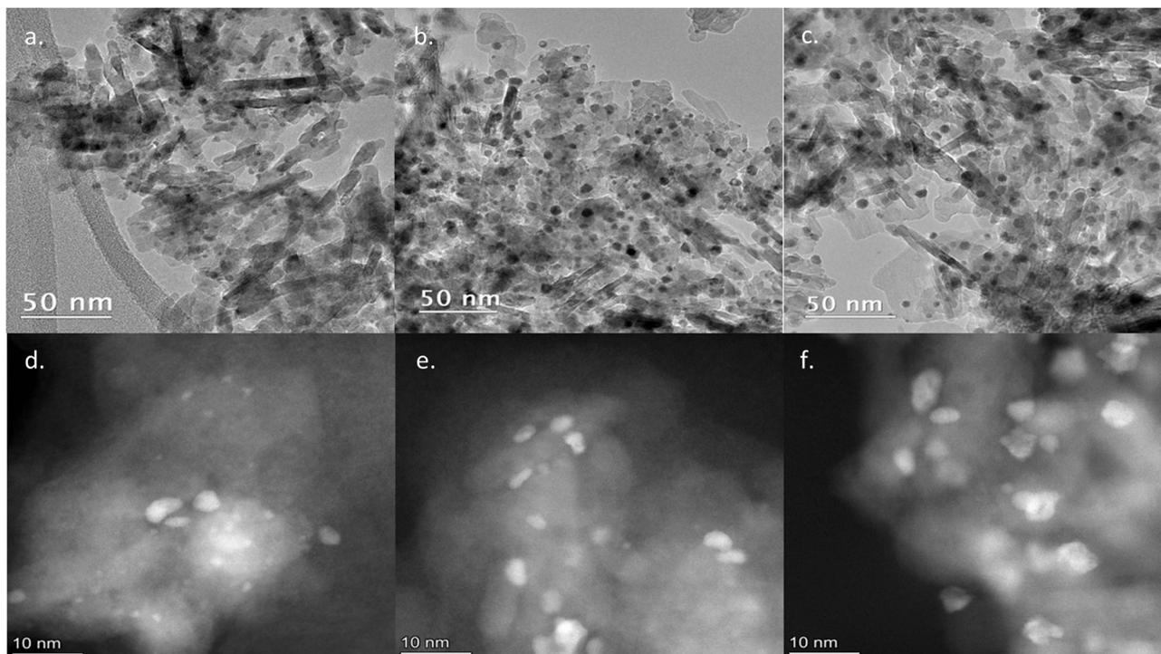
**Fig. 2** Electron microscopy micrographs of the catalysts prepared by CVI. a–c: TEM images (50 $\times$  magnification), d–f: AC-STEM images (80 $\times$  magnification). a and d: 1.0 wt% CVI, b and e: 2.5 wt% CVI, c and f: 5.0 wt% CVI.
