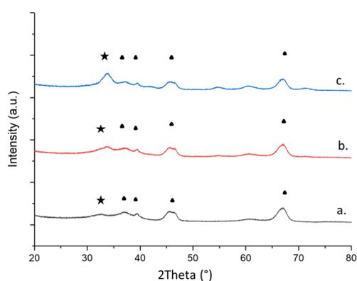
**Fig. 3** XRD patterns of (a.) 1.0 wt% Pd/Al<sub>2</sub>O<sub>3</sub>, (b.) 2.5 wt% Pd/Al<sub>2</sub>O<sub>3</sub> and (c.) 5.0 wt% Pd/Al<sub>2</sub>O<sub>3</sub> catalysts. (Black star) PdO, JCPDS no. 00-006-0515. (Black triangle)  $\gamma$ -Al<sub>2</sub>O<sub>3</sub>, JCPDS no. 10-0425.
