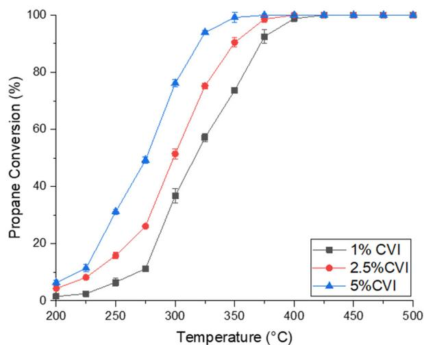
**Fig. 1** Propane conversion as a function of temperature for the Pd/ $\text{Al}_2\text{O}_3$  catalysts synthesised by chemical vapour impregnation. (Black square) 1.0 wt% Pd/ $\text{Al}_2\text{O}_3$ , (red circle) 2.5 wt% Pd/ $\text{Al}_2\text{O}_3$ , (blue triangle) 5.0 wt% Pd/ $\text{Al}_2\text{O}_3$ . Reaction conditions: 1000 ppm propane/10%  $\text{O}_2/\text{N}_2$ , gas hourly space velocity (GHSV)  $50\,000 \text{ h}^{-1}$ , temperature range 200–500 °C.
