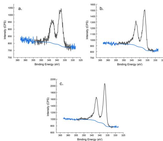
**Fig. 4** Pd 3d core-level XPS spectra for (a.) 1.0 wt% Pd/Al<sub>2</sub>O<sub>3</sub>, (b.) 2.5 wt% Pd/Al<sub>2</sub>O<sub>3</sub> and (c.) 5.0 wt% Pd/Al<sub>2</sub>O<sub>3</sub> catalysts.
