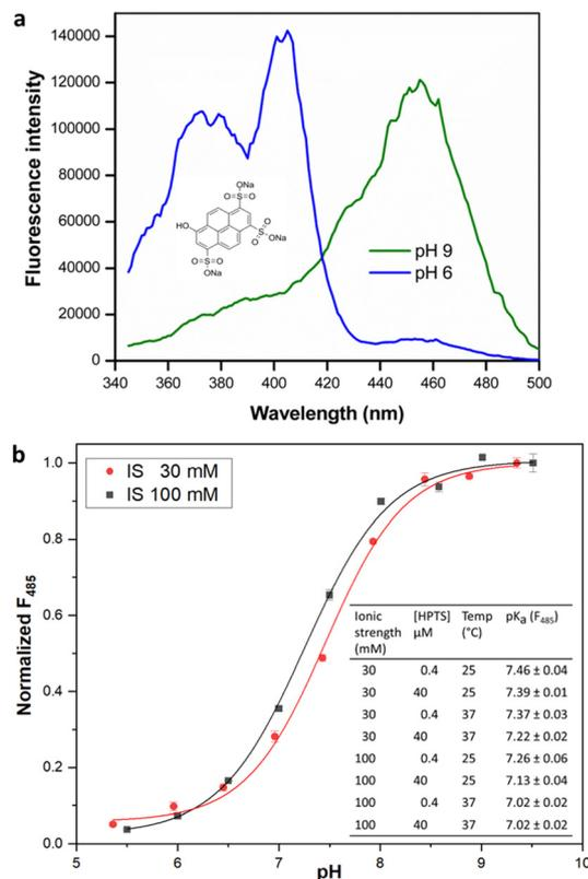
**Fig. 1** (a) HPTS structure (inset) and fluorescence excitation spectra,  $\lambda_{em} = 511$  nm. (b) Dependence of fluorescence intensity (485 nm) of HPTS on pH at 25  $^{\circ}$ C. Inset:  $pK_a$  estimates for HPTS under different reaction conditions. Fluorescence measurements were made as described in methods.  $pK_a$  values are given as mean  $\pm$  SD ( $n = 3$ ).
