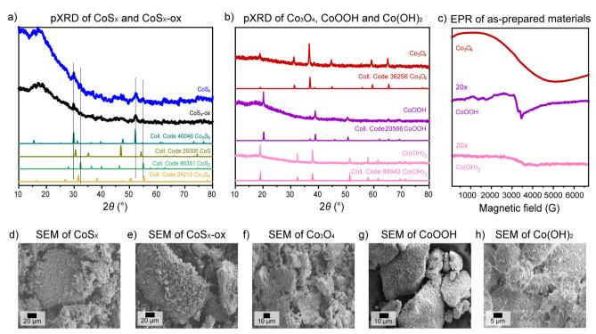
Fig. 1 Bulk characterization of all as-prepared materials by (a and b) pXRD with comparison to literature diffraction pattern of different cobalt sulfide phases, Co<sub>3</sub>O<sub>4</sub>, CoOOH, or Co(OH)<sub>2</sub>. Reference pXRD patterns were obtained from the Inorganic Crystal Structure Database (ICSD). Analysis by (c) EPR, where the EPR spectra of CoOOH and Co(OH)<sub>2</sub> have been vertically scaled to show minor signals, and by (d-h) SEM.
