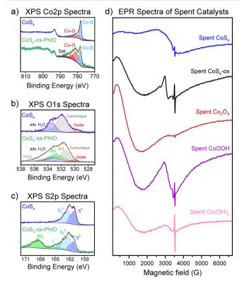
Fig. 4 a) Co 2p, b) O 1s, and c) S 2p XPS spectra of  $CoS_x$  (blue) and  $\mathsf{CoS}_{\mathsf{x}}\text{-}\mathsf{ox}\text{-}\mathsf{PhIO}$  (green). The XPS spectra of  $\mathsf{CoS}_{\mathsf{x}}$  are replicated from Fig. 2 for a more convenient comparison. d) EPR spectra of spent (post-catalytic) CoS<sub>x</sub> (blue), CoS<sub>x</sub>-ox (black), Co<sub>3</sub>O<sub>4</sub> (red), CoOOH (purple), and Co(OH)2 (pink).
