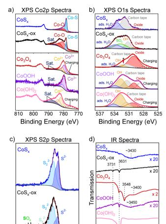
Fig. 2 XPS Co 2p (a), O 1s (b), and S 2p spectra (c) and IR spectra (d) of  $CoS_x$  (blue),  $CoS_x$ -ox (black),  $Co_3O_4$  (red), CoOOH (purple), and Co(OH)<sub>2</sub> (pink). Fitted components to the XPS spectra are shown as colored peaks. The asterisk in (b) denotes an instrumental artefact. Individual IR spectra have been vertically scaled as indicated on the right in (d) to show low intensity bands.
