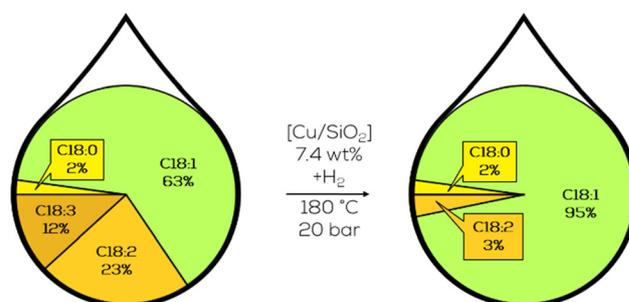
Fig. 19 Composition of the C18 fatty acid fraction in the selective hydrogenation of canola oil as performed by Zaccheria.<sup>113</sup>
