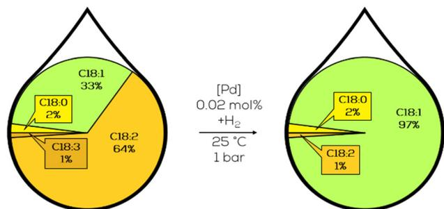
Fig. 39 Fatty acid composition of the C18 fraction in the partial hydrogenation of sunflower oil-derived methyl ester as performed by Behr *et al.*<sup>195</sup>
