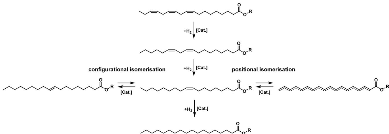
Fig. 5 Simplified reaction scheme of linolenate hydrogenation.<sup>30,43</sup>
