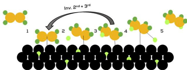
Fig. 10 Hydrogenation mechanism postulated by Horiuti and Polanyi.<sup>77</sup>
