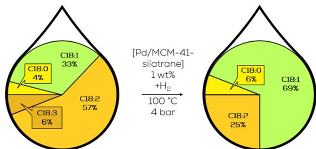
Fig. 24 C18 fatty acid composition in the hydrogenation of soybean oil-derived methyl ester over heterogeneous Pd catalysts with silatrane doped SiO<sub>2</sub> support structure as performed by Luengnaruemitchai.<sup>136</sup>
