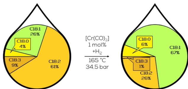
Fig. 31 C18 fatty acid composition in the hydrogenation of soybean oil by chromium carbonyl complexes as performed by Frankel *et al.*<sup>172</sup>
