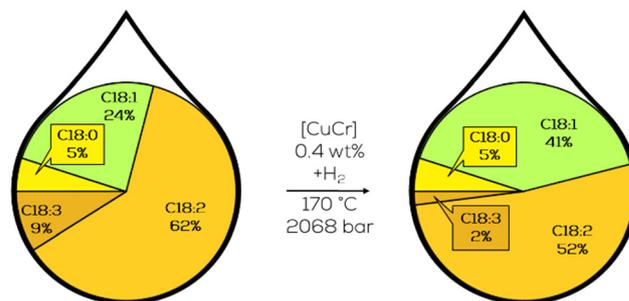
Fig. 12 C18 fatty acid composition in the hydrogenation of soybean oil under high hydrogen pressure as performed by Koritala *et al.*<sup>95</sup>
