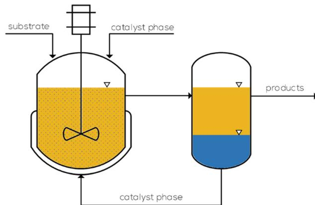
Fig. 35 Concept for reactions with a homogeneous catalyst immobilized in the second aqueous phase.
