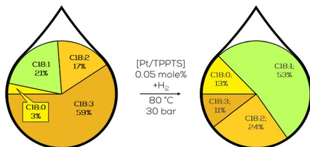
Fig. 36 Fatty acid composition of the C18 fraction in the partial hydrogenation of linseed oil-derived methyl ester as performed by Papadogianakis.<sup>189</sup>
