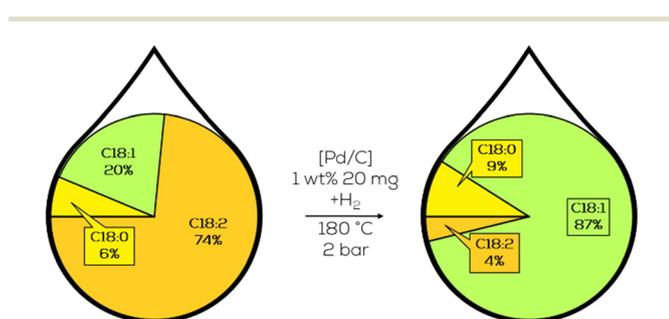
Fig. 20 Composition of the C18 fatty acid fraction in the selective hydrogenation of sunflower oil as performed by Romanenko.<sup>121</sup>
