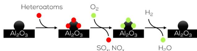
Fig. 23 Regeneration of heterogeneous Pd catalysts by oxygen from gaseous feed stream as proposed by research on sulphur Yoshimura.<sup>137</sup>
