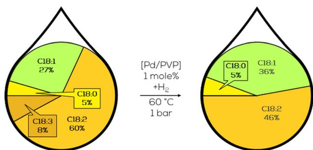
Fig. 37 Fatty acid composition of the C18 fraction in the partial hydrogenation of linseed oil-derived methyl ester as performed by Schumann and Bayer.<sup>190</sup>
