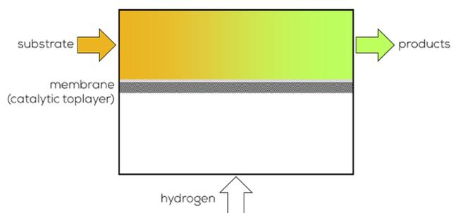
Fig. 43 Crossflow configuration for membrane reactors as used by Rezac.<sup>205</sup>
