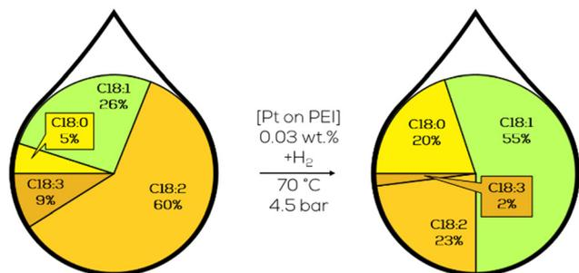
Fig. 44 Fatty acid composition of the C18 fraction in the partial hydrogenation of soybean oil in a cross-flow membrane reactor as performed by Rezac.<sup>205</sup>
