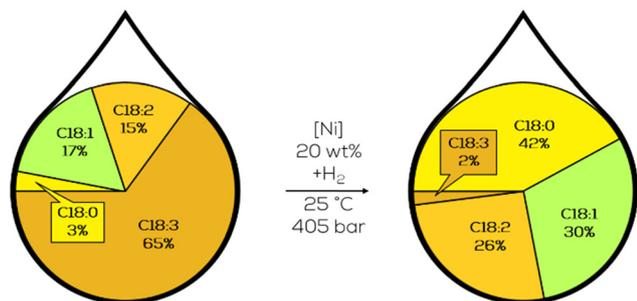
Fig. 9 C18 fatty acid composition in the hydrogenation of linseed oil performed by Normann.<sup>75</sup>
