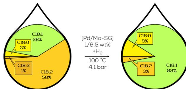
Fig. 26 C18 fatty acid composition in the hydrogenation of sunflower oil with Mo-doped Pd catalyst immobilized in sol-gel as performed by Tonetto.<sup>144</sup>
