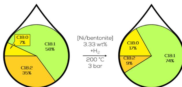
Fig. 29 Fatty acid composition of the C18 fraction in the hydrogenation of jatropa oil-derived methyl ester as performed by Wei.<sup>50</sup>
