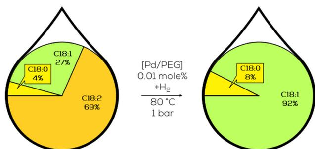
Fig. 40 Fatty acid composition of the C18 fraction in the partial hydrogenation of sunflower oil-derived methyl ester as performed by Wei Liu.<sup>201</sup>
