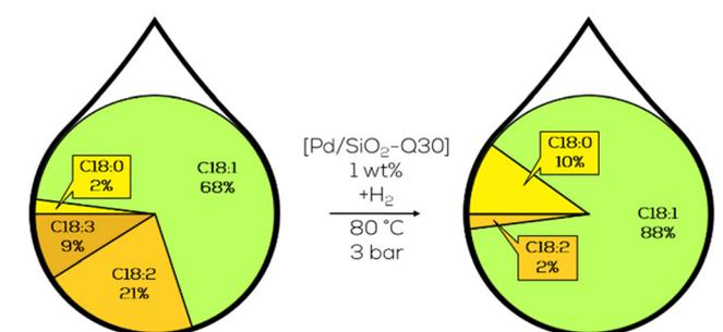
Fig. 21 C18 fatty acid composition in the hydrogenation of canola oil-derived biodiesel over macroporous Pd on SiO<sub>2</sub> as performed by Luengnaruemitchai.<sup>127</sup>
