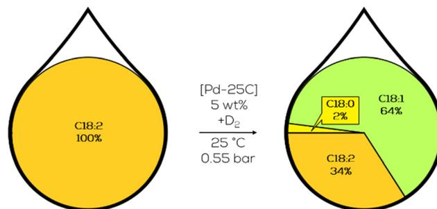
Fig. 17 C18 fatty acid composition in the deuteration of methyl linoleate with Pd on carbon as performed by Koritala *et al.*<sup>109</sup>
