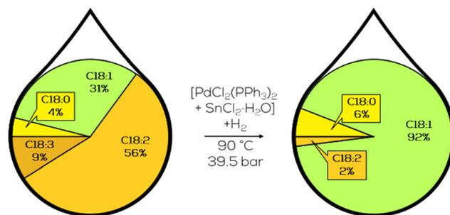
Fig. 33 C18 fatty acid composition in the selective hydrogenation of soybean methyl ester as performed by Bailar and Itatani.<sup>176</sup>
