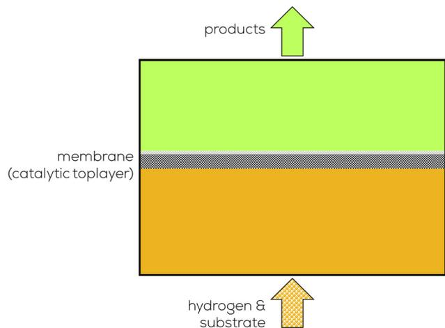
Fig. 41 Parallel-flow configuration for membrane reactors as used by Schomäcker.<sup>208</sup>
