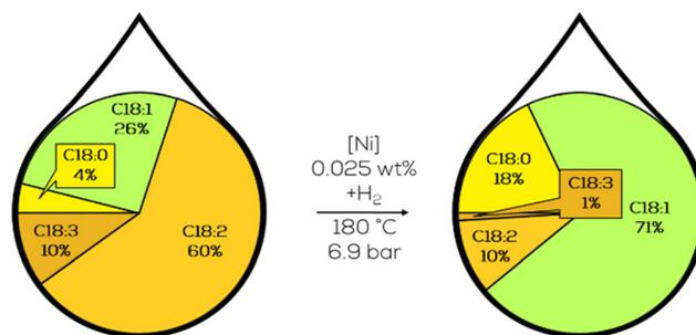
Fig. 16 C18 fatty acid composition in the continuous slurry hydrogenation of soybean oil in a co-current tubular flow reactor as described by Koritala *et al.*<sup>102</sup>
