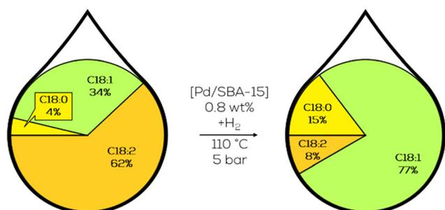
Fig. 25 Composition of the C18 fatty acid fraction in the selective hydrogenation of sunflower oil as performed by Belkacemi.<sup>142</sup>
