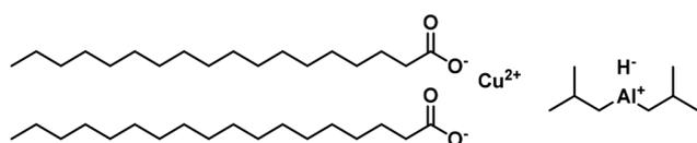
Fig. 15 Copper stearate and diisobutyl aluminium hydride precursors for homogeneously catalyzed hydrogenation of soybean oil, as used by Koritala *et al.*<sup>99</sup>
