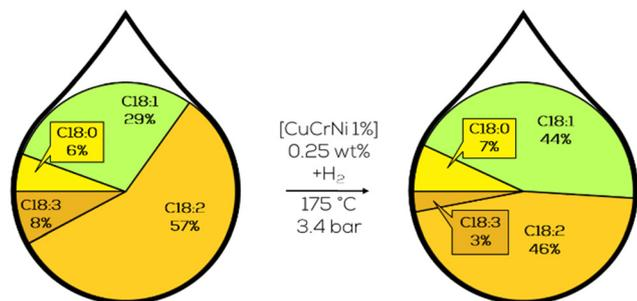
Fig. 11 C18 fatty acid composition in the hydrogenation of refined soybean oil with Ni-containing CuCr catalysts as performed by Griffin and co-workers.<sup>88</sup>
