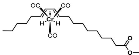
Fig. 30 Chromium carbonyl complex coordinating to conjugated diene used for hydrogenation of unsaturated fatty esters by Frankel *et al.*<sup>171</sup>
