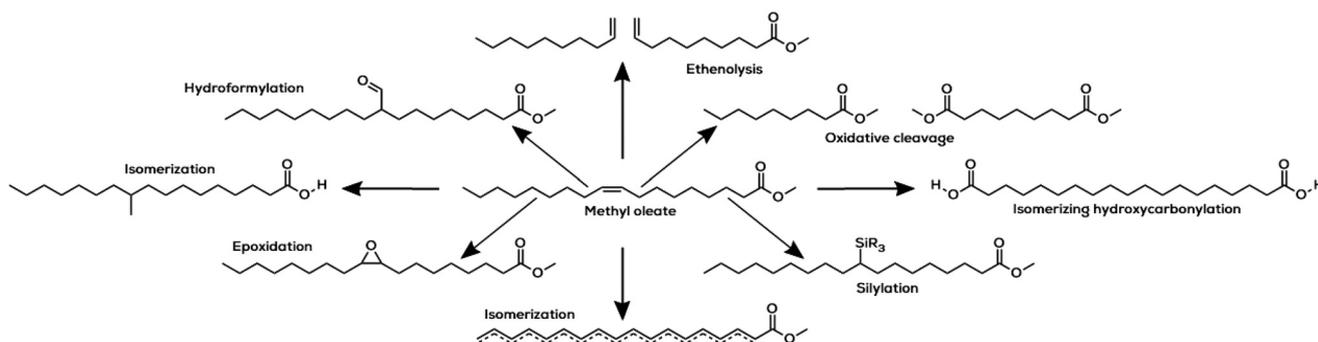
Fig. 4 Selection of homogeneously catalysed reactions reported with methyl oleate.<sup>11,23,42,43</sup>
