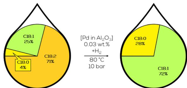
Fig. 42 Fatty acid composition of the C18 fraction in the hydrogenation of sunflower oil in a membrane reactor with a Pd-modified membrane in parallel flow configuration as performed by Schomäcker.<sup>209</sup>
