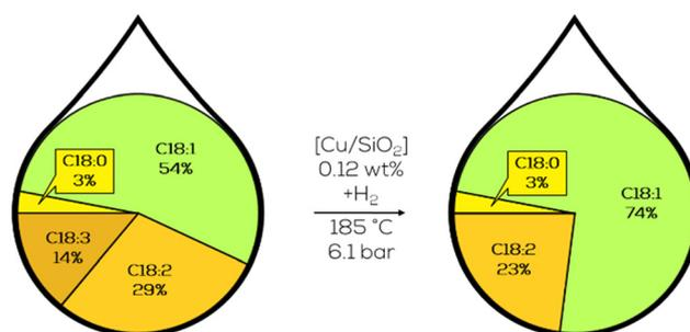
Fig. 13 C18 fatty acid composition in the hydrogenation of canola oil with heterogeneous copper catalysts immobilized on SiO<sub>2</sub> as performed by Johannsson *et al.*<sup>97</sup>
