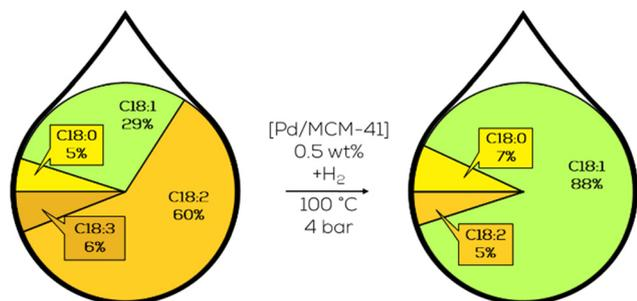
Fig. 22 C18 fatty acid composition in the hydrogenation of soybean oil-derived methyl ester focusing on increased *c*-C18:1 formation by 2 nm sized Pd-nanoparticles on MCM-41 as performed by Luengnaruemitchai.<sup>133</sup>
