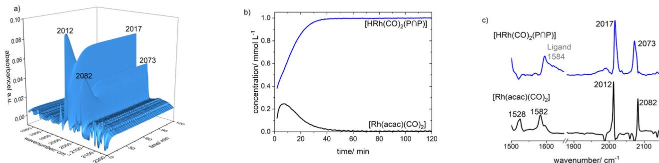
**Fig. 9** a) *In situ* IR-spectra from the catalyst formation in dependency of the time; b) concentration profiles and c) pure component spectra from the peak group analysis (PGA) of IR-spectroscopic data. Conditions:  $[\text{Rh}] = 1 \text{ mM}$ ,  $[\text{P}^{\text{N}}\text{P}] = 1 \text{ mmol}$ ,  $p(\text{CO}) = 1.0 \text{ MPa}$ ,  $p(\text{H}_2) = 1.0 \text{ MPa}$ ,  $\vartheta = 50 \text{ }^\circ\text{C}$ , solvent: cyclohexane.
