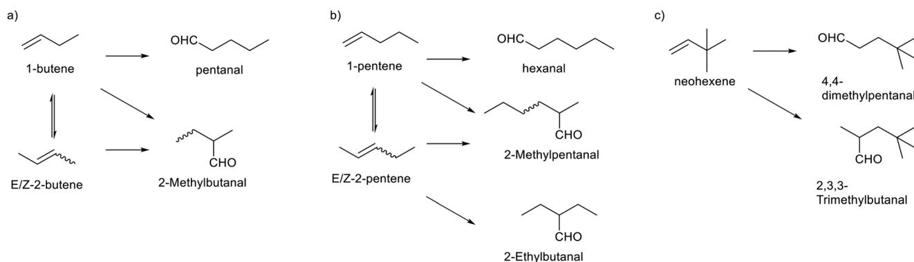
**Scheme 2** Isomerization–hydroformylation of a) butene, b) pentene and c) neohexene. Co-substrates  $\text{CO}$  and  $\text{H}_2$  have been left out as well as the catalyst  $[\text{HRh}(\text{CO})_2(\text{P}\cap\text{P})]$  for clarity.
