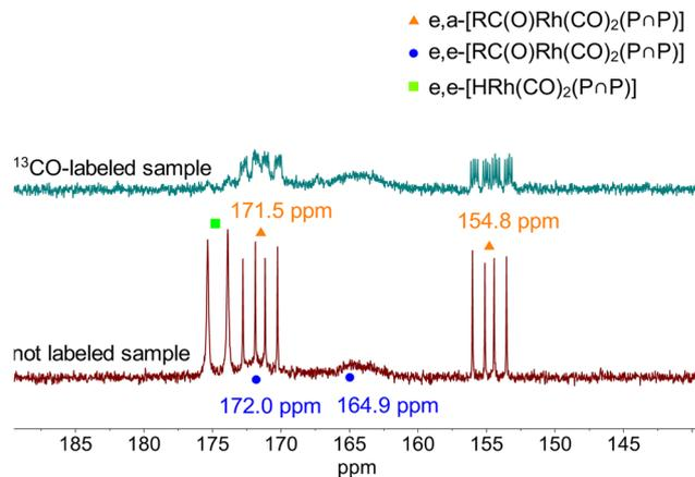
**Fig. 25**  $^{31}\text{P}\{^1\text{H}\}$ -NMR spectra of *e,a*- and *e,e*-[RC(O)Rh(CO)<sub>2</sub>(PnOP)] complexes at 253 K (bottom: without  $^{13}\text{C}$ -labeling and top: after  $^{13}\text{C}$  labeling). Further conditions: [Rh] = 20 mM, [PnOP] = 20 mM, [neohexene] = 80 mM,  $p(\text{CO})$  = 0.1 MPa, solvent: toluene- $d_8$ .
