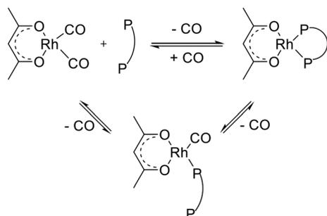
**Scheme 4** Formation of  $[Rh(acac)(PNP)]$  starting from  $[Rh(acac)(CO)_2]$  and BiPhePhos (PNP). The monocarbonyl complex  $[Rh(acac)(CO)(\kappa^1-PNP)]$  can be formed which highly depends on the reaction conditions.
