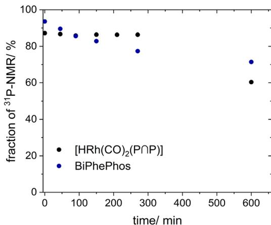
**Fig. 17** Hydrolysis control test. Integral fractions for  $[\text{HRh}(\text{CO})_2(\text{PNP})]$  (black) and BiPhePhos (blue) based on quant.  $^{31}\text{P}\{^1\text{H}\}$ -spectra. Further conditions:  $[\text{Rh}] = 20 \text{ mM}$ ,  $[\text{PNP}] = 20 \text{ mM}$ ,  $[\text{H}_2\text{O}]/[\text{PNP}] = 20$ ,  $p = 0.1 \text{ MPa}$ , solvent: 1,4-dioxane.
