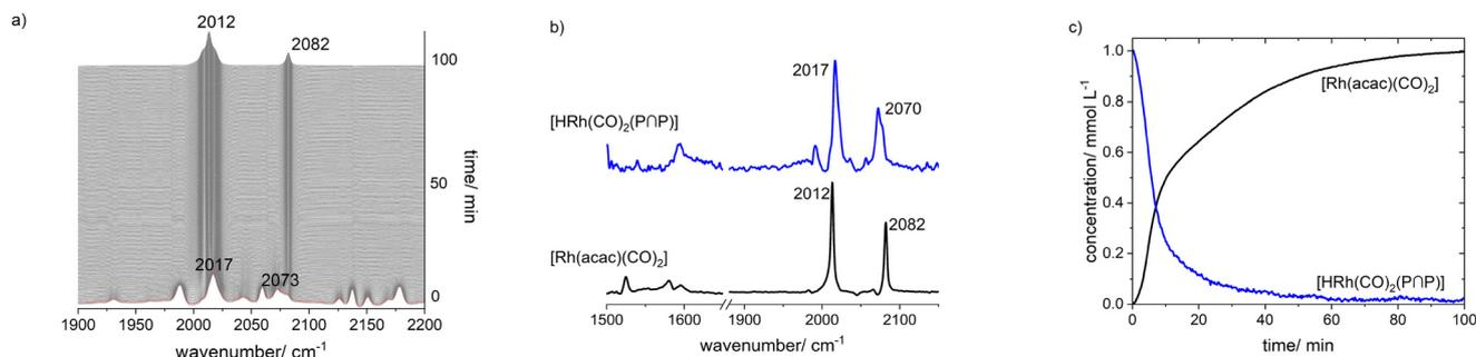
**Fig. 16** *In situ* IR-spectra series of the reaction of  $[\text{HRh}(\text{CO})_2(\text{PNP})]$  with air, b) pure component spectra extracted from a), c) corresponding relative absorbance profiles extracted with the peak group analysis. Conditions:  $[\text{Rh}] = 1 \text{ mM}$ ,  $[\text{PNP}] = 1 \text{ mM}$ ,  $p(\text{air}) = 0.3 \text{ MPa}$ ,  $\vartheta = 90 \text{ }^\circ\text{C}$ ,  $t = 90 \text{ min}$ , solvent: cyclohexane.
