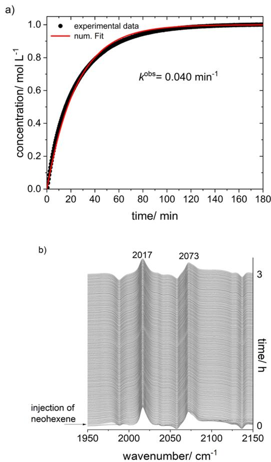
**Fig. 4** Neohexene hydroformylation using Rh/BiPhePhos catalyst. a) Concentration profile of 4,4-dimethyl-1-butene formation, b) *in situ* FTIR-spectra of the carbonyl region. Conditions: [Rh] = 1 mM, [P $\cap$ P] = 1 mM, [neohexene] = 1 M,  $t$  = 3 h,  $p(\text{H}_2)$  = 1.0 MPa,  $p(\text{CO})$  = 1.0 MPa,  $\vartheta$  = 90 °C, solvent: cyclohexane.
