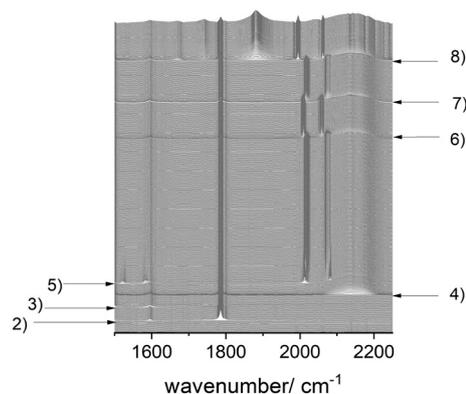
**Fig. 5** *In situ* spectroscopic IR-data of a sequential dosage experiment. Conditions: [Rh] = 1 mM, [P $\cap$ P] = 1 mM, [DPC] = 2 mM,  $p(\text{H}_2/\text{D}_2)$  = 1.0 MPa,  $p(\text{CO})$  = 1.0 MPa,  $p(\text{C}_2\text{H}_4)$  = 1.0 MPa,  $\vartheta$  = 50 °C, solvent: cyclohexane.
