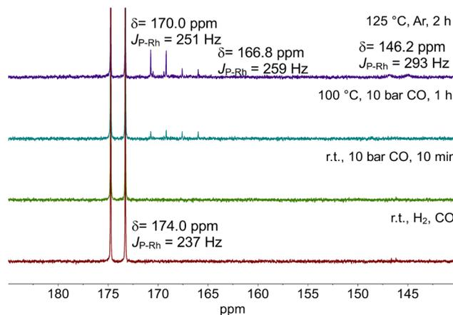
**Fig. 15**  $^{31}\text{P}\{^1\text{H}\}$ -spectra of  $[\text{HRh}(\text{CO})_2(\text{PNP})]$  under syngas, CO and Ar at varying temperatures. Further conditions:  $[\text{Rh}] = 20 \text{ mM}$ ,  $[\text{PNP}] = 20 \text{ mM}$ ,  $p = 0.1 \text{ MPa}$ , solvent: toluene- $d_8$ .
