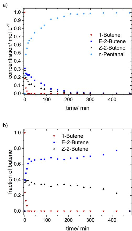
**Fig. 2** Concentration profiles of butene isomers and *n*-pentanal obtained for the 1-butene hydroformylation experiment. a) Absolute concentrations versus time and b) relative molar fractions of the butene isomers over time. Conditions: [Rh] = 1 mM, [P $\cap$ P] = 1 mM, [1-butene] = 1 M,  $t$  = 8 h,  $p(\text{H}_2)$  = 1.0 MPa,  $p(\text{CO})$  = 1.0 MPa,  $\vartheta$  = 90 °C, solvent: cyclohexane.
