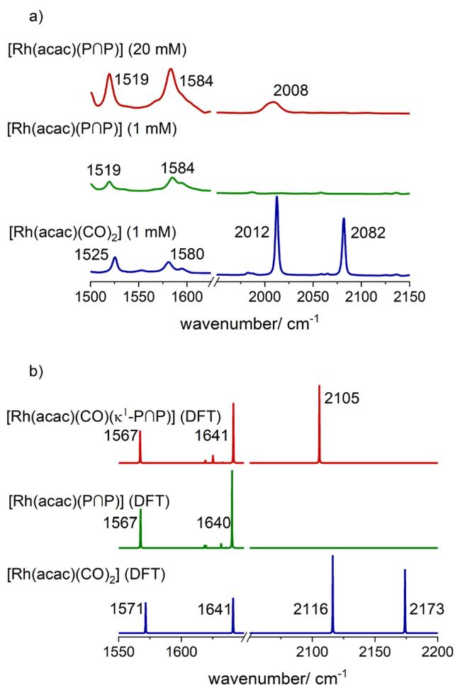
**Fig. 7** a) *In situ* IR-spectra of  $[Rh(acac)(CO)_2]$  and  $[Rh(acac)(PNP)]$  and b) DFT-based vibrational spectra (ESI-††). Conditions:  $[Rh] = 1 \text{ mM}$ ,  $[PNP] = 1 \text{ mM}$ ,  $p(Ar) = 0.1 \text{ MPa}$ ,  $\vartheta = 30 \text{ }^\circ\text{C}$ , solvent: cyclohexane.
