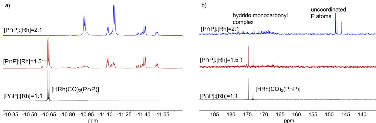
Fig. 19 a)  $^1\text{H}\{^{31}\text{P}\}$ -NMR and b)  $^{31}\text{P}\{^1\text{H}\}$ -NMR spectra of rhodium hydride complexes in  $\text{H}_2$  atmosphere under variation of the ligand concentration (conditions:  $[\text{Rh}] = 20 \text{ mM}$ ,  $p(\text{H}_2) = 0.1 \text{ MPa}$ ,  $\vartheta = 25 \text{ }^\circ\text{C}$ , solvent: toluene- $d_8$ ).
