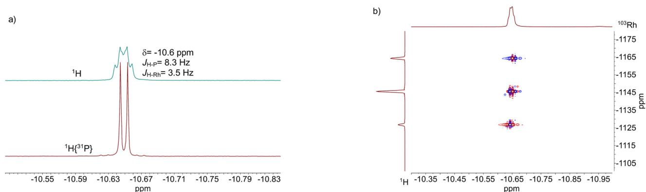
**Fig. 11** a)  $^1\text{H}$ -NMR and  $^1\text{H}({}^{31}\text{P})$ -NMR and b)  $^1\text{H}$ - $^{103}\text{Rh}$ -HMBC spectrum of  $[\text{HRh}(\text{CO})_2(\text{P}^{\text{N}}\text{P})]$ . Conditions:  $[\text{Rh}] = 20 \text{ mM}$ ,  $[\text{P}^{\text{N}}\text{P}] = 20 \text{ mM}$ ,  $p(\text{Ar}) = 0.1 \text{ MPa}$ ,  $\vartheta = 25 \text{ }^\circ\text{C}$ , solvent: toluene- $d_8$ .
