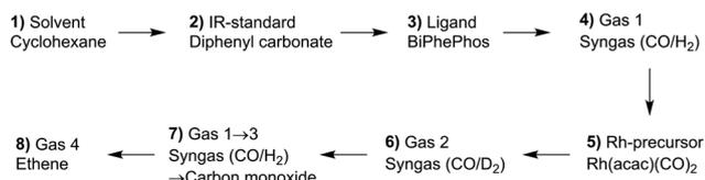
**Scheme 3** Sequence for the stepwise dosage experiment. Time interval between the steps was 10 min. Further reaction conditions:  $\vartheta$  = 50 °C, [Rh] = 1 mM, [P $\cap$ P] = 1 mM, [DPC] = 1 mM,  $P(\text{syngas})$  = 2.0 MPa,  $p(\text{ethene})$  = 1.0 MPa.
