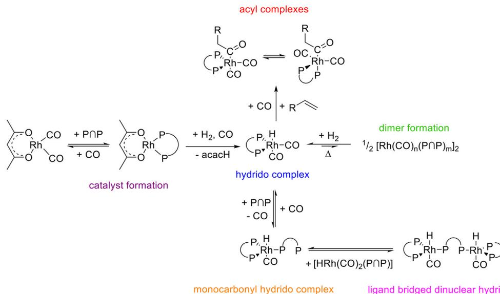
Fig. 26 Summary of the interconversions between diphosphite (BiPhePhos) modified rhodium complexes in the alkene hydroformylation.
