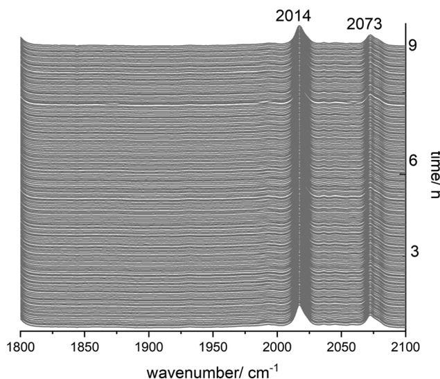
Fig. 14 *In situ* IR-spectroscopic data from the stability test of  $[\text{HRh}(\text{CO})_2(\text{P}\cap\text{P})]$  under an Ar atmosphere. Conditions:  $[\text{Rh}] = 1 \text{ mM}$ ,  $[\text{P}\cap\text{P}] = 1 \text{ mM}$ ,  $p(\text{Ar}) = 1.0 \text{ MPa}$ ,  $\vartheta = 90 \text{ }^\circ\text{C}$ , solvent: cyclohexane.
