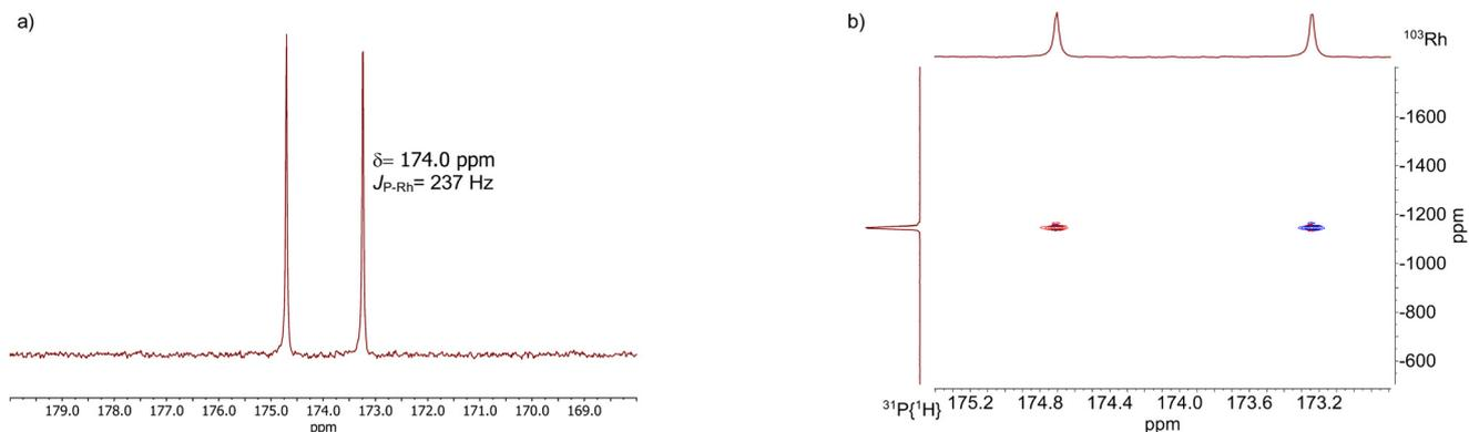
Fig. 12 a)  $^{31}\text{P}\{^1\text{H}\}$ -NMR of  $[\text{HRh}(\text{CO})_2(\text{P}\cap\text{P})]$  and b)  $^{31}\text{P}\{^1\text{H}\}$ - $^{103}\text{Rh}$ -HMBC spectrum (no decoupling) of  $[\text{HRh}(\text{CO})_2(\text{P}\cap\text{P})]$ . Conditions:  $[\text{Rh}] = 20 \text{ mM}$ ,  $[\text{P}\cap\text{P}] = 20 \text{ mM}$ ,  $p(\text{CO}) = 0.05 \text{ MPa}$ ,  $p(\text{H}_2) = 0.05 \text{ MPa}$ ,  $\vartheta = 25 \text{ }^\circ\text{C}$ , solvent: toluene- $d_8$ .
