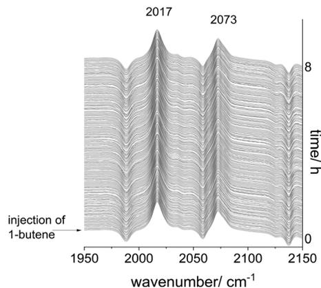
**Fig. 3** *In situ* FTIR-spectra measured during 1-butene hydroformylation. Conditions: [Rh] = 1 mM, [P $\cap$ P] = 1 mM, [1-butene] = 1 M,  $t$  = 8 h,  $p(\text{H}_2)$  = 1.0 MPa,  $p(\text{CO})$  = 1.0 MPa,  $\vartheta$  = 90 °C, solvent: cyclohexane.
