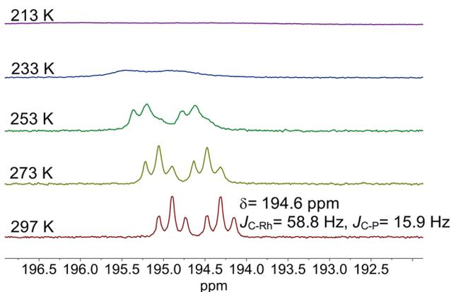
Fig. 13  $^{13}\text{C}\{^1\text{H}\}$ -NMR spectra of  $[\text{HRh}(\text{CO})_2(\text{P}\cap\text{P})]$  after isotopic labelling with 50%  $^{13}\text{C}$  under variation of the temperature. Conditions:  $[\text{Rh}] = 20 \text{ mM}$ ,  $[\text{P}\cap\text{P}] = 20 \text{ mM}$ ,  $p(^{12}\text{CO}) = 0.025 \text{ MPa}$ ,  $p(^{13}\text{CO}) = 0.025 \text{ MPa}$ ,  $p(\text{H}_2) = 0.05 \text{ MPa}$ , solvent: toluene- $d_8$ .
