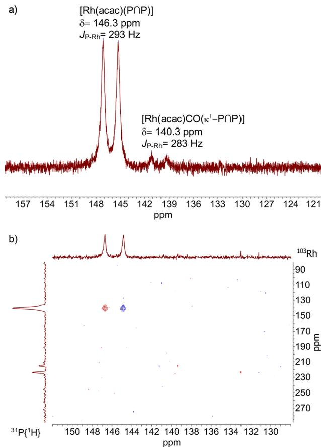
**Fig. 8** a)  $^{31}\text{P}\{^1\text{H}\}$ -NMR-spectrum of  $[\text{Rh}(\text{acac})(\text{P}\cap\text{P})]$  and b)  $^{31}\text{P}\{^1\text{H}\}$ - $^{103}\text{Rh}$ -NMR of  $[\text{Rh}(\text{acac})(\text{P}\cap\text{P})]$ . Conditions:  $[\text{Rh}] = 20$  mM,  $[\text{P}\cap\text{P}] = 20$  mM,  $p(\text{Ar}) = 0.1$  MPa,  $\vartheta = 25$  °C, solvent: toluene- $d_6$ ; spectrum b) was acquired at  $\vartheta = 30$  °C.
