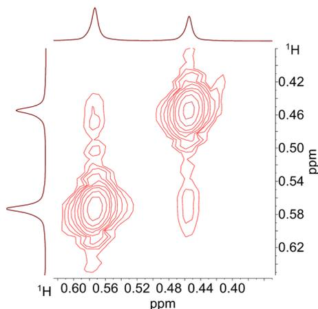
**Fig. 24**  $^1\text{H}$ - $^1\text{H}$ -EXSY spectrum of the equilibrium between *e,a*- and *e,e*-[RC(O)Rh(CO)<sub>2</sub>(PnOP)] complexes at 253 K. Further conditions: [Rh] = 20 mM, [PnOP] = 20 mM, [neohexene] = 80 mM,  $p(\text{CO})$  = 0.1 MPa, solvent: toluene- $d_8$ .
