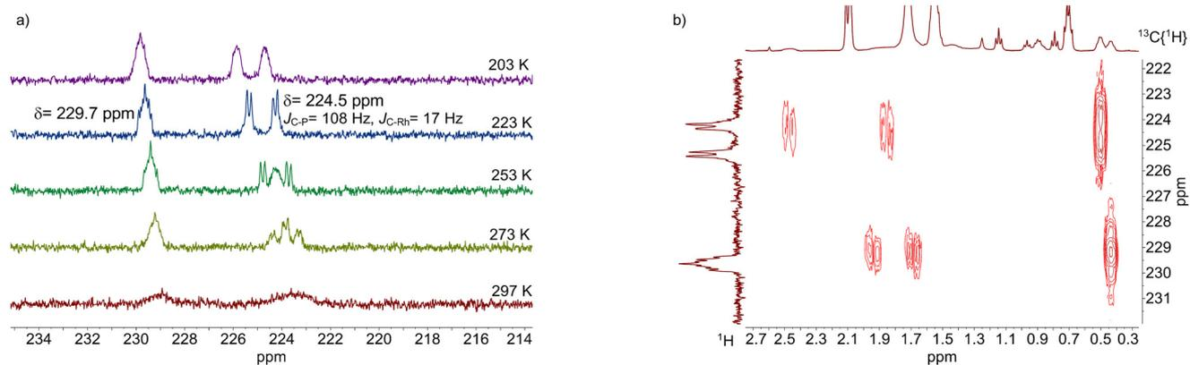
**Fig. 23** <sup>13</sup>C{<sup>1</sup>H}-NMR (a) and <sup>1</sup>H-<sup>13</sup>C-HMBC-NMR (b) spectra of stereoisomeric acyl complexes in a 5 mm sapphire tube after <sup>13</sup>CO labeling. Conditions: [Rh] = 20 mM, [PNP] = 20 mM,  $p(^{13}\text{CO}) = 1.0$  MPa,  $p(\text{C}_2\text{H}_4) = 1.0$  MPa, solvent: toluene-*d*<sub>8</sub>.
