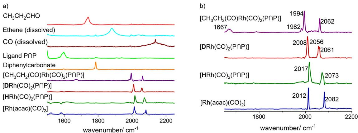
**Fig. 6** a) Extracted pure component spectra from the PGA processing of collected *in situ* spectroscopic IR-data of a sequential dosage experiment, b) selection of extracted spectra for rhodium carbonyl complexes (enlarged view). Conditions:  $[Rh] = 1 \text{ mM}$ ,  $[PNP] = 1 \text{ mM}$ ,  $[DPC] = 2 \text{ mM}$ ,  $p(H_2/D_2) = 1.0 \text{ MPa}$ ,  $p(CO) = 1.0 \text{ MPa}$ ,  $p(C_2H_4) = 1.0 \text{ MPa}$ ,  $\vartheta = 50 \text{ }^\circ\text{C}$ , solvent: cyclohexane.
