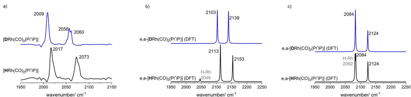
**Fig. 10** a) IR spectroscopic data from H/D-exchange experiment on  $[\text{H}/\text{DRh}(\text{CO})_2(\text{P}^{\text{N}}\text{P})]$  conditions:  $[\text{Rh}] = 1 \text{ mM}$ ,  $[\text{P}^{\text{N}}\text{P}] = 1 \text{ mM}$ ,  $p(\text{CO}) = 1.0 \text{ MPa}$ ,  $p(\text{H}_2/\text{D}_2) = 1.0 \text{ MPa}$  and DFT-based IR-spectra (ESI-†) of the H/D-exchange for b) e,e-complex and c) e,a-coordination of the ligand. Colours: black: hydrido, blue: deuteride complex.
