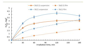
Fig. 4 H<sub>2</sub>O<sub>2</sub> production from Sb(0.5) and Sb(1) dispersed in solution and in the film (1.5% of catalyst).
