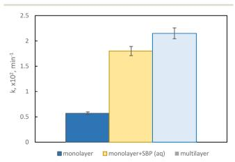
Fig. 5 Kinetic constants obtained from DCP using different photocatalytic films in three different conditions: the catalyst in a monolayer, coupled with peroxidase enzyme in solution and in multilayer films.
