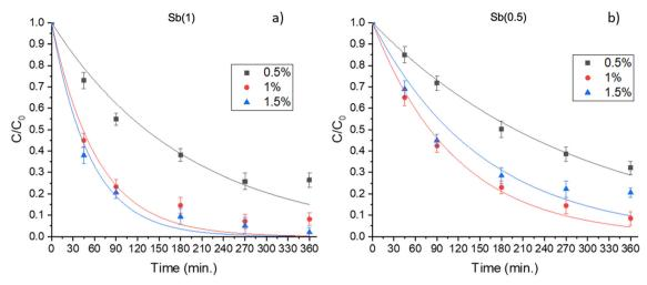
Fig. 3 2,4-Dichlorophenol degradation using films containing different photocatalysts: a) Sb(1) P-doped C<sub>3</sub>N<sub>4</sub> (Sb(1)) and b) Sb(0.5) P-doped C<sub>3</sub>N<sub>4</sub> (Sb(0.5)).
