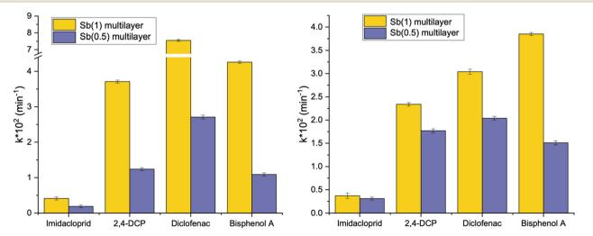
Pseudo-first order kinetic constants derived by degradation curves of the pollutant's mixture in Milli-Q water (left) and aquaculture water Fia. 6 (right).
