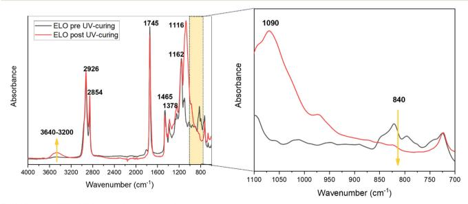
Fig. 2 Real-time FTIR of ELO pre- and post-photocuring
