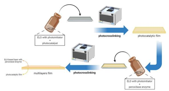
Fig. 1 ELO film preparation procedure
