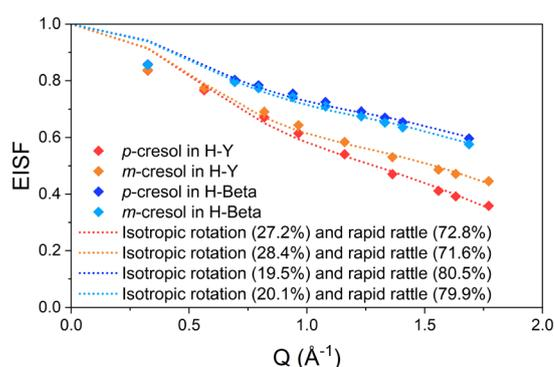
**Fig. 5** Simulated EISFs of *p*- and *m*-cresol in H-Y and H-beta at 370 K, fit by combined models of isotropic rotation and rapid rattling. Percentages of molecules undergoing each mode of motion are shown in brackets.
