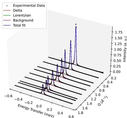
Fig. 1 QENS spectra across the measured  $Q$  range of  $p$ -cresol in H-Y at 370 K.
