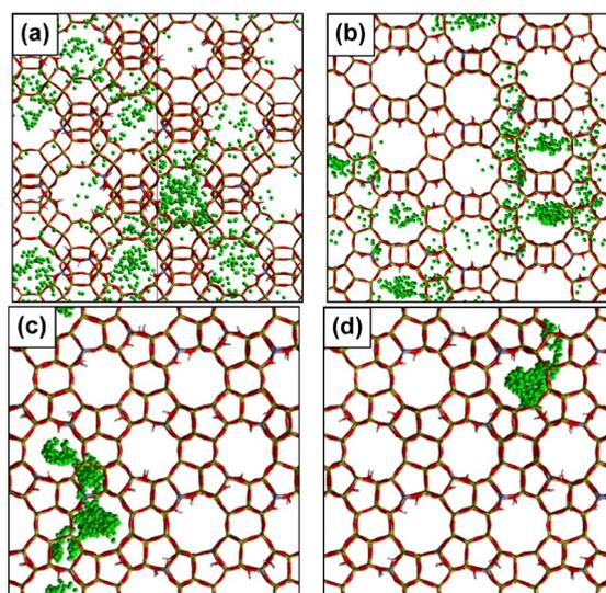
**Fig. 11** Trajectories of a cresol molecule printed every 5 ps up to 5 ns (tracking a ring carbon atom), for (a) *p*-cresol in H-Y, (b) *p*-cresol in H-beta, (c) *p*-cresol and (d) *m*-cresol in H-ZSM5 at 653 K.
