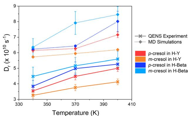
**Fig. 4** Rotational diffusion coefficients of *p*- and *m*-cresol in H-Y and H-beta from 340–400 K, calculated from the QENS experiment and MD simulations.
