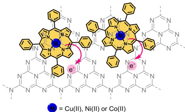
Fig. 33 Representation of the hybrid structures of Cu3-, Ni3-, and Co3-g-C<sub>3</sub>N<sub>4</sub>.
