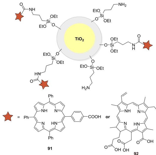
Fig. 40 Representation of the TiO<sub>2</sub>-APTES-PS NPs.
