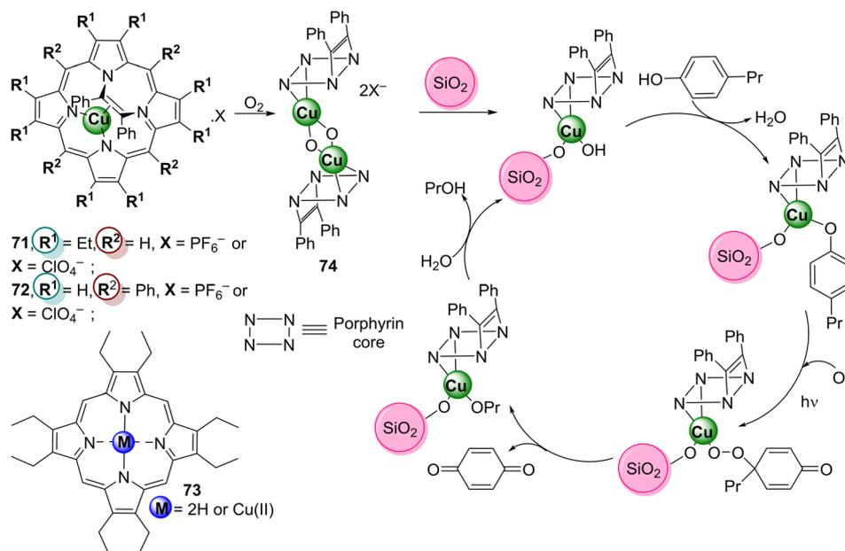
Fig. 25 Copper(I) complexes of the  $N^{21},N^{22}$ -etheno bridged porphyrins **71** and **72**, and the proposed mechanism of the photodegradation of 4-propylphenol catalysed by these complexes immobilized on silica gel.
