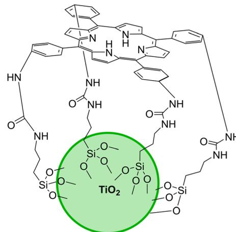
Fig. 22 Representation of the porphyrin-based hybrid silica-titania photocatalyst 67.
