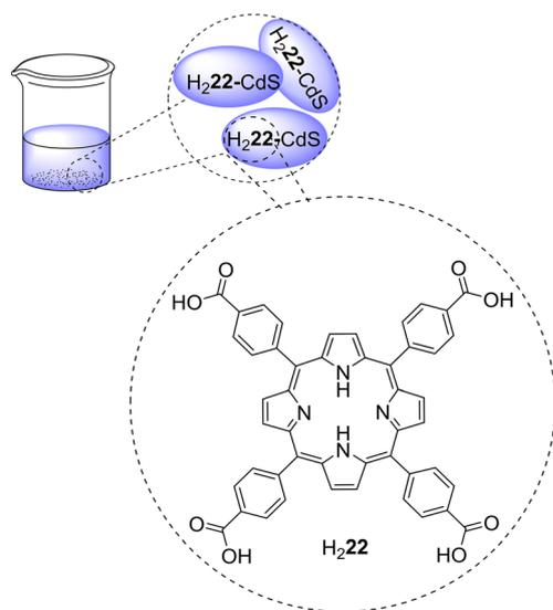
Fig. 30 Representation of CdS nanocomposites modified with H<sub>2</sub>22 for the photodegradation of dyes.
