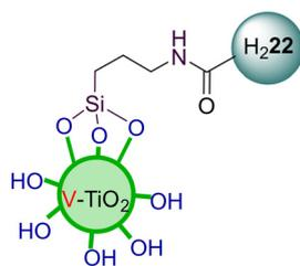
Fig. 37 Representation of vanadium doped TiO<sub>2</sub> modified with H<sub>2</sub>22 using a 3-aminopropylsilane bridging unit.
