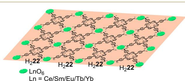
Fig. 10 Representation of Ln-H<sub>2</sub>22 MOF nanosheets.
