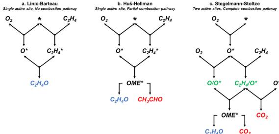
Fig. 1 Simplified representations of the (a) Linic-Barteau, (b) Huš-Hellman, and (c) Stegelmann-Stoltze reaction networks. indicates empty metallic site. X\* indicating an adsorbed species. OME denotes the oxametallacycle intermediate. O\* indicates a species adsorbed on an oxide site.
