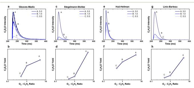
Fig. 4 (a and b) Experimental and (c-h) simulated ethylene oxide responses and yields for pump-probe experiments with varied oxygen to ethylene ratios at 523 K. The experimental results showed increased ethylene oxide production with increasing oxygen to ethylene ratio<sup>15</sup> with the simulated results showing similar general trends, but the HH model is the only one to have a concave type relationship with increasing O2: C2H4 ratio. Experimental data was adapted from ref. 15.
