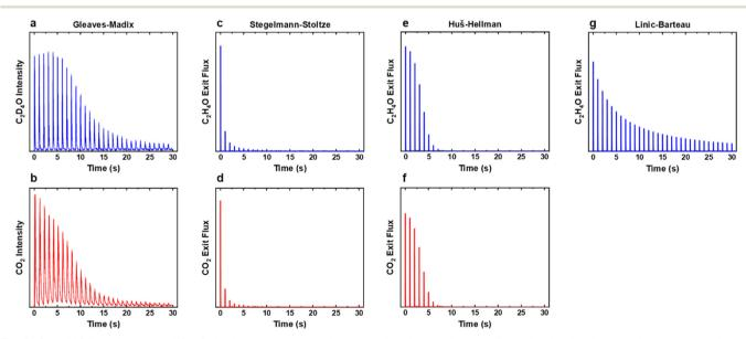
Fig. 6 (a and b) Experimental and (c-g) simulated ethylene oxide and combustion product exit fluxes for the titration experiment where ethylene was pulsed over the oxidised silver surface at 547 K. The HH model was run with 60% decreased surface area as the conversion of ethylene was 100% during the unmodified experiment. None of the models were found to recreate the experimentally observed trends. Experimental data was adapted from ref. 15.
