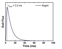
Fig. 2 Simulated pulse of Ar through the TAP microreactor with the time of maximum intensity overlayed. The maximum intensity matches that reported experimentally of 3.5 ms. <sup>15</sup>
