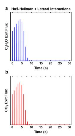
Fig. 7 Simulated (a) ethylene oxide and (b) CO2 exit flux for the multi-pulse titration experiment over oxidised silver using the HH model with lateral interactions included. All other parameters were kept consistent with the original experiment. Peak ethylene oxide production was observed in pulse 5, with a rapid decrease in production observed afterwards. The same trend was observed in the CO2 (acetaldehyde) flux.
