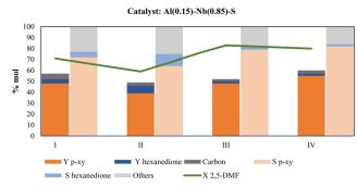
Fig. 9 Catalyst performance with respect to treatment applied before the re-use in terms of yield and selectivity to p-xylene and hexanedione, 2,5-DMF conversion, and carbon % (deposited on used catalyst). Fresh catalyst (column I), catalyst without treatment (column II), after washing with 1,4-dioxane (column III), and after calcination (column IV). Reaction conditions: 250 °C, 30 bar of ethylene, 0.15 g of catalyst, 0.15 g of 2,5-DMF and magnetic stirring of 1000 rpm.
