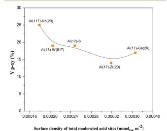
Fig. 3 Yield to p-xylene  $(Y_{p-xy})$  as a function of the surface density of total moderate acid sites (number of moderate Br and Le acid sites per surface of solid).
