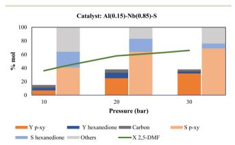
Fig. 8 Influence of ethylene pressure on the catalytic activity in terms of yield and selectivity to p-xylene and hexanedione, 2,5-DMF conversion and carbon % (deposited on used catalyst). Reaction conditions: 250 °C, 0.15 g of catalyst, 0.3 g of 2,5-DMF, 1,4-dioxane as solvent, 5 h of reaction time and magnetic stirring at 1000 rpm.
