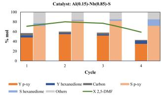
Fig. 10 Catalyst performance with consecutive reuses in terms of yield and selectivity of p-xylene and hexanedione, 2,5-DMF conversion and carbon % (deposited on used catalyst). Reaction conditions: 250 °C, 30 bar of ethylene, 0.15 g of catalyst, 0.15 g of 2,5-DMF and magnetic stirring of 1000 rpm.
