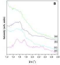
Fig. 1 Low angle XRD patterns of A) SBA-15 (a),  $Ga(\infty)$ -S (b), Nb(77)-S (c), W(1020)-S (d), Zr(28)-S (e), Al(17)-S (f), and B) Al(17)-Ga(26)-S (a), Al(117)-Nb(20)-S (b), Al(18)-W(817)-S (c), Al(17)-Zr(20)-S (d).
