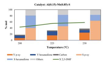
Fig. 7 Influence of temperature on the catalytic activity in terms of yield and selectivity to *p*-xylene and hexanedione, 2,5-DMF conversion and carbon % (measured by EA on the recovered catalyst after reaction). Reaction conditions: 20 bar of ethylene, 0.15 g of catalyst, 0.3 g of 2,5-DMF, 1,4-dioxane as solvent, 5 h of reaction time and magnetic stirring at 1000 rpm.
