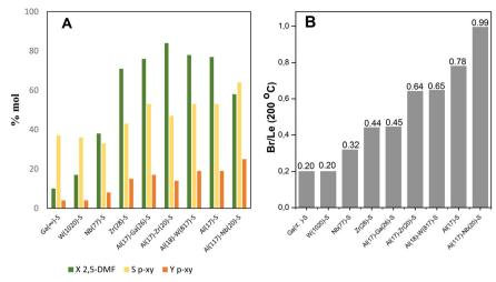
Fig. 2 A) Catalytic activity in terms of 2,5-DMF conversion  $(X_{2,5-\mathrm{DMF}})$ , p-xylene selectivity  $(S_{p-xy})$  and p-xylene yield  $(Y_{p-xy})$ , for the different catalysts. B) Br/Le ratio of sites with moderate strength (from IR data with pyridine desorption at 200 °C) measured for each catalyst. Data ordered in function of increasing Br/Le ratio.
