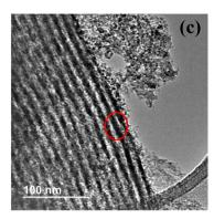
Fig. 4 TEM images of the Al(117)-Nb(20)-S ordered mesoporous material obtained with different magnification: at 100 nm (a) and 200 nm (b) scales, and pore diameter visualization (c).
