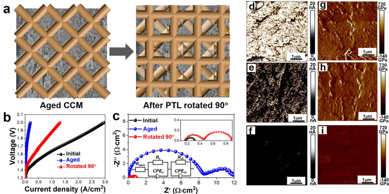
Fig. 2 (a) Schematic diagram of the Ti mesh rotated 90 degrees before and after the aging test. (b) Polarization curve of the RuO<sub>2</sub> catalyst before and after the aging test at 1.8 V. (c) Impedance spectra before and after the aging test at 1.8 V. AFM measured for CL before (d and g) and after aging in zone (1) (e and h) and zone (2) (f and i). (d, e, and f) Conductivity of CL by the AFM test. (g, h, and i) stiffness of CL by the AFM test.
