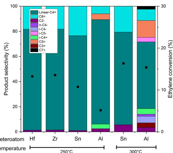
Fig. 5 Product selectivity (bars) and ethylene conversion (black squares) obtained from ethylene oligomerization over Ni/M-Beta catalysts. Reference reaction conditions: 30 bar total pressure,  $P_{\text{ethylene}} = 10 \text{ bar}$  and contact time of  $0.017 \text{ min g}_{\text{cat}}^{-1} \text{ mL}^{-1}$ .
