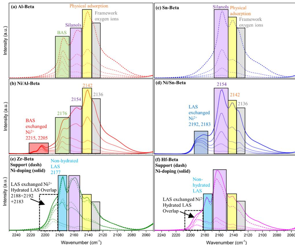
**Fig. 3** FTIR spectra within the CO vibration region upon desorption over Si/M-Beta catalysts. (a) and (b): Al-Beta without and after nickel loading; (c) and (d): Sn-Beta without and after nickel loading. The boxes filled with color represent different species upon CO adsorption. Spectra of Zr-Beta and Hf-Beta are shown in (e) and (f), with the overlay plots to show the shift.
