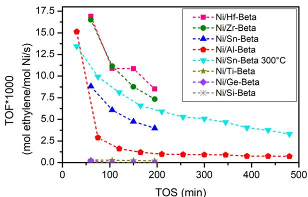
Fig. 4 Rate of ethylene conversion *versus* time on stream for all catalysts. Reference reaction conditions: 30 bar total pressure,  $P_{\text{ethylene}} = 10 \text{ bar}$ ,  $T = 250 \text{ °C}$  and contact time of  $0.017 \text{ min g}_{\text{cat}}^{-1} \text{ mL}^{-1}$ . An additional experiment is presented using Ni/Sn-Beta at 300 °C.
