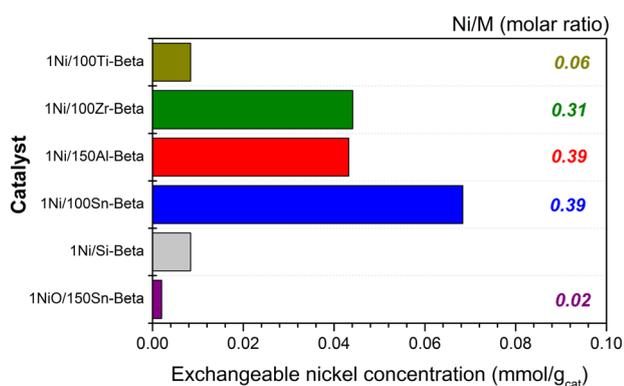
Fig. 2 Nickel-ion exchange capacities of different catalysts, measured from NH<sub>4</sub><sup>+</sup> reverse ion exchange. Ni/M ratios represent the molar fraction of nickel-exchanged species by the total metal content.
