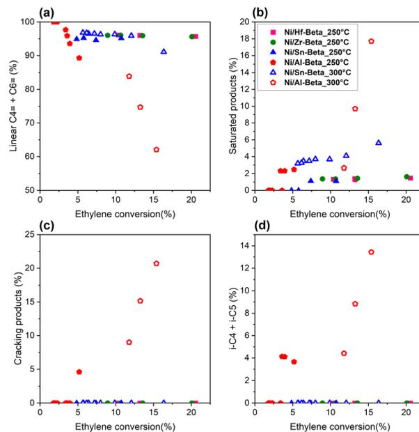
**Fig. 6** Selectivity towards (a) linear butenes and hexenes, (b) saturated products, (c) cracking products and (d) isomerization products over Ni/M-Beta catalysts during ethylene oligomerization. Reference reaction conditions: 30 bar total pressure,  $P_{\text{ethylene}} = 10$  bar and contact time of  $0.017 \text{ min g}_{\text{cat}}^{-1} \text{ mL}^{-1}$ .
