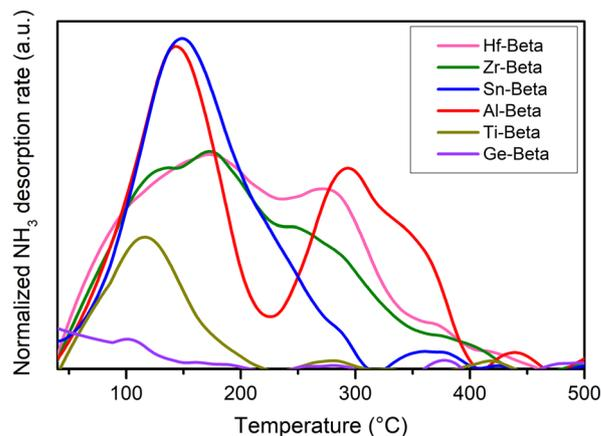
Fig. 1  $NH_3$ -TPD/TGA profiles for M-Beta zeolitic materials.
