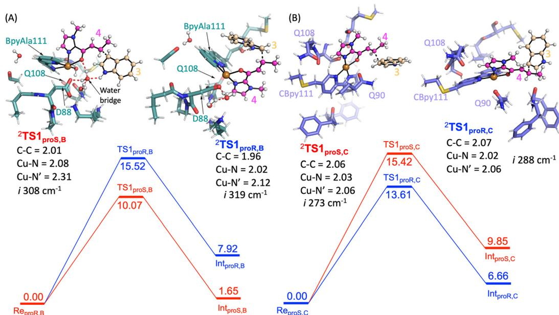
**Fig. 5** Potential energy landscape for the Friedel–Crafts alkylation by A) SCP\_Q111BpyAla and B) SCP\_Q111CBpy. Energy values are in kcal mol<sup>-1</sup>. The optimized geometric structures of the transitions are shown on the left and right of free energy landscape with their important bond lengths in Å. The imaginary frequency represents the stretching vibration of C–C bonds between 3 and 4 for each transition state.
