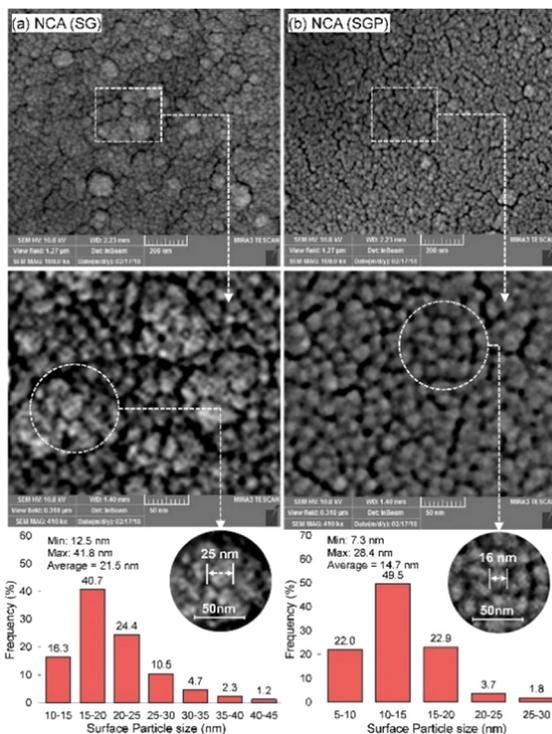
**Fig. 15** The surface particle size histogram of Co-promoted Ni-spinel nano-catalysts fabricated via sol-gel and hybrid sol-gel-plasma methods: (a) NCA (SG refers to catalysts from the sol-gel method) and (b) NCA (SGP refers to catalysts from sol-gel-plasma methods). Reproduced from ref. 163 with permission from Chemical Engineering journal, copyright 2019.
