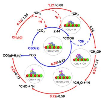
**Fig. 3** Schematic diagram of methane dry reforming reaction. The corresponding activation energy is  $E_a$  (red) and reaction energy (black) is in the unit of eV for each step. Reproduced from ref. 45 with permission from Nature Communications, copyright 2023.
