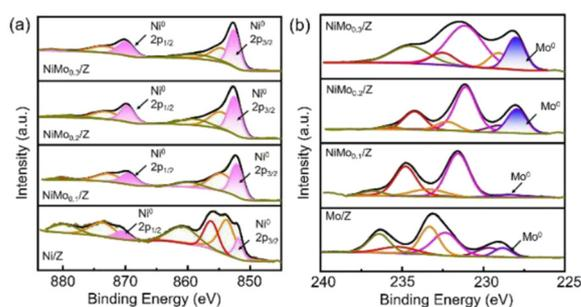
**Fig. 9** The *ex situ* spectra (a) Ni<sup>0</sup> 2p and (b) Mo<sup>0</sup> 3d XPS spectra of the reduced catalysts. Reproduced from ref. 125 with permission from American Chemical Society Catalysis, copyright 2021.
