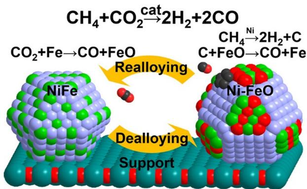
**Fig. 11** De-alloying and re-alloying behaviour of a Fe-Ni-alloyed particle during the dry reforming of methane. Reproduced from ref. 130 with permission from Journal of American Chemical Society, copyright 2017.
