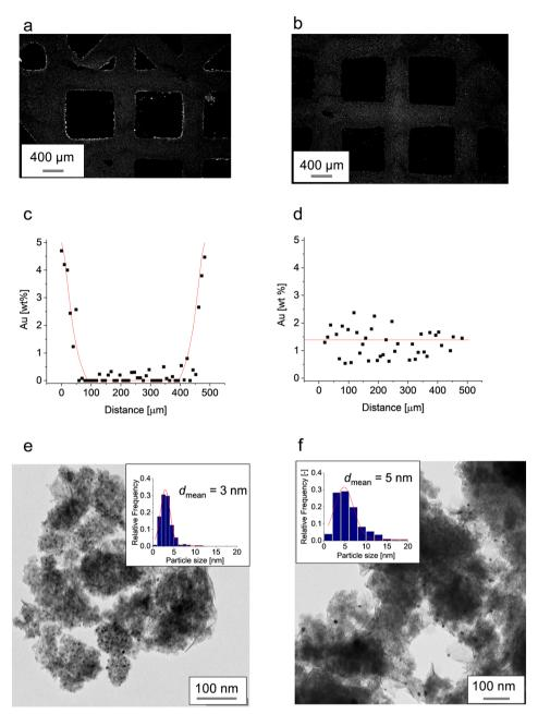
Fig. 5 Internal SEM micrographs of the 3D printed  $Au/Al_2O_3$  catalyst prepared with a) DPU and b) DP method. EDX scans of the catalyst prepared with c) DPU and d) DP method. TEM micrographs and gold nanoparticle size distribution obtained with e) DPU and f) DP methods.
