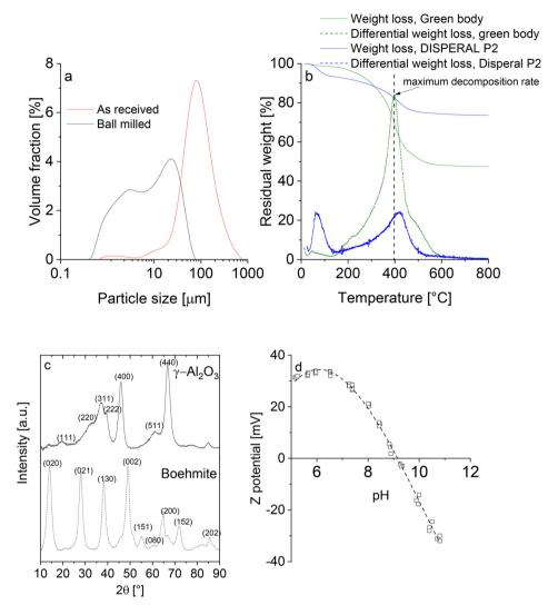
Fig. 2 a) Particle size distribution of boehmite b) thermogram of pure boehmite and the green body c) XRD profiles of boehmite and γ-Al<sub>2</sub>O<sub>3</sub> d) zeta-potential as a function of pH for  $\gamma$ -Al<sub>2</sub>O<sub>3</sub>.
