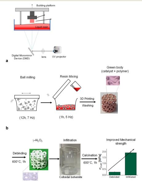
Fig. 1 a) Schematic representation of a DLP printer b) schematization of the printing policy
