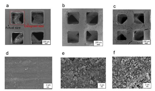
Fig. 4 SEM micrographs of the 3D printed green body (a and d), debinded (b and e) and infiltrated (c and f)  $\gamma$ -Al<sub>2</sub>O<sub>3</sub> support.
