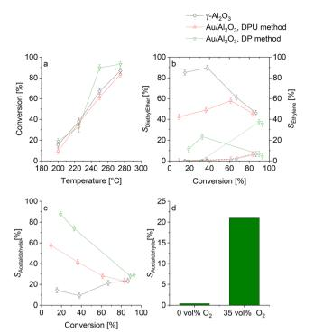
Fig. 6 Oxidative dehydrogenation of ethanol at atmospheric pressure, ethanol-to-oxygen ratio of 2 and flow rate of 100 mL min<sup>-1</sup>. a) Ethanol conversion as a function of temperature b) selectivity towards the dehydration products vs. ethanol conversion (solid line is diethyl ether, dashed line is ethylene) c) selectivity to acetaldehyde vs. conversion d) selectivity to acetaldehyde in the presence and absence of O2 on  $\gamma$ -Al<sub>2</sub>O<sub>3</sub>.
