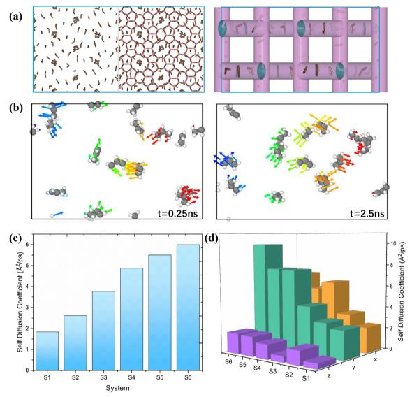
Fig. 2 (a) Snapshot of MD trajectory and (b) motion of propylene molecules in MFI at 553 K; (c) self-diffusion coefficient of propylene and (d) selfdiffusion coefficient of propylene distributed in the x, y and z directions.
