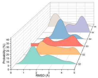
Fig. 3 The RMSD of propylene molecule inside MFI zeolite.
