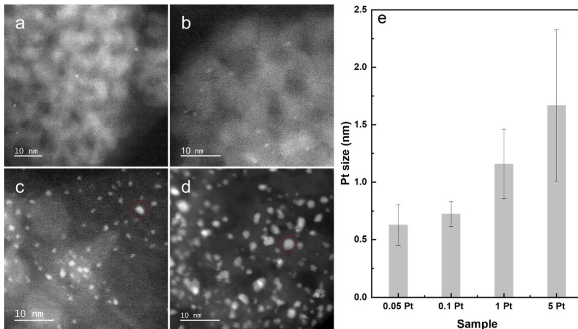
Fig. 2 HAADF-STEM images of 0.05Pt (a), 0.1Pt (b), 1Pt (c) and 5Pt (d) samples after  $\text{H}_2$  activation at 400 °C for one hour and the Pt size distribution determined using these images (e) with the error bar representing the standard deviation of the size measurement. Note that the red circles in (c) and (d) exhibit the well-defined Pt crystal lattice.
