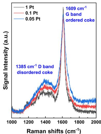
Fig. 9 Raman spectra of spent Pt/Al<sub>2</sub>O<sub>3</sub> samples aiming to determine the coke species deposited on these samples during the 20 h stability tests. The laser excitation wavelength is 244 nm.
