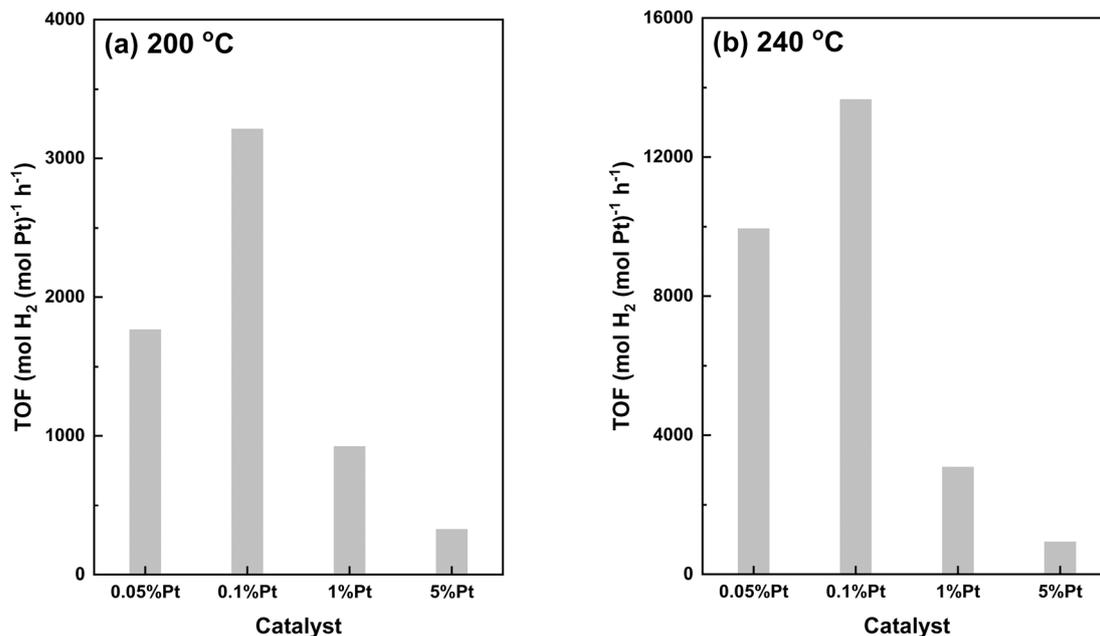
Fig. 5 TOF of Pt over Pt/Al<sub>2</sub>O<sub>3</sub> catalysts at 200 °C (a) and 240 °C (b) in MCH dehydrogenation.
