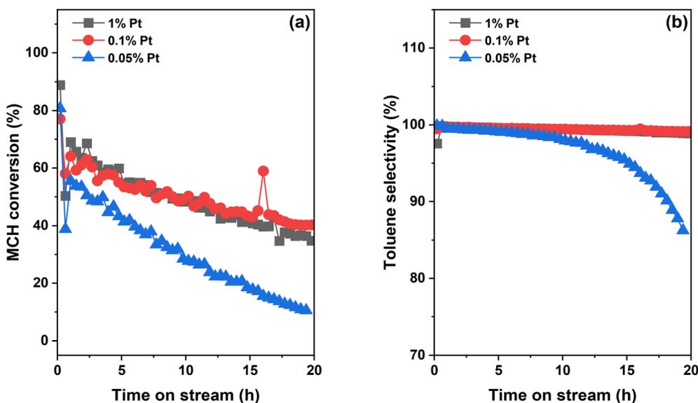
Fig. 6 MCH conversion (a) and toluene selectivity (b) over Pt/Al<sub>2</sub>O<sub>3</sub> catalysts during 20 h MCH dehydrogenation tests at 320 °C. Amounts of catalysts used for the reaction: 30 mg 0.1Pt sample, 60 mg 0.05Pt sample, and 3 mg 1Pt sample mixed with 27 mg quartz sand. Reaction conditions: 6.5 mL min<sup>-1</sup> Ar and 0.006 mL min<sup>-1</sup> MCH injected using a syringe pump.
