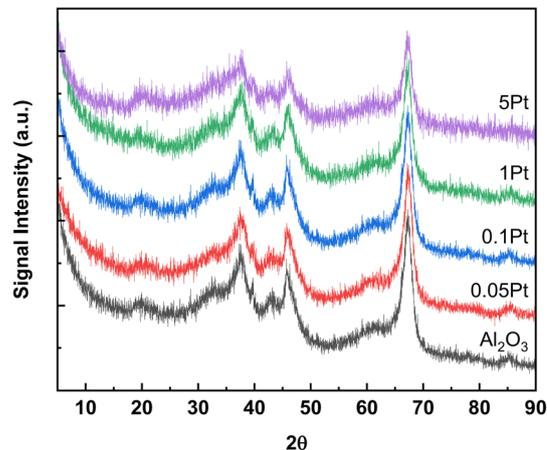
**Fig. 1** XRD patterns of as-calcined Pt/Al<sub>2</sub>O<sub>3</sub> samples.
