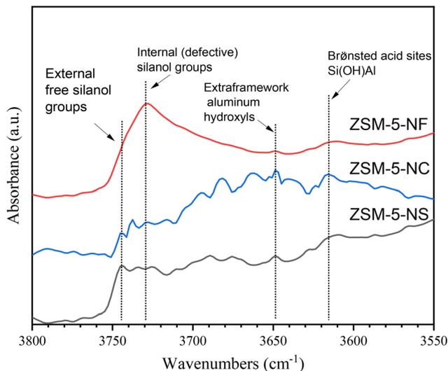
**Fig. 6** FTIR spectra in the OH-stretch region (3800–3550 cm<sup>-1</sup>) of the samples with different morphologies.
