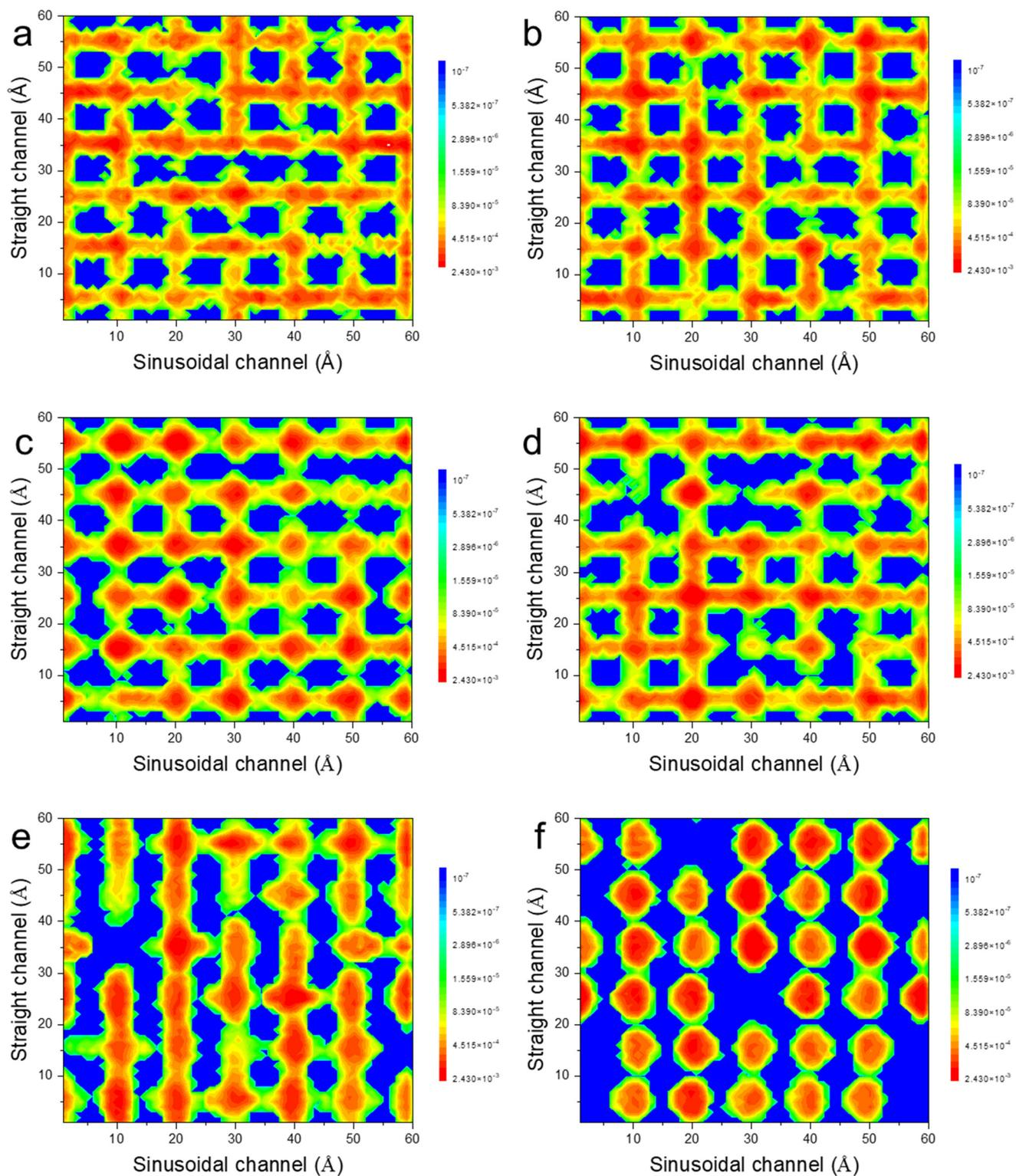
Fig. 9 Contour lines for the diffusion of (a) methanol, (b) ethene, (c) propylene, (d) *n*-butene, (e) *p*-xylene, and (f) *o*-xylene molecules in the straight and sinusoidal channels of H-ZSM-5 zeolite at 743 K.
