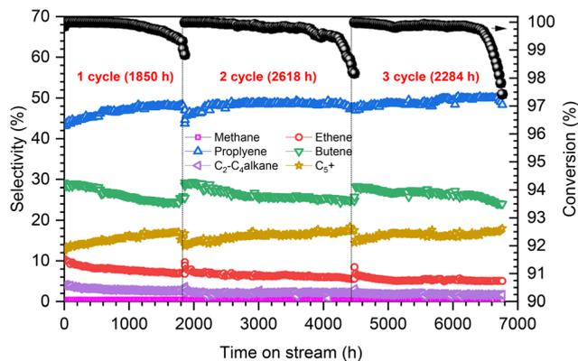
Fig. 11 Methanol conversion of methanol as a function of time on stream over shaped ZSM-5-NS. Reaction conditions:  $T = 460\text{--}480\text{ }^{\circ}\text{C}$ ,  $\text{WHSV} = 1.25\text{ h}^{-1}$ , catalyst weight = 80 g.
