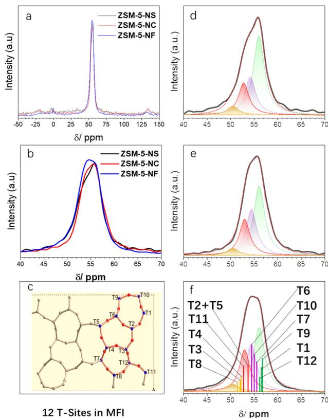
**Fig. 10**  $^{27}\text{Al}$  MAS NMR spectra of ZSM-5 with different morphologies, (a) low magnification, (b) high magnification, and (c) crystallographically distinct 12 T-sites in the MFI structure,<sup>44</sup> (d) peak fitting of ZSM-5-NS, (e) peak fitting of ZSM-5-NC, and (f) peak fitting of ZSM-5-NF.
