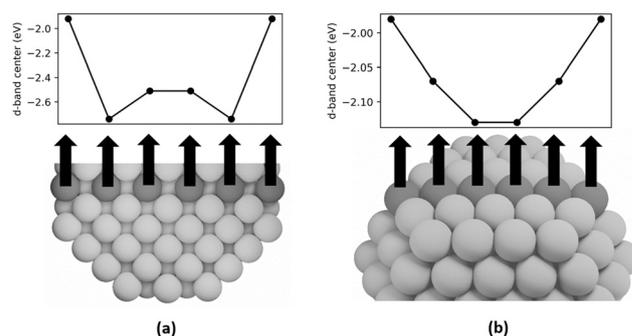
Fig. 8 a) Plot of d-band center for each shaded atom along the cross-section of the Pt-314 nanoparticle. The first and last atoms are present on the terraces (CN = 9), and the remaining atoms are present in the bulk (CN = 12). b) Plot of d-band center for each shaded atom on the terrace of the Pt-314 nanoparticle. The first and last atoms correspond to undercoordinated steps (CN = 7) and the remaining atoms correspond to terrace atoms (CN = 9).
