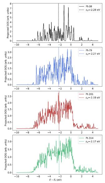
Fig. 9 Smoothed projected density of states (pDOS) of Pt atoms in nanoparticles of different sizes. The pDOS is normalized by the number of atoms
