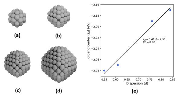
Fig. 6 Schematics of octahedral nanoparticle clusters in the order of decreasing dispersion (a) Pt-38, (b) Pt-79, (c) Pt-201, (d) Pt-314. (e) Plot of d-band centers of the nanoparticle clusters against dispersion. A linear fit is also shown along with the slope (0.41), intercept (-2.51 eV), and coefficient of determination ( $R^2 = 0.98$ ).
