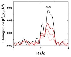
Fig. 2 Pt L<sub>III</sub> EXAFS for samples with Pt nanoparticles of different sizes. Pt foil (black), large sample (dark red), medium sample (moderate red), and small sample (light red).
