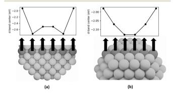
Fig. 8 a) Plot of d-band center for each shaded atom along the crosssection of the Pt-314 nanoparticle. The first and last atoms are present on the terraces (CN = 9), and the remaining atoms are present in the bulk (CN = 12), b) Plot of d-band center for each shaded atom on the terrace of the Pt-314 nanoparticle. The first and last atoms correspond to undercoordinated steps (CN = 7) and the remaining atoms correspond to terrace atoms (CN = 9).
