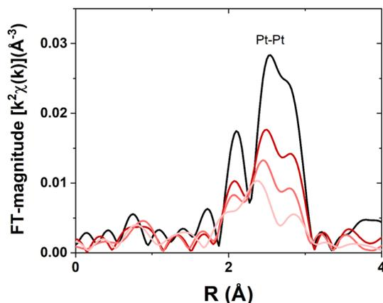
**Fig. 2** Pt L<sub>III</sub> EXAFS for samples with Pt nanoparticles of different sizes. Pt foil (black), large sample (dark red), medium sample (moderate red), and small sample (light red).
