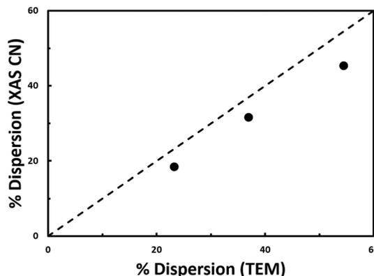
**Fig. 3** Dispersion determined from coordination number from EXAFS fitting versus dispersion determined from STEM. Results from the nanoparticle materials from this study (black circles) are plotted alongside the empirical relationship from literature (dashed black line).<sup>10</sup>
