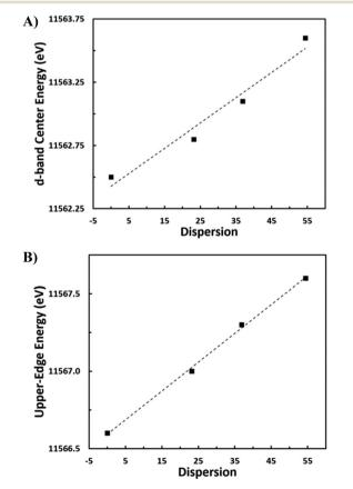
Fig. 7 A) d-Band center energy versus nanoparticle dispersion. B) Upper-edge energy versus nanoparticle dispersion.
