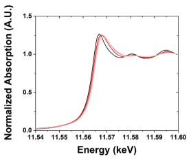
Fig. 4 Pt L<sub>III</sub> XANES for samples with Pt nanoparticles of different sizes. Pt foil (black), large sample (dark red), medium sample (moderate red), and small sample (light red).
