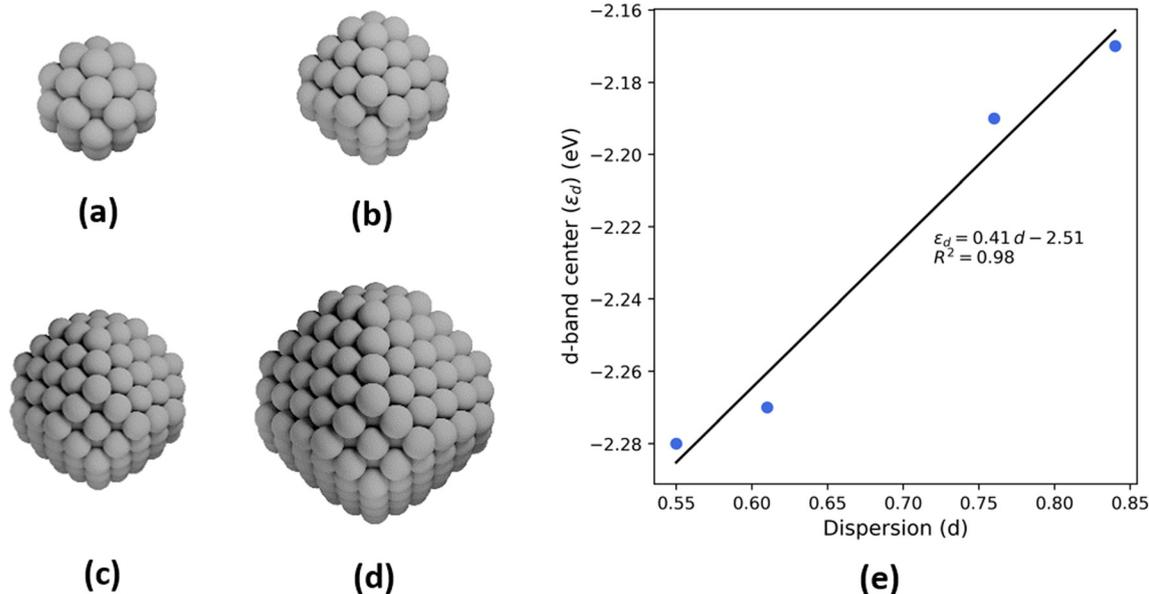
**Fig. 6** Schematics of octahedral nanoparticle clusters in the order of decreasing dispersion (a) Pt-38, (b) Pt-79, (c) Pt-201, (d) Pt-314. (e) Plot of d-band centers of the nanoparticle clusters against dispersion. A linear fit is also shown along with the slope (0.41), intercept (-2.51 eV), and coefficient of determination ( $R^2 = 0.98$ ).
