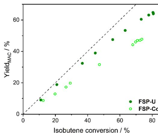
Fig. 8 Methacrolein yield over isobutene conversion for FSP-Co (light) and FSP-U (dark) measured during selective isobutene oxidation. Dotted line indicates the progress of the stoichiometric reaction.
