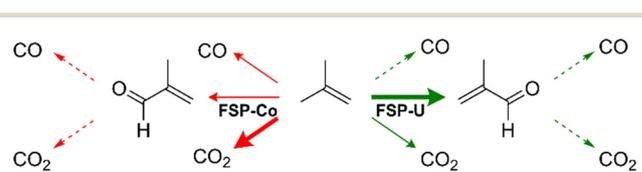
**Fig. 10** Schematic illustration of the reaction network for selective isobutene oxidation over FSP-Co and FSP-U. Bold arrows indicate the most favoured reaction pathway and dashed arrows the least favoured. The arrows depict the general pathways but do not imply more detailed mechanistic information.
