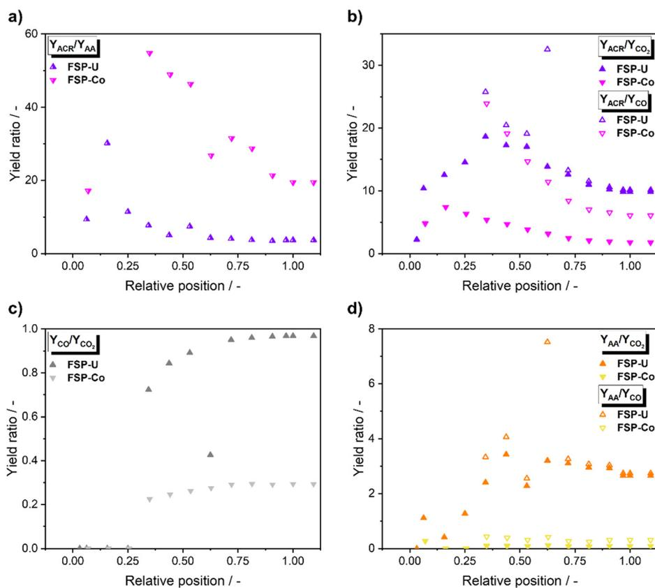
Fig. 3 Yield ratios of acrolein/acrylic acid (a), acrolein/CO<sub>x</sub> (b), CO/CO<sub>2</sub> (c) and acrylic acid/CO<sub>x</sub> (d) of FSP-Co (light) and FSP-U (dark) along the catalyst bed during selective propylene oxidation.
