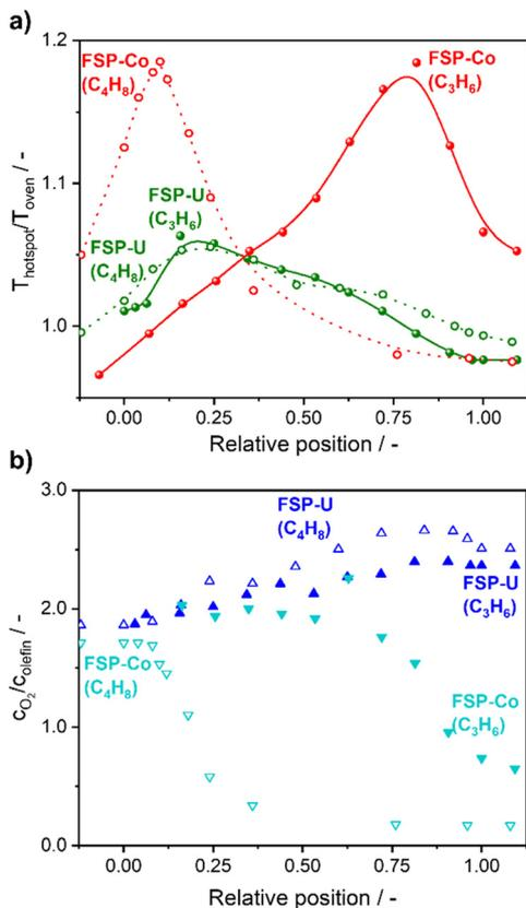
**Fig. 11** Ratios of  $T_{\text{hotspot}}/T_{\text{oven}}$  (a) and oxygen/olefin concentration (b) along the catalyst bed of FSP-U and FSP-Co during selective propylene (filled) or isobutene (empty) oxidation.
