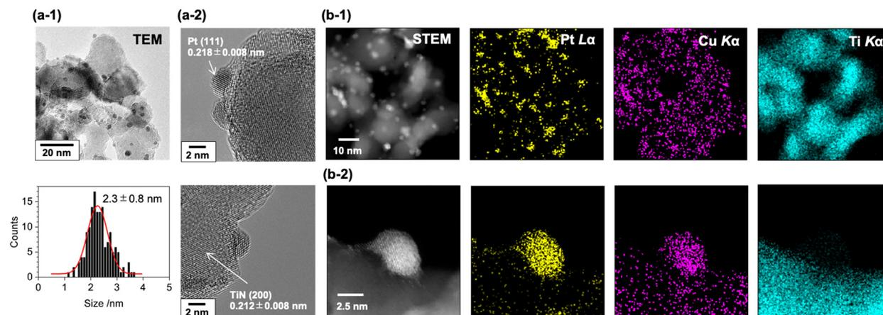
**Fig. 2** (a-1) TEM image with particle size distribution and (a-2) highly magnified TEM images of the PtCu-1.0/TiN catalyst. The averaged particle size was estimated by the Gaussian curve fitting of the particle size distribution (red line). (b) STEM-EDS mappings for Pt L $\alpha$ , Cu K $\alpha$ , and Ti K $\alpha$  of the PtCu-1.0/TiN catalyst with (1) low and (2) high magnifications.
