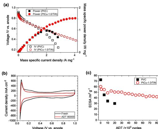
**Fig. 6** (a) IV profiles for PtCu-1.0/TiN (○) and Pt/C (□) and mass specific power plots for PtCu-1.0/TiN (●) and Pt/C (■). (b) CV profiles of the MEA with PtCu-1.0/TiN before (after initial conditioning) and after 80 000 cycles of the accelerated degradation test (ADT). (c) ECSA variation against the number of the ADT cycles for PtCu-1.0/TiN and Pt/C (TEC10E50E, TKK).
