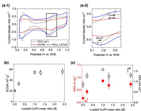
**Fig. 5** (a-1) CV profiles for Pt/TiN (red), PtCu-1.0/TiN (blue), and commercial Pt/C (TKK, TEC10E50E; black dotted line). (a-2) The expanded figure of the black square area in (a-1). (b) Electrochemical surface area (ECSA) and (c) mass specific activity (MSA, red square, left axis) and surface specific activity (SSA, white circle, right axis) for PtCu-*X*/TiN catalysts (*X* = 0–2.4).
