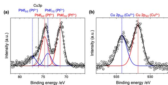
**Fig. 4** (a) Pt 4f and (b) Cu 2p<sub>3/2</sub> XPS spectra with the Gaussian fitting results of the PtCu-1.0/TiN sample.
