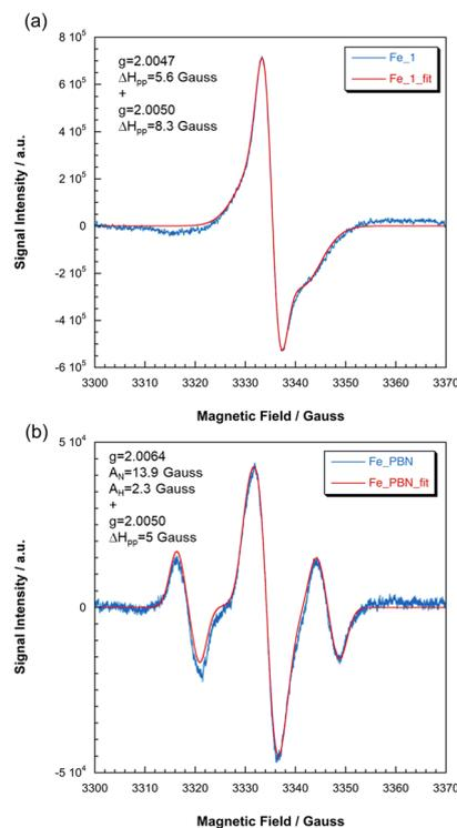
Fig. 3 Experimental (blue line) and least squares fit (red line) EPR spectra of the reaction (**1a** + **3a**  $\rightarrow$  **4aa**) at  $t = 1$  h before (a) and after (b) addition of *N*-tert-butyl- $\alpha$ -phenylnitrene (PBN).
