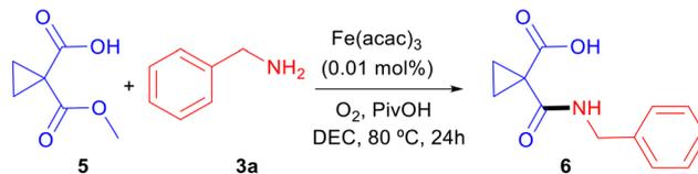
**Scheme 4** Selective amidation of 1-(methoxycarbonyl)cyclopropane-1-carboxylic acid (**5**).
