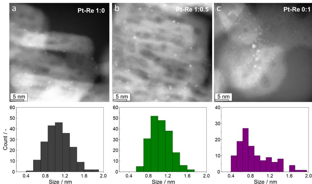
**Fig. 1** High-angle annular dark field scanning transmission electron micrographs of (a) the monometallic Pt-Re 1:0, (b) the bimetallic Pt-Re 1:0.5, and (c) the reference sample Pt-Re 0:1 with histograms of the size distribution. Note, that only clusters >0.4 nm were measured.
