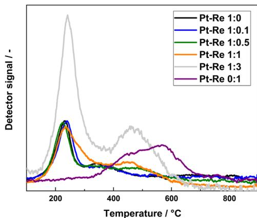
**Fig. 2** Temperature-programmed reduction of as-prepared bimetallic Pt-Re/Al<sub>2</sub>O<sub>3</sub> catalysts and the monometallic references. Analysis parameters: 10% H<sub>2</sub>/Ar, 10 °C min<sup>-1</sup>.
