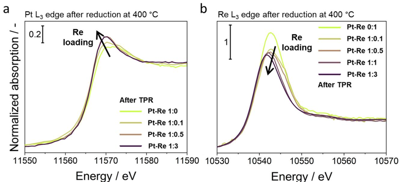
Fig. 4 Comparison of *in situ* X-ray absorption spectra at (a) the Pt and (b) Re  $L_3$  edge after reduction of the bimetallic Pt–Re catalysts with various ratios at 400 °C for 30 min with  $10\text{ °C min}^{-1}$  in 11%  $H_2/He$ . Spectra were acquired after cool-down to room temperature in 11%  $H_2/He$ .
