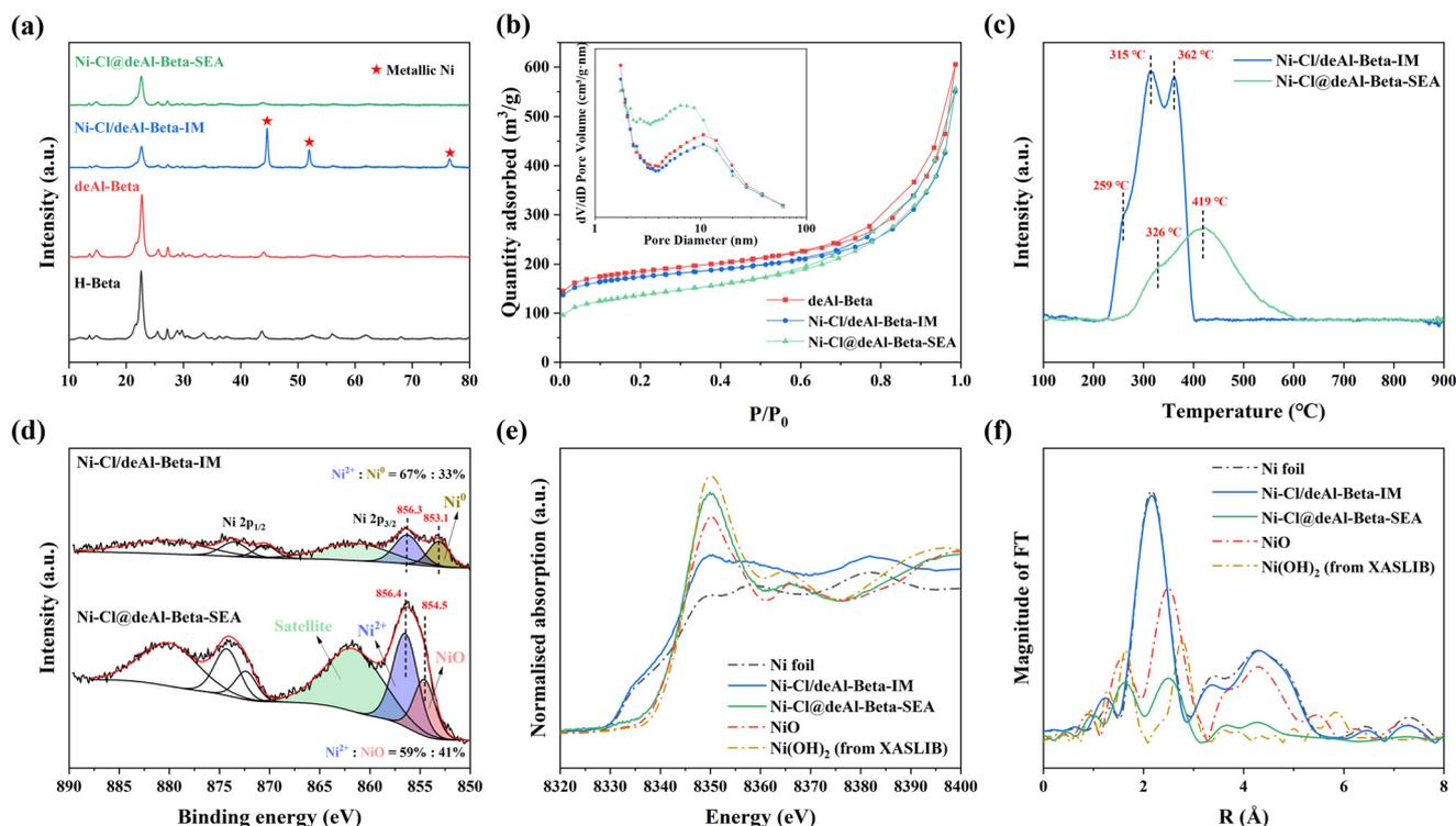
**Fig. 2** (a) XRD patterns and (b) N<sub>2</sub> physisorption isotherms of the beta zeolite supports and the associated Ni catalysts; (c) H<sub>2</sub>-TPR (of the as-prepared Ni catalysts after drying at 120 °C for 4 h), (d) XPS profiles, (e) XANES and (f) Fourier transform of  $k^3$ -weighted EXAFS spectra of the reduced Ni-Cl@deAl-beta-SEA and Ni-Cl/deAl-beta-IM. Note that the data of Ni(OH)<sub>2</sub> is referred to the XASLIB database.
