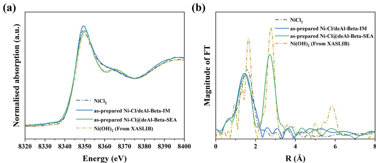
Fig. 3 Ni K-edge XANES analysis (a) of Ni form in as-prepared Ni-Cl/deAl-beta-IM and Ni-Cl@deAl-beta-SEA (after drying at 120 °C for 4 h) and (b) the Fourier transform of  $k^3$ -weighted EXAFS spectra.
