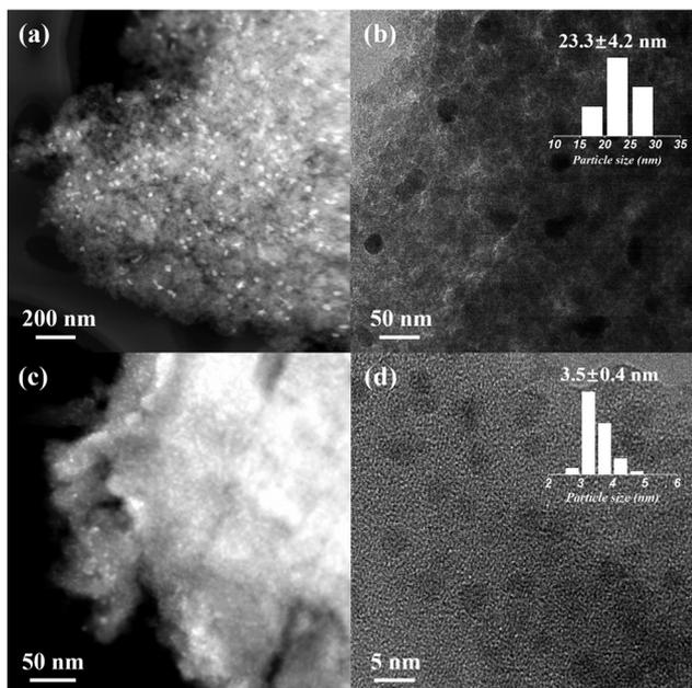
**Fig. 1** HAADF-STEM and HRTEM micrographs of (a and b) Ni-Cl/deAl-beta-IM and (c and d) Ni-Cl@deAl-beta-SEA. The particle size distribution of the studied catalysts was based on statistics of counting ca. 100 particles from relevant HRTEM images (using ImageJ).
