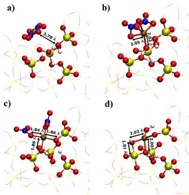
Fig. 6 Optimised geometries of metallic complexes adsorbed on the deAl-beta framework:  $\text{Ni}(\text{NO}_3)_2$  adsorption to the silanol nest at (a) full protonation (IM), (b) first degree of deprotonation, (c) second degree of deprotonation, and (d)  $\text{Ni}(\text{OH})_2$  adsorption at the doubly deprotonated silanol nest.
