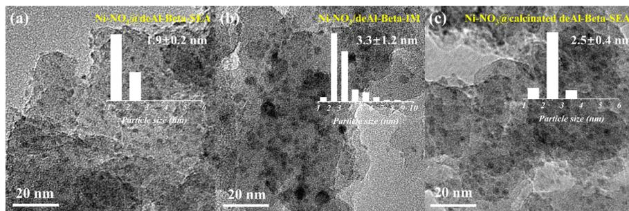
Fig. 5 TEM images of Ni catalysts prepared using  $\text{Ni}(\text{NO}_3)_2$  as the precursor. (a)  $\text{Ni}-\text{NO}_3$ @deAl-beta-SEA, (b)  $\text{Ni}-\text{NO}_3$ @deAl-beta-IM and (c)  $\text{Ni}-\text{NO}_3$ @calcinated deAl-beta-SEA. The particle size distribution of the three catalysts was based on statistics of counting ca. 100 particles from relevant HRTEM images (using ImageJ).
