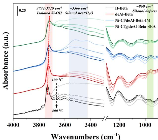
Fig. 4 *In situ* DRIFTS studies on reduction of Ni catalysts prepared by IM and IM with NiCl<sub>2</sub> as precursor.
