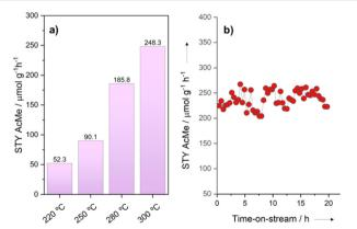
Fig. 4 (a) Catalytic performance as a function of the temperature and (b) catalytic stability test during 20 h at 300 °C for the methanol carbonylation reaction in terms of methyl acetate productivity over the Cu-H-MOR catalyst.
