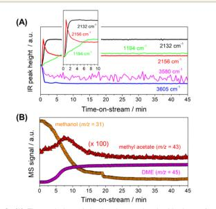
Fig. 8 (A) The evolution of the bands associated with the surface species involved in the reaction and (B) evolution of the reactants and products in the gas phase analyzed online by MS during the reaction.
