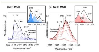
Fig. 3 The FTIR study of adsorption of CO at 77 K over (A) H-MOR and (B) Cu-H-MOR samples.
