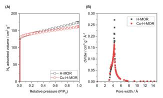
Fig. 2 (A) N<sub>2</sub> adsorption-desorption isotherms at 77 K for mordenite samples and (B) the pore-size distribution.
