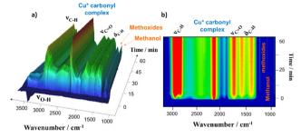
6 (a) The three-dimensional and (b) two-dimensional representations of the bands that appear and disappear as a function of time during the carbonylation reaction at 200 °C and 1 bar in the Cu-H-MOR sample.
