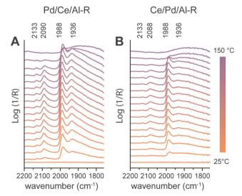
Fig. 6 Operando Diffuse Reflectance Infrared Fourier Transform Spectroscopy (DRIFTS) spectra under CH<sub>4</sub> oxidation reaction conditions, for (A) Pd/Ce/Al-R and (B) Ce/Pd/Al-R catalysts after calcination at 850 °C and in situ reduction at 450 °C in 50 vol%  $H_2/N_2$ . Conditions: CH<sub>4</sub> 1 vol%, O<sub>2</sub> 4 vol/%, N<sub>2</sub> balance, 50 mL min<sup>-1</sup> total flow. R = reduced.
