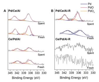
Fig. 5 X-ray photoelectron spectroscopy (XPS) results in the Pd 3d region, with the fitting of Pd 3d peaks.(A) Pd/CeO<sub>x</sub>/γAl<sub>2</sub>O<sub>3</sub> (Pd/Ce/Al); (B)  $CeO_x/Pd/\gamma-Al_2O_3$  (Ce/Pd/Al); R = reduced. Due to significant noise and low intensity in the XPS of Ce/Pd/Al-R and Ce/Pd/Al-R-S catalysts, deconvolution and peak fitting were not performed for these catalysts.
