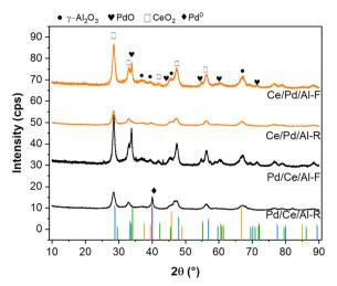
Fig. 4 X-ray diffraction (XRD) patterns of fresh and reduced Pd/CeO<sub>x</sub>/  $\gamma Al_2O_3$  (Pd/Ce/Al) and CeO<sub>x</sub>/Pd/ $\gamma Al_2O_3$  (Ce/Pd/Al) catalysts. F = fresh; R = reduced. Reference patterns:  $\gamma$ -Al<sub>2</sub>O<sub>3</sub> (ICCD 00-004-0858) in yellow, tetragonal PdO (COD 414668) in green, CeO2 (COD 7217887) in blue, Pd (COD 1011105) in purple.
