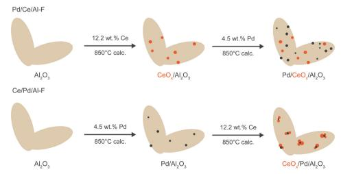
Fig. 1 Schematic showing the impregnation sequence in the as-prepared Pd/CeO<sub>x</sub>/Al<sub>2</sub>O<sub>3</sub> (Pd/Ce/Al-F) and CeO<sub>x</sub>/Pd/Al<sub>2</sub>O<sub>3</sub> (Ce/Pd/Al-F) catalysts
