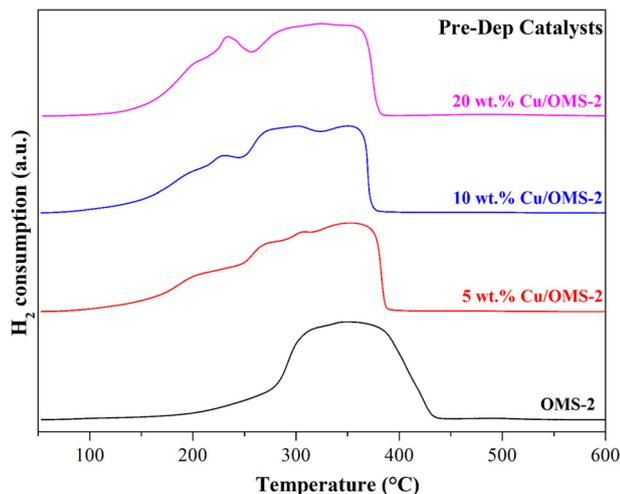
Fig. 3 H<sub>2</sub>-TPR profiles of 5, 10 and 20 wt% Cu/OMS-2 catalysts prepared by the Pre-Dep method.
