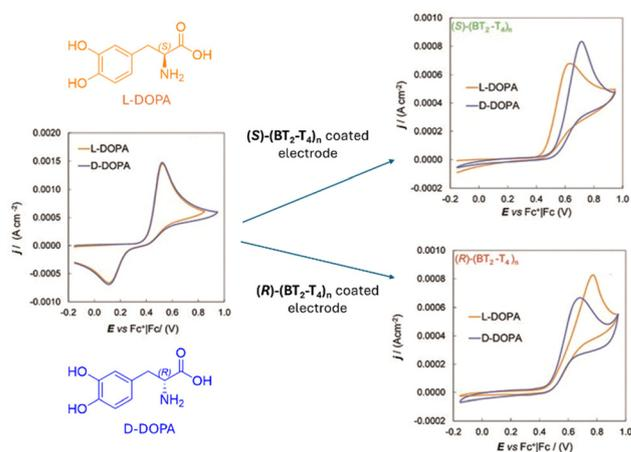
**Fig. 16** Cyclic voltammetry of DOPA enantiomers (4 mM H<sub>2</sub>O + 50 mM HCl) recorded with (left) a bare GC electrode, (right, up) a GC electrode coated with (S)-(BT<sub>2</sub>-T<sub>4</sub>)<sub>n</sub>, and (right, down) a GC electrode coated with (R)-(BT<sub>2</sub>-T<sub>4</sub>)<sub>n</sub>, the enantiomeric pair of bithianaphthene-based oligomers. Reproduced from ref. 79 with permission from The Royal Society of Chemistry, copyright 2010.
