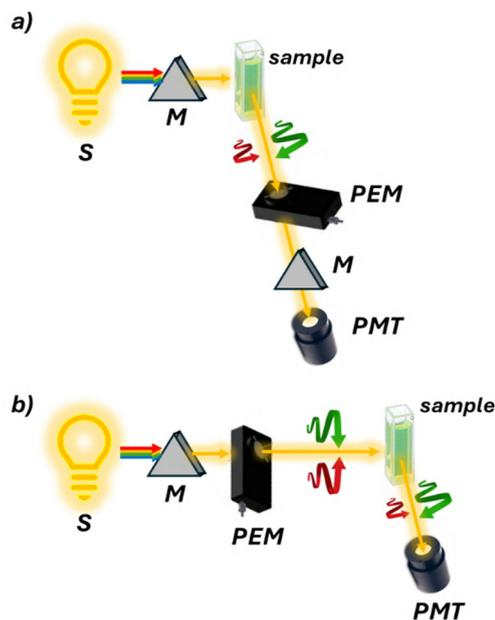
Fig. 8 Schematic representation of (a) a CPL and (b) an FDCCD spectro-polarimeter. FDCCD has the same optical components as CD with the photomultiplier tube (PMT) placed at  $90^\circ$  to collect the fluorescence. CPL instead has the photoelastic modulator (PEM) after the sample to detect the differently emitted right and left circular polarizations.
