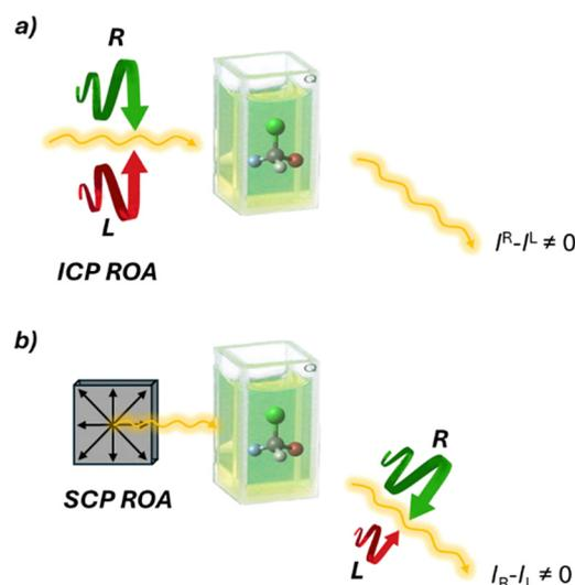
Fig. 10 Schematic representation of the two ROA techniques. (a) ICP ROA measures  $(I^R - I^L)$ , where  $I^R$  and  $I^L$  are the scattered intensities in right- and left-circularly polarized incident light, respectively. (b) SCP ROA measures  $(I_R - I_L)$ , where  $I_R$  and  $I_L$  are the intensities of the right- and left-circularly polarized components, respectively, of the scattered light using incident light of fixed polarization.
