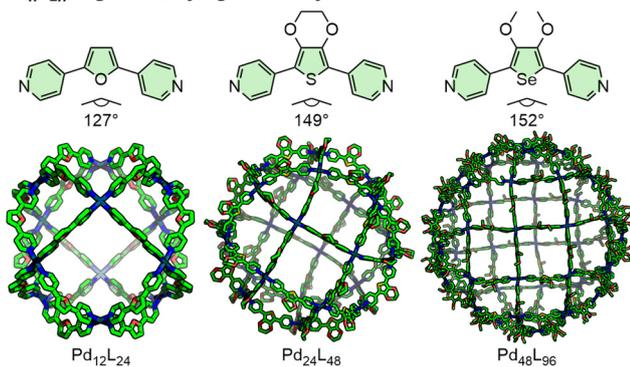
Fig. 2 Different nuclearity Pd<sub>n</sub>L<sub>2n</sub> coordination cages assembled from bis-monodentate ligands and Pd(II) ions ( $n = 12, 24$  and  $48$  from left to right).
