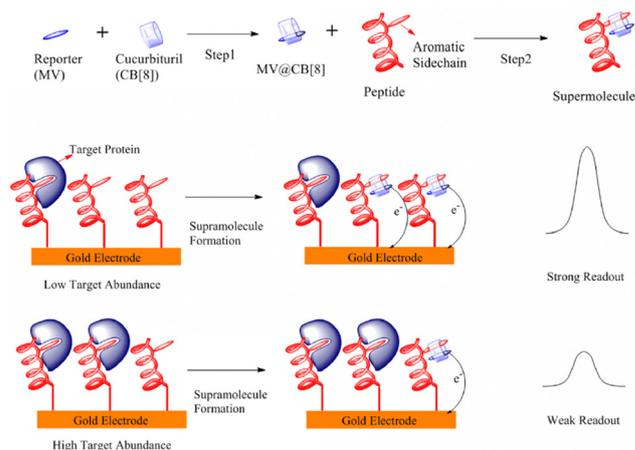
Fig. 22 Protein sensing technique through electrochemical readout at a gold surface. CB[8] is Q8.<sup>109</sup> Reproduced with permission from ref. 109. Copyright 2012 American Chemical Society.
