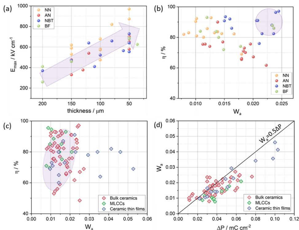
Fig. 19 Impact of thickness on (a)  $E_{\max}$  (b) normalised  $W_a = W_{\text{rec}}/E_{\max}$  and  $\eta$  in NN, AN, NBT, and BF-based ceramics (c) normalised  $W_a$  with  $\eta$  (d) normalised  $W_a$  with  $\Delta P$  in bulk ceramics, MLCCs, and thin films.
