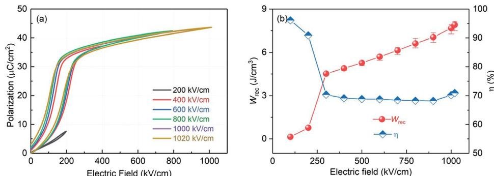
Fig. 15 Energy storage of ANT + Mn multilayer capacitors. (a) Unipolar  $P$ - $E$  loops and (b)  $W_{\text{rec}}$  and  $\eta$  measured at different electric fields from 200 kV  $\text{cm}^{-1}$  to 1020 kV  $\text{cm}^{-1}$ .<sup>81</sup> Reproduced from ref. 81 with permission from the Royal Society of Chemistry.
