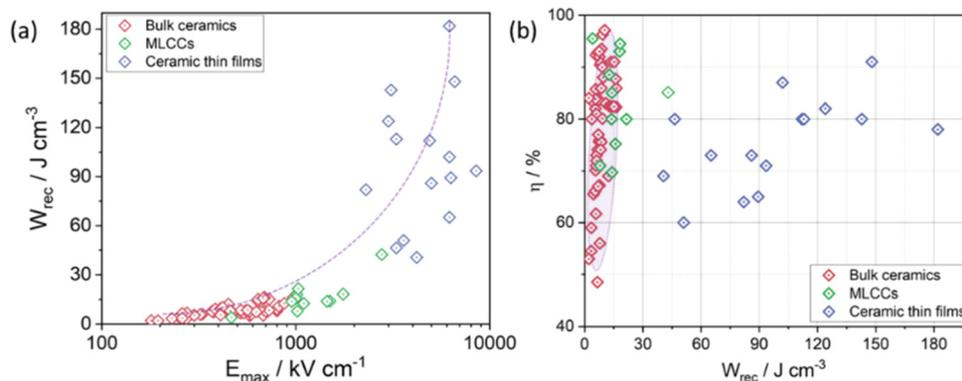
Fig. 18 The comparison between (a)  $E_{\max}$  and  $W_{\text{rec}}$  and (b)  $W_{\text{rec}}$  and  $\eta$  in terms of thickness.
