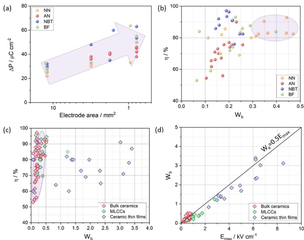
Fig. 20 The relationship between (a) electrode area and  $\Delta P$  in NN, AN, NBT, and BF-based ceramics (b) normalised  $W_{\text{b}}$  and  $\eta$  in NN, AN, NBT, and BF-based ceramics (c) normalised  $W_{\text{b}}$  and  $\eta$  in bulk ceramics, MLCCs, and thin films (d) normalised  $W_{\text{b}}$  and  $E_{\text{max}}$  in bulk ceramics, MLCCs, and thin films.
