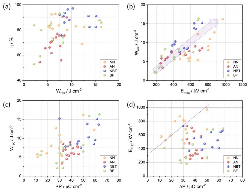
Fig. 17 Comparison between (a)  $W_{\text{rec}}$  vs.  $\eta$  (b)  $W_{\text{rec}}$  vs.  $E_{\text{max}}$  (c)  $W_{\text{rec}}$  and  $\Delta P$  (d)  $E_{\text{max}}$  vs.  $\Delta P$  in different bulk ceramics.
