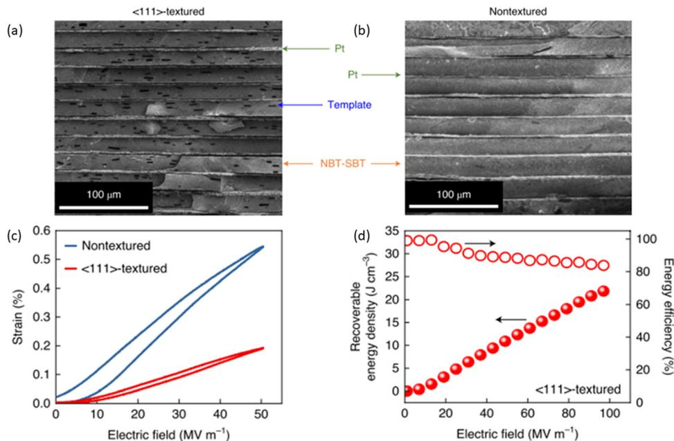
Fig. 24 SEM cross-section of (a) textured and (b) untextured NBT-SBT MLCCs. (c)  $S-E$  Loops of textured and nontextured MLCCs. (d) The energy storage performance of textured NBT-SBT MLCCs.<sup>205</sup> Reproduced from ref. 205 with permission from Springer Nature.
