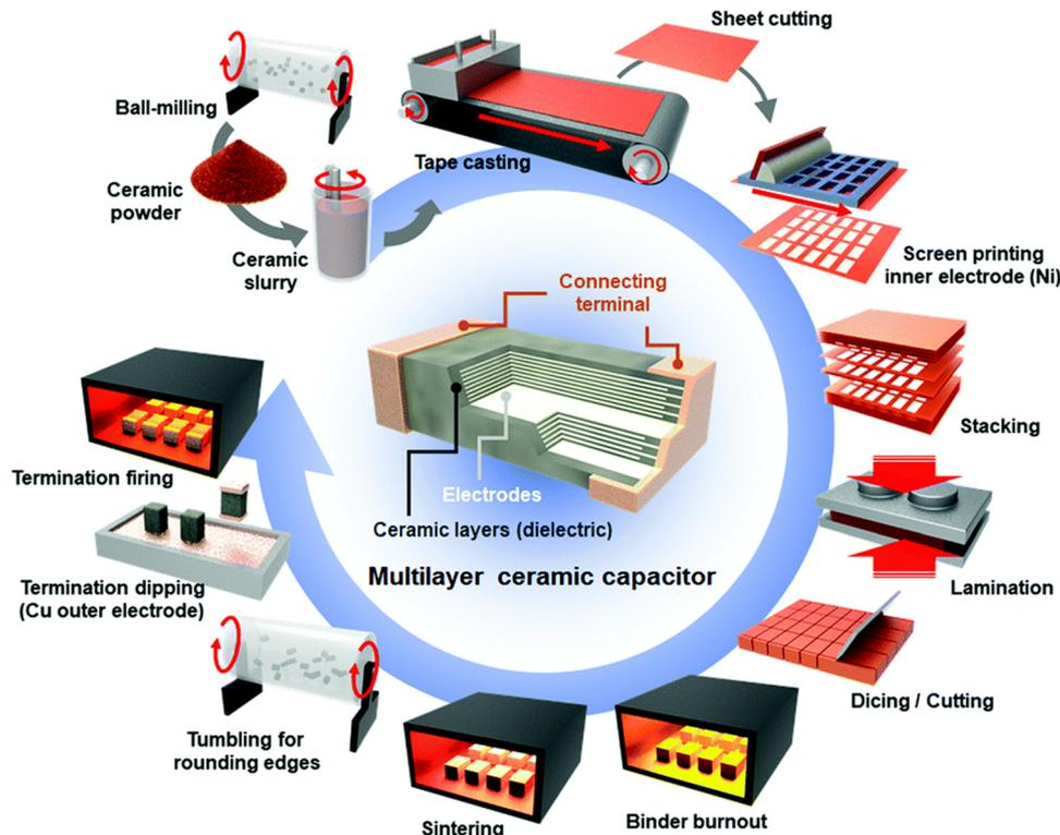
Fig. 12 Schematics of the fabrication process with its construction.<sup>194</sup> Reproduced from ref. 194 with permission from the Royal Society of Chemistry.
