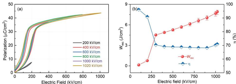
Fig. 15 Energy storage of ANT + Mn multilayer capacitors. (a) Unipolar  $P$ - $E$  loops and (b)  $W_{\text{rec}}$  and  $\eta$  measured at different electric fields from 200  $\text{kV cm}^{-1}$  to 1020  $\text{kV cm}^{-1}$ .<sup>81</sup> Reproduced from ref. 81 with permission from the Royal Society of Chemistry.
