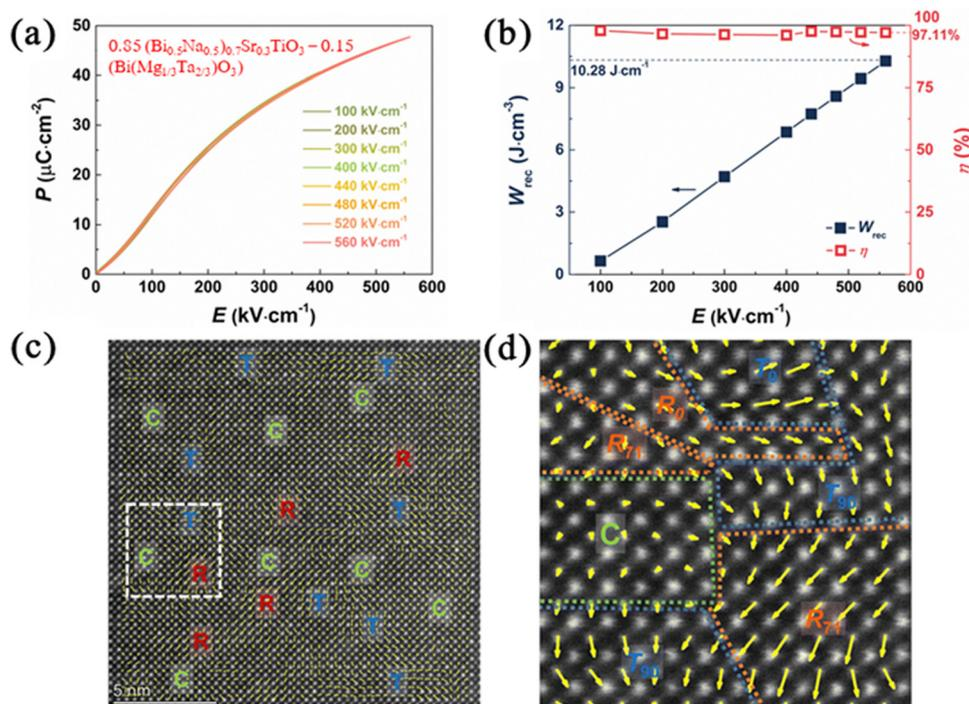
Fig. 9 Properties of 0.85  $(\text{Bi}_{0.5}\text{Na}_{0.5})_{0.7}\text{Sr}_{0.3}\text{TiO}_3-0.15 (\text{Bi}(\text{Mg}_{1/3}\text{Ta}_{2/3})\text{O}_3)$  ceramics (a)  $P$ - $E$  Loops (b)  $W_{\text{rec}}$  and  $\eta$  values (c) HRDP STEM polarisation vector image along  $[100]_c$  (d) enlarged image from the white frame.<sup>160</sup> Reproduced from ref. 160 with permission from the Royal Society of Chemistry.
