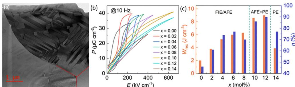
Fig. 8 (a) Overview of bright-field TEM image displaying three grains of the Ag<sub>0.64</sub>Bi<sub>0.12</sub>NbO<sub>3</sub> + 0.10 wt% MnO<sub>2</sub> ceramic (b) unipolar  $P$ - $E$  loops measured at 10 Hz, and (c)  $W_{\text{rec}}$  and  $\eta$  of AN- $x$ Bi ceramics at room temperature.<sup>77</sup> Reproduced from ref. 77 with permission from the Royal Society of Chemistry.
