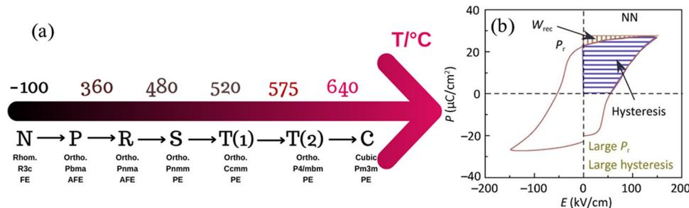
Fig. 6 (a) Phase transition of NN ceramics as a function of temperature (b) PE Loop of NN.<sup>33</sup> Reprinted (adapted) with permission from ref. 33 under the terms of the Creative Commons CC BY license, Elsevier.
