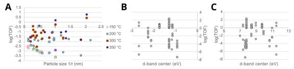
Fig. 26 Turnover frequencies (TOF) of different supported catalysts in the CO<sub>2</sub> hydrogenation reaction as a function of (A) reaction temperature and particle size (1/r), (B) plotted against the d-band center of the metal, and (C) plotted against the adjusted d-band center of the metal as a function of the difference between the metal work function and the conduction band minimum of the MO. (B) and (C) are normalized to the maximum value observed per T.
