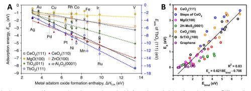
Fig. 10 (A) Correlation between metal/support adsorption energies and oxide formation enthalpies of metal adatoms. Different lines show the trends for different MO supports. Adapted with permission from ref. 92. Copyright 2018, Springer Nature. (B) Metal/support interaction determined from the plot of the activation barrier for diffusion ( $E_a$ ) of metal adatoms against the binding energy ( $E_{bind}$ ) of single metal atoms. From ref. 95. Copyright 2020, Springer Nature
