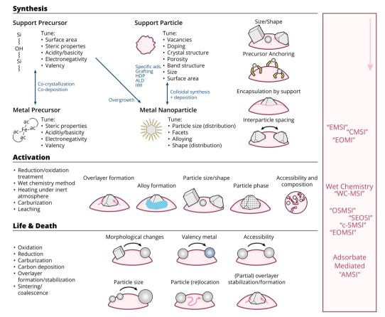
Fig. 17 Schematic overview of the means through which MSI can be tuned, as well as the resulting physicochemical properties affected by these means throughout the lifetime of a catalyst (i.e., during synthesis, activation, reaction, deactivation). The right side of the figure shows typically used abbreviations in literature, and the point in the lifetime of a catalyst when they are at play.
