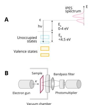
Fig. 23 (A) Energy level diagram of inverse photoemission spectroscopy. Typical energy values for the measurement in the near ultraviolet region are also indicated. (B) Schematic diagram of the experimental setup which implements the concept displayed in panel A. Adapted with permission from ref. 235. Copyright 2012, Elsevier
