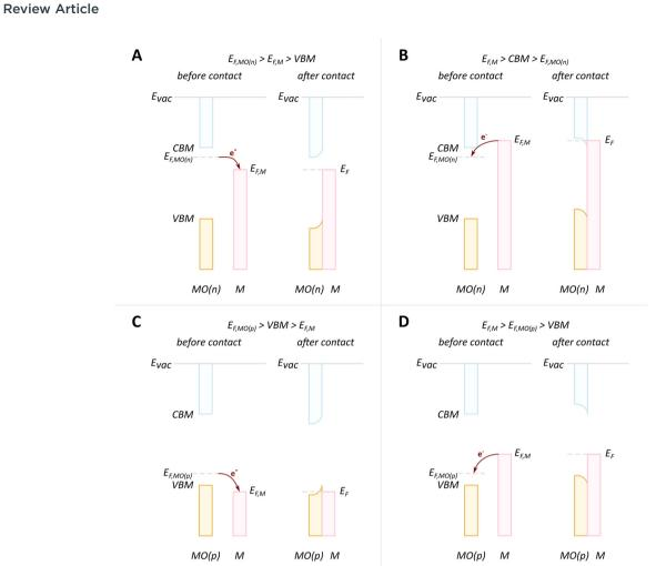
Fig. 7 Schematic diagrams of charge redistribution and band bending for different cases of doping types and Fermi level positions. (A) n-type donordoped MO with Fermi level of MO higher than that of metal; (B) n-type donor-doped MO with Fermi level of MO lower than that of metal; (C) p-doped MO with Fermi level of MO higher than that of metal; (D) p-doped MO with Fermi level of MO lower than that of metal. Adapted with permission from ref. 84. Copyright 2015, Springer Nature.
