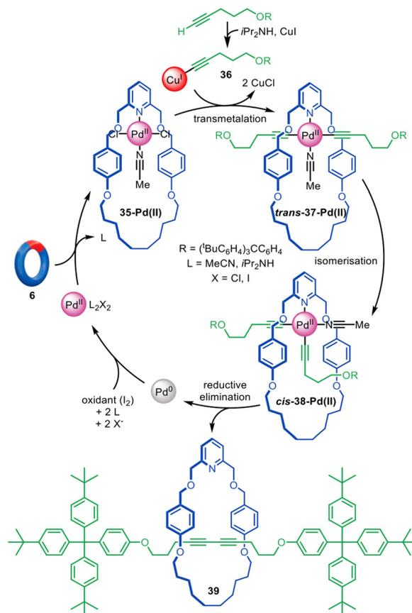
Fig. 11 Active template synthesis of [2]rotaxanes through the Pd(II)-mediated oxidative homocoupling of terminal alkynes.<sup>84</sup>
