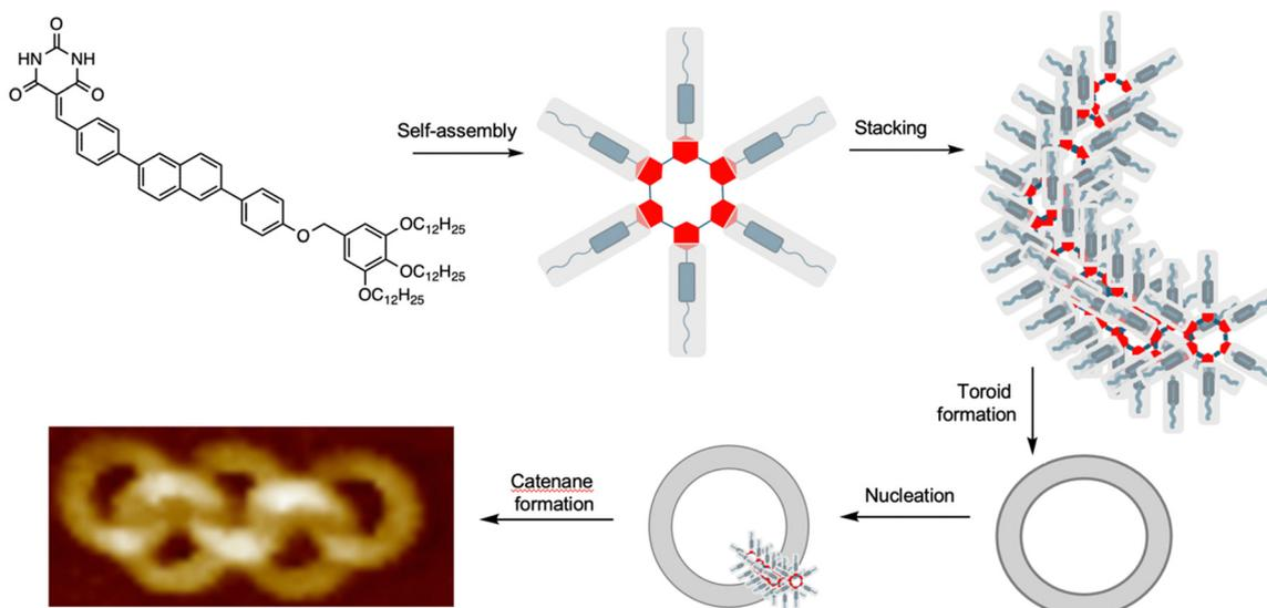
Fig. 29 Yagai's self-assembling polycatenanes consisting of  $\sim 13$  nm diameter supramolecular rings.<sup>140</sup> The molecules with a polar head group, rigid segment and non-polar tail assemble into rosettes that stack to form helical strands and toroids. The internal surface of the toroids seed the formation of new stacks, leading to supramolecular polycatenanes.<sup>140</sup>
