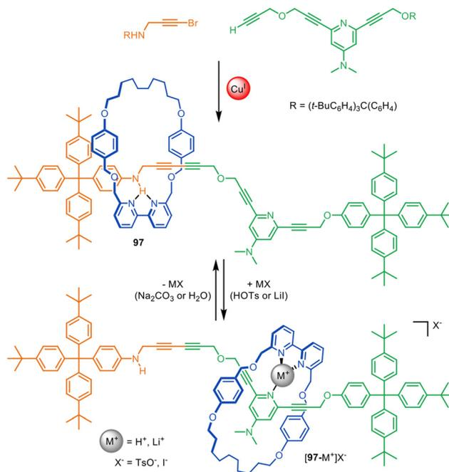
Fig. 30 Active template Cadiot–Chodkiewicz synthesis of molecular shuttle **97**. The position of the macrocycle on the axle is governed by relatively weak intercomponent interactions.<sup>67</sup>
