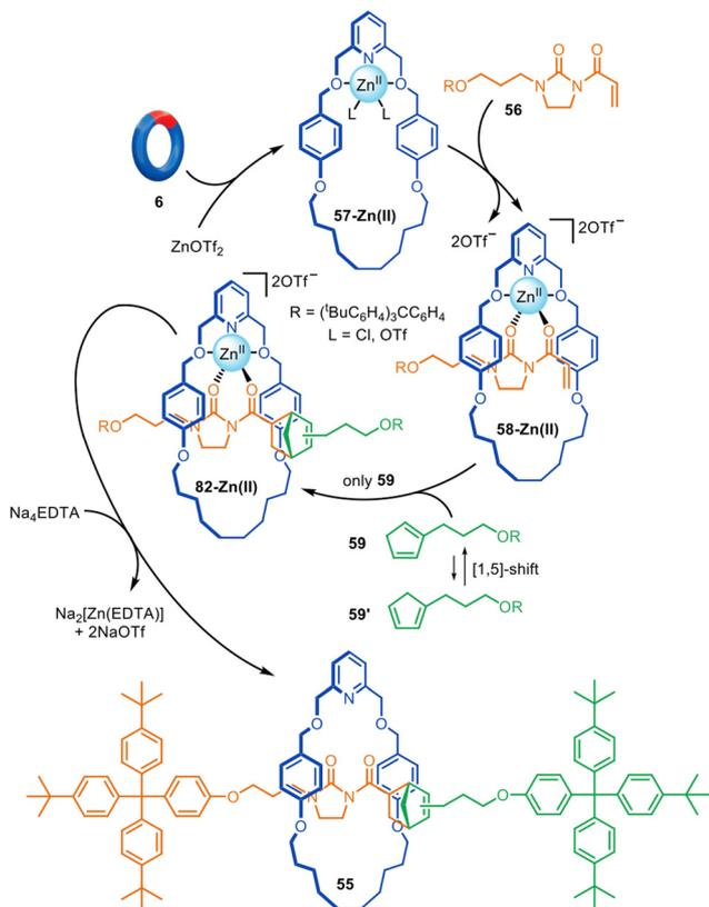
Fig. 18 Active template synthesis of [2]rotaxanes through the Zn(II)-mediated Diels–Alder of imidazolones and cyclopentadiene derivatives.<sup>110</sup>
