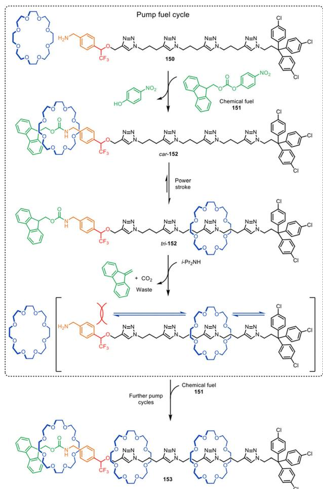
Fig. 48 An autonomous catalysis-driven artificial molecular pump **150** which operates continuously in the presence of chemical fuel **151**.<sup>223</sup>
