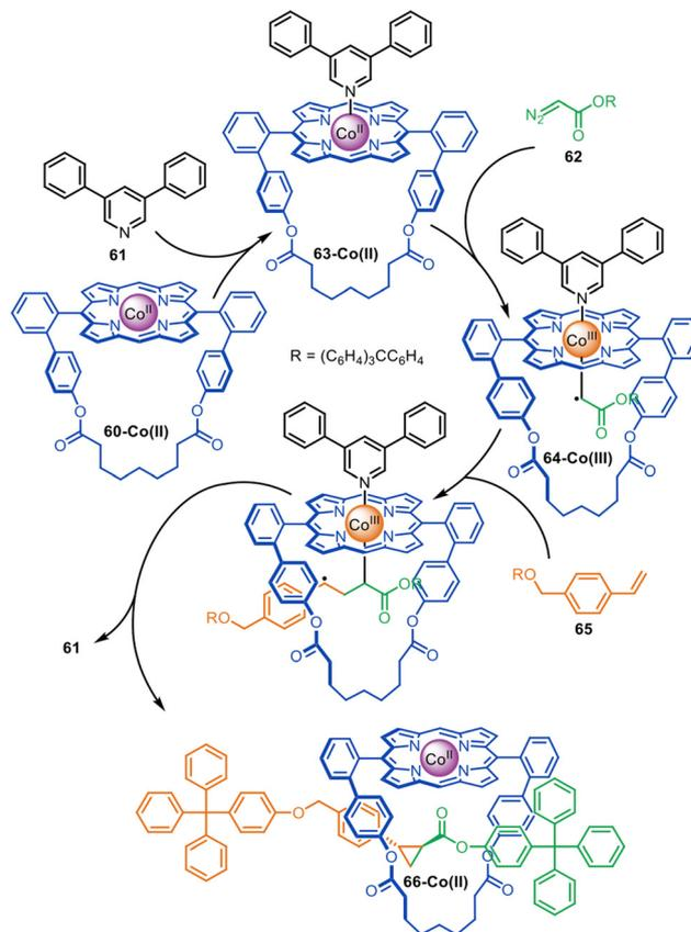
Fig. 19 Megiatto’s active template synthesis of [2]rotaxanes through the Co(II)-mediated radical carbene transfer between diazo and styrene derivatives.<sup>114</sup>
