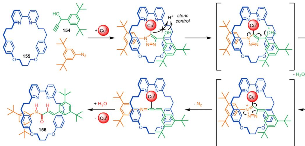
Fig. 49 Proposed mechanism of the tandem active template CuAAC rearrangement reported by Goldup and co-workers.<sup>225</sup>
