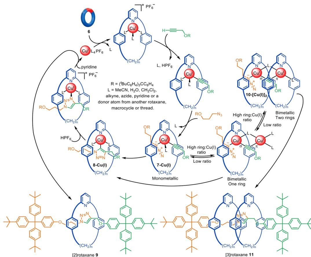
Fig. 4 Mechanism of the active template CuAAC reaction leading to [2]- or [3]rotaxanes depending on the ratio of macrocycle to Cu(I).<sup>28</sup>
