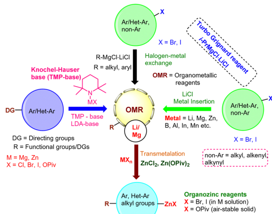
Fig. 1 Reported methods for the preparation of organometallic reagents (RMX).
